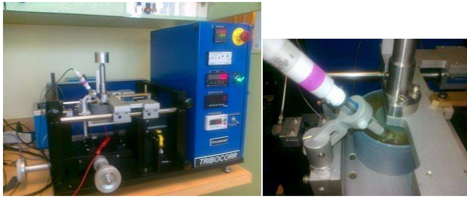
Figure II.21. Machine de Tribocorrosion-Ecole Polytechnique de Montréal LARFIS.
