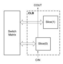
Figure B.11: High-level block diagram of a CLB in Spartan FPGAs [173]
