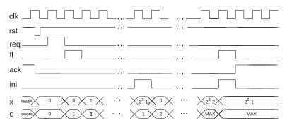
Figure 2.3: Timing diagram of communication signals in the tool  $(MAX = 2^N - 2^{N-k_{max}})$
