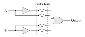
Figure B.2: Programmable circuit with intact fusible links
