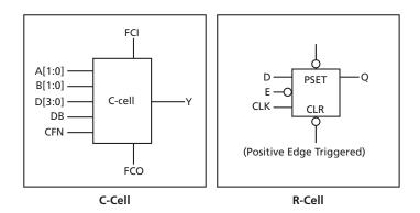
Figure B.12: AX C-Cell and R-Cell [178]
