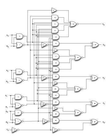
Figure 4.2: 74283 gate-level schematic
