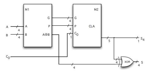
Figure 4.1: 4-bit fast adder circuit
