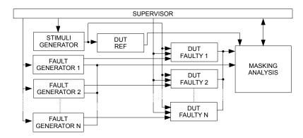
Figure 2.7: The proposed parallel architecture for FIFA
