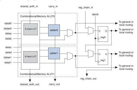
Figure B.8: ALM High-Level Block Diagram [166]
