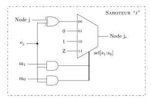
Figure 2.2: General scheme of a saboteur
