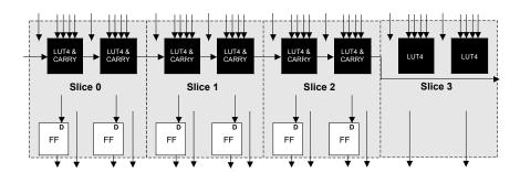
Figure B.14: PFU block diagram [180]
