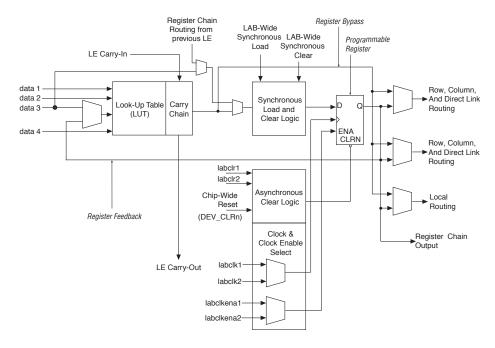
Figure B.9: LE Block Diagram [168]
