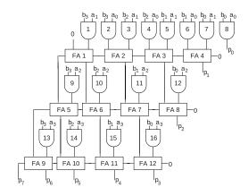
Figure 3.8: Structure of a 4-bit multiplier block
