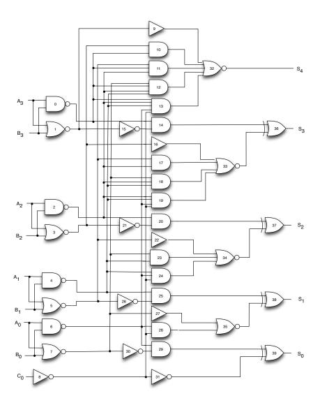
Figure 5.11: Circuit 74283 - Gate level
