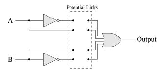
Figure B.1: Programmable circuit concept
