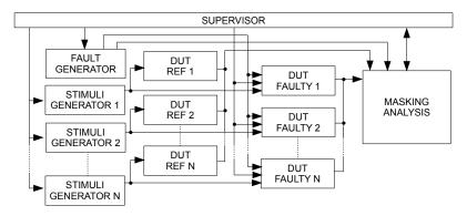
Figure 2.6: A simple parallel architecture for FIFA
