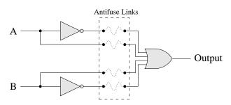
Figure B.4: Programmable circuit with intact antifuses
