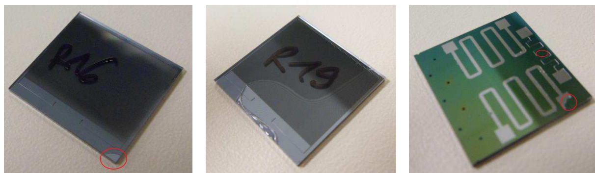
Fig. 57b: illustrations of fabrication issues encountered: benign irregularity (left) and serious defect (middle) of Pyrex bonding, and platinum filaments partial tearing (right).
