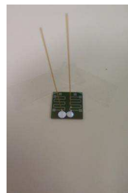
Fig. 55d: bench (top) and zoom on one chip (bottom) before gluing (left), after gluing one capillary on each chip (middle), and after gluing two capillaries on each chip (right)
