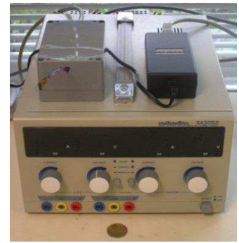
Fig. 60c: power supplies (OA, fans, heater + Peltier)
