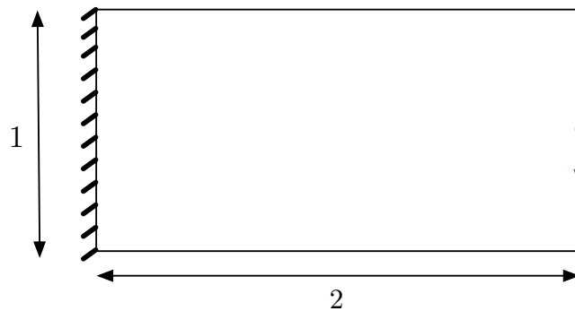
Figure 2.13: Boundary conditions for the 2 \times 1 cantilever.
