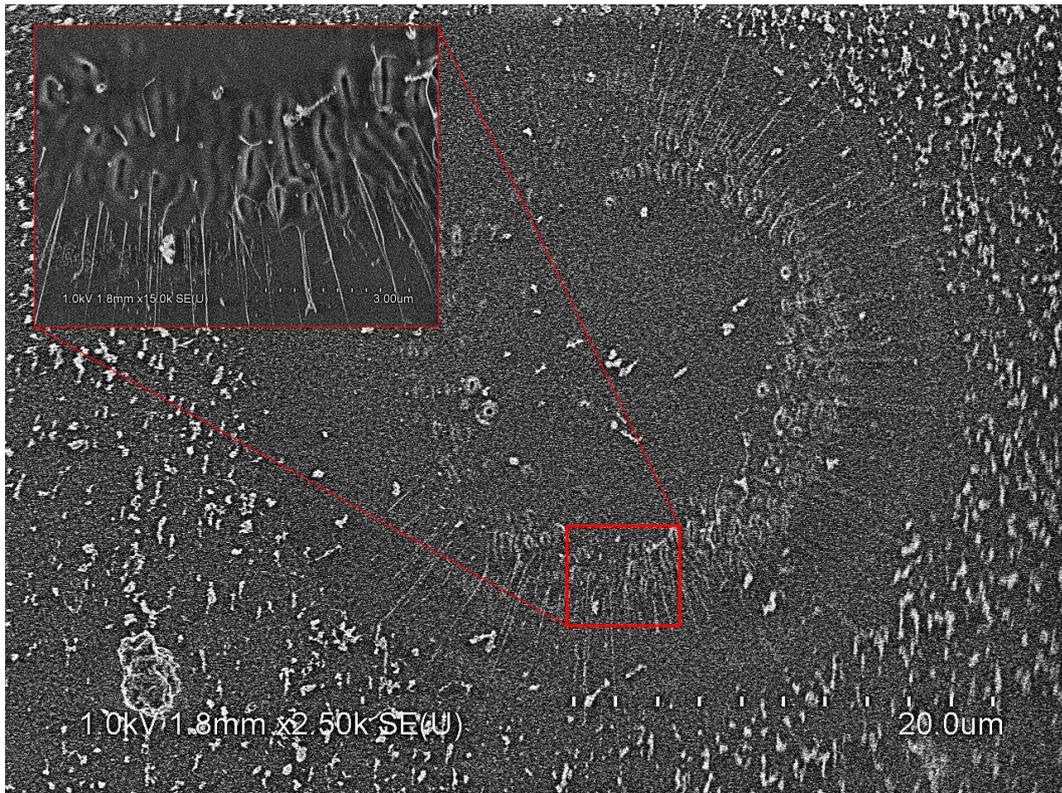
Figure 4.1: SEM image of SiO<sub>2</sub> irradiated with a single IR pulse. Pulse duration is  $\tau=60$  fs and fluence at  $F = 1.2$  J/cm<sup>2</sup> (corresponding to 150% of the SDTH).
