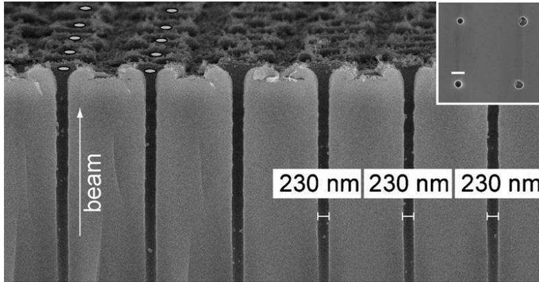
Figure 2: Profile of an array of channels drilled with identical  $0.70 \mu\text{J}$  energy per pulse and beam position such that channel length is  $10 \mu\text{m}$  and diameter  $230 \text{ nm}$ . The pitch is  $1.6 \mu\text{m}$ . White circles indicate channel positions. Inset shows post-processed surface for an additional sample closer to threshold with pitch  $800 \text{ nm}$ . Scale bar is  $200 \text{ nm}$ . Figure from [8].
