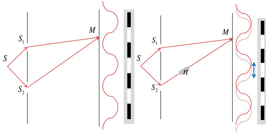
Figure 2.2: Young's double slit experiment, on the right part an object of homogeneous refractive index  $n$  has been added in the path of one ray,  $a$  is the separation between the slits,  $D$  the distance between the slits plane and the observation plane,  $S$  is the light source,  $S_1, S_2$  are the two slits,  $M$  is a point on the observation plane and  $x$  is the shift of the fringe pattern due to the phase object
