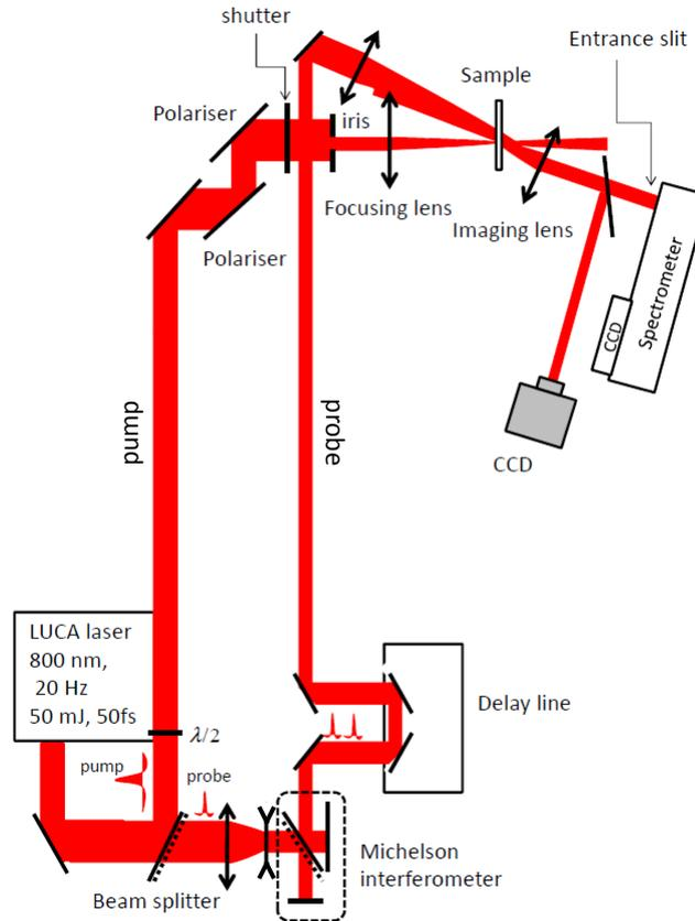
Figure 2.8: The experimental setup in its simplest version.
