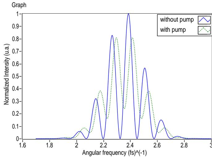
Figure 2.6: The simulated interference is plotted. Blue solid curve correspond to the case where reference and probe pulse go through the same medium. Green, dotted curve correspond to a  $\pi/2$  phase shift, induced by a pump pulse preceding the probe pulse.
