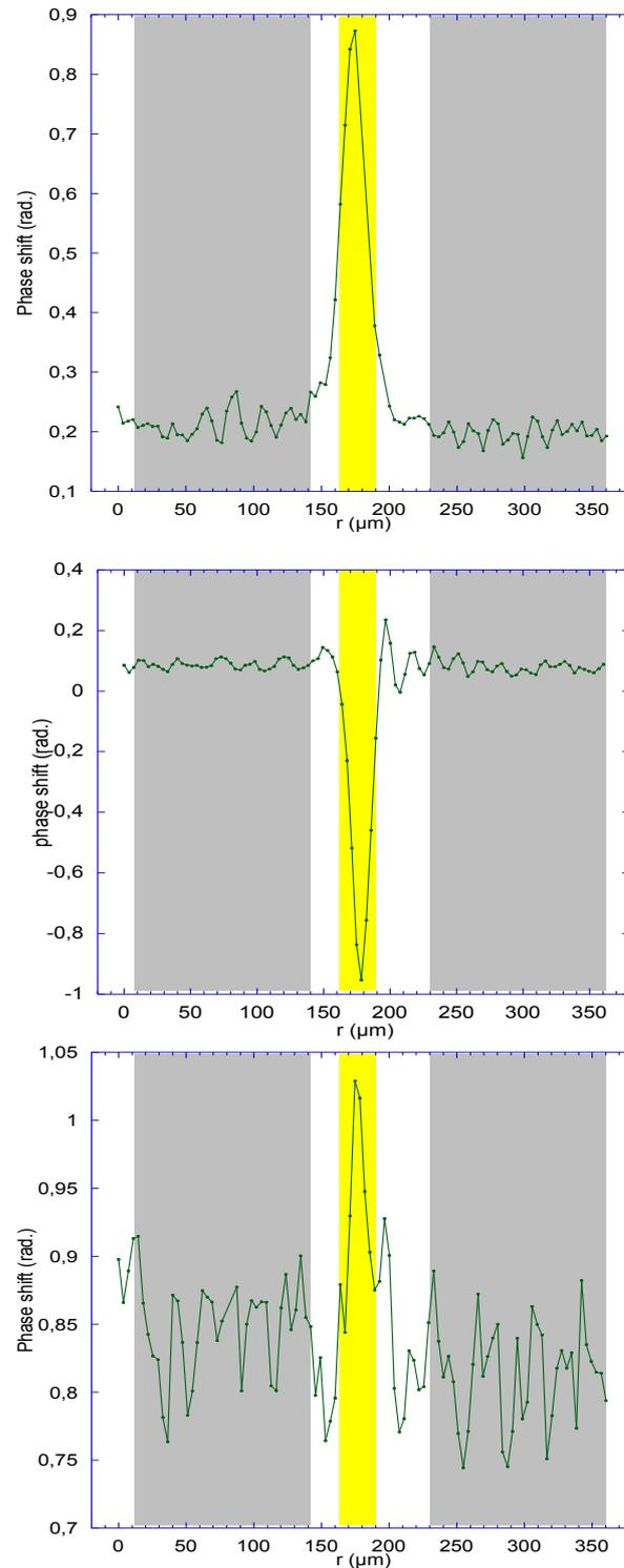
Figure 2.11: Phase shift as a function of the transverse coordinate of the beam  $r$ , for three pump-probe delays. From top to bottom different contributions encountered are : Kerr effect, free carrier generation and trapped carrier formation respectively (see section 2.4.1 for more details) The three different regions to be integrated are illustrated, with light grey being the integration over the ground level and yellow the actual measured signal.
