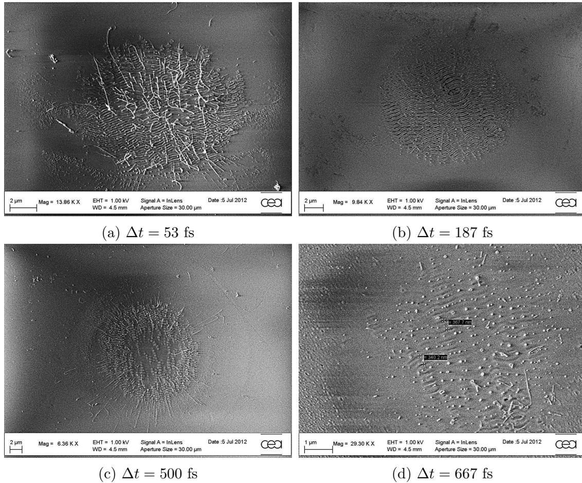
Figure 4.13: SEM images of  $\text{SiO}_2$  irradiated with 3 double-pulse (UV and IR) sequences of varying delays [ $\Delta t = -667$  fs to 1.3 ps] at corresponding fluencies of  $1.9 \text{ J/cm}^2$  for UV ( $\tau = 60$  fs) and  $2 \text{ J/cm}^2$  for IR ( $\tau = 300$  fs). Lower and higher delay for which damaging was observed is represented. Notice the change in scale between the images.
