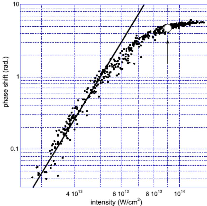
Figure 2.1: Phase shift as a function of laser intensity measured in  $\text{Al}_2\text{O}_3$ . The pump wavelength is 800 nm and the duration is 60 fs. The line is indicating an  $I^6$  dependence law. The arrow and empty circle indicate the breakdown threshold. Figure from [72].
