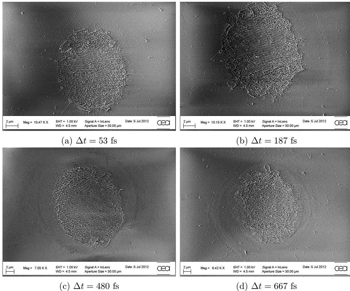
Figure 4.17: SEM images of  $\text{SiO}_2$  irradiated with 10 double-pulse (UV and IR) sequences of varying delays [ $\Delta t = t = -667$  fs to 1.3 ps] at corresponding fluencies of  $1.9 \text{ J/cm}^2$  for UV ( $\tau = 60$  fs) and  $2 \text{ J/cm}^2$  for IR ( $\tau = 300$  fs). Lower and higher delay for which damaging was observed is represented. Notice the change in scale between the images.
