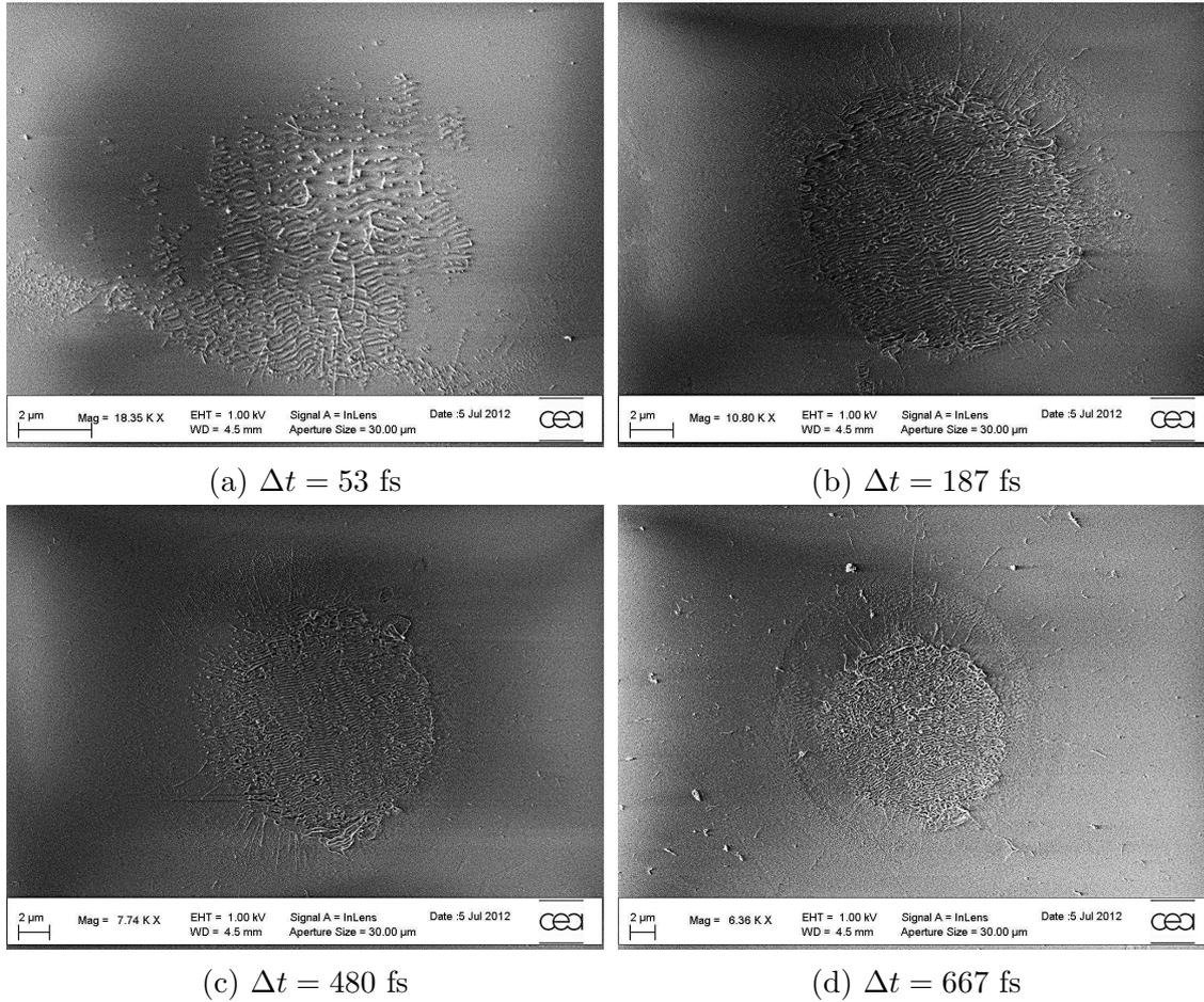
Figure 4.15: SEM images of  $\text{SiO}_2$  irradiated with 5 double-pulse (UV and IR) sequences of varying delays [ $\Delta t = -667$ fs to 1.3 ps] at corresponding fluencies of  $1.9 \text{ J/cm}^2$  for UV ( $\tau = 60$  fs) and  $2 \text{ J/cm}^2$  for IR ( $\tau = 300$  fs). Lower and higher delay for which damaging was observed is represented. Notice the change in scale between the images.
