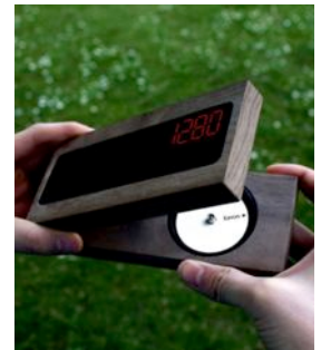
Figure 17 GPS on an ordinary phone (Top); Compass Phone by Hayeon Yoo (Bottom). It measures the distance between two people and converts it to the time it takes for them to meet each other. The centre of the compass indicates the user’s position and its needle indicates the other person’s direction (hayeon.yoo.com)
