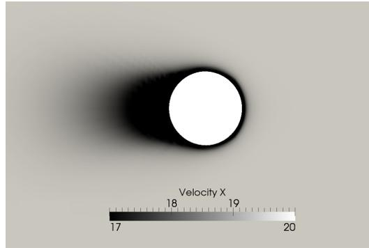
Fig. 9. Velocity in the x-direction (defined in Fig.3), cylinder in near-axial flow with a yaw angle  $\alpha = 5^\circ$ , view in the plane (y,z) at a distance  $x = 0.46$  m from the first end of the cylinder.
