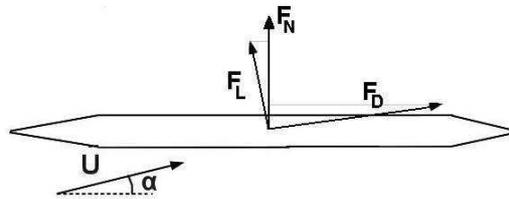
Fig. 1. Cylinder in near axial flow with an angle  $\alpha$ , definition of the normal force  $F_N$ , the lift force  $F_L$  and the drag force  $F_D$ .
