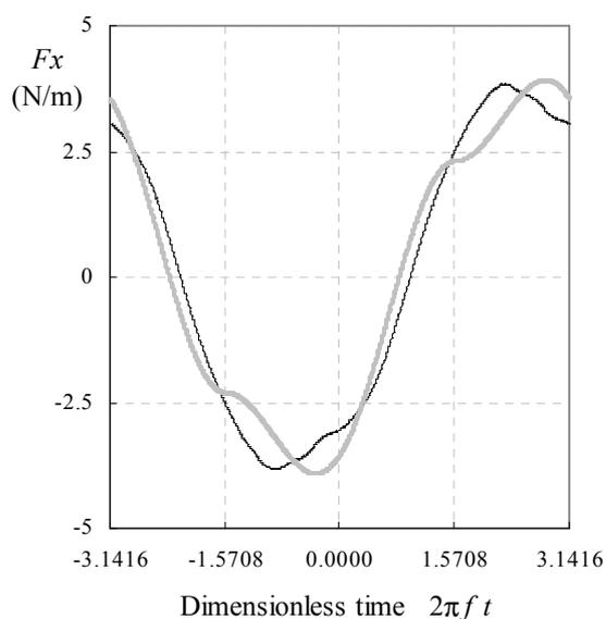
Fig. 6: evolution of the x-component of the force during one cycle of oscillation for the central cylinder for a displacement of the array proportional to  $\sin 2\pi ft$ . Black line: result of the computation of the reference case, gray line: Morison-like fit of the result of the computation (see next Section )
