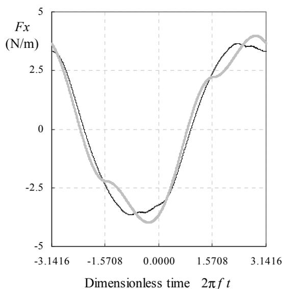
Fig. 5: evolution of the x-component of the force exerted upon the upper center cylinder during one cycle of oscillation, for a displacement of the array proportional to  $\sin 2\pi ft$ . Black line: result of the computation of the reference case, gray line: Morison-like fit of the result of the computation (see next Section )
