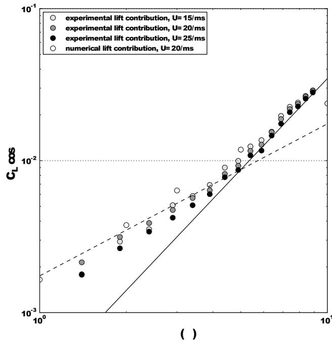
Fig. 6. Experimental and numerical lift contributions to the normal force  $C_L \cos \alpha$ . A transition between the linear and the quadratic regimes is observed.
