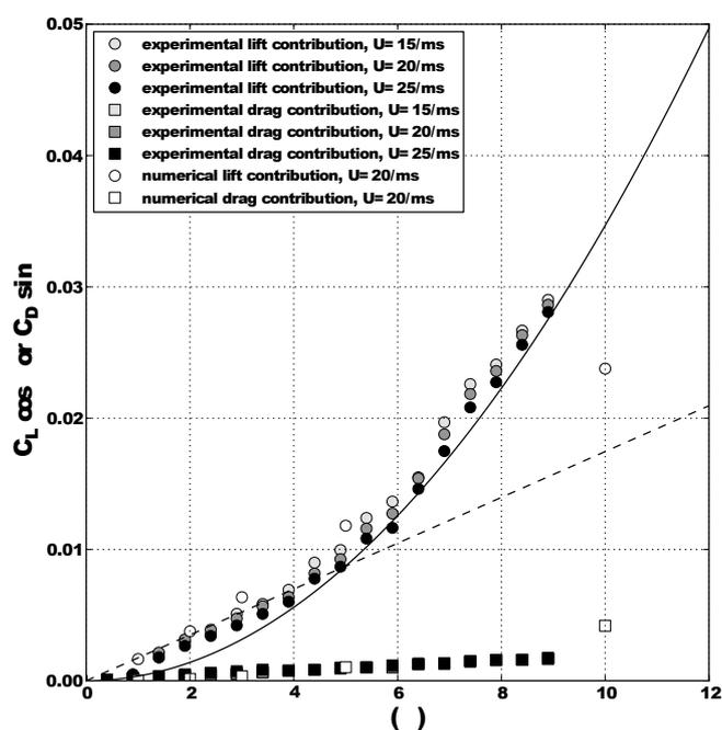
Fig. 5. Lift and drag contributions to the normal force  $C_L \cos \alpha$  et  $C_D \sin \alpha$  such as  $C_N = C_L \cos \alpha + C_D \sin \alpha$ . Comparison between experimental measurements and CFD simulation results. Linear regime for  $\alpha < 5^\circ$  and comparison with the cross flow principle for  $\alpha > 5^\circ$ .
