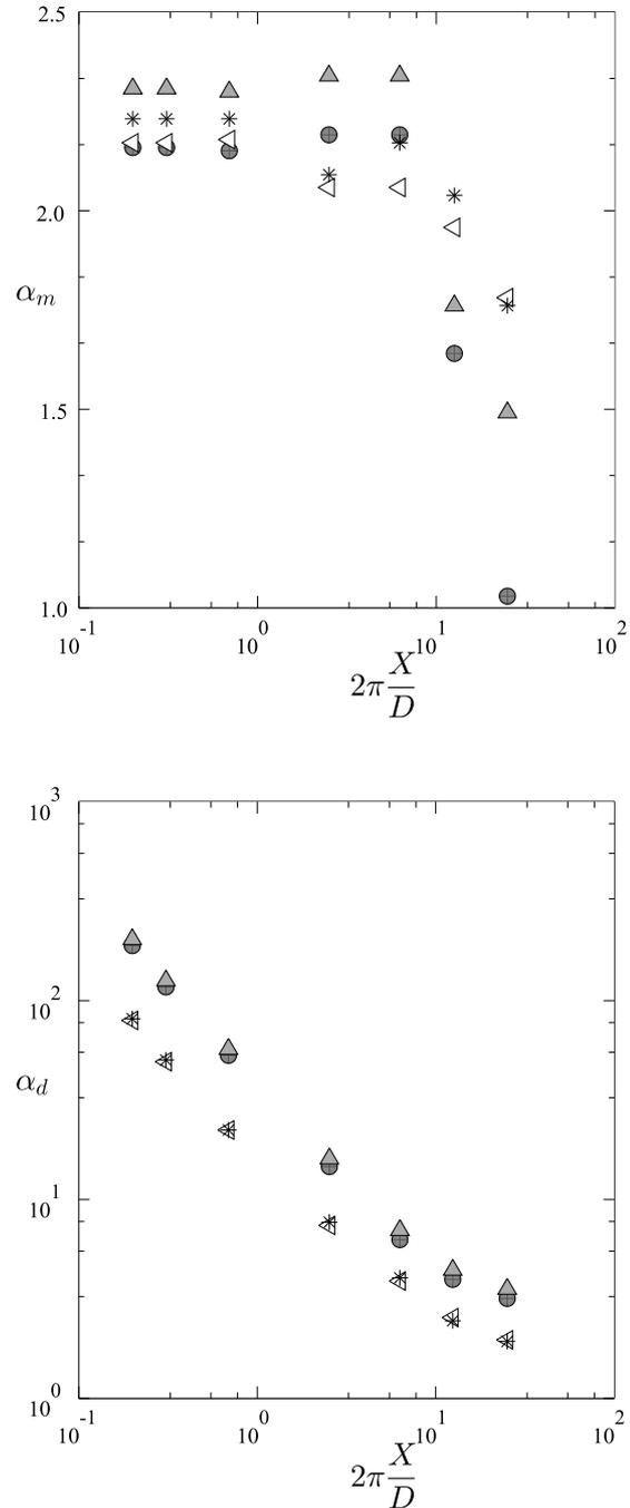
Fig. 8: mass and drag coefficients vs. Keulegan Carpenter number.  $\bullet$ : center cylinder,  $\triangle$ : left central cylinder,  $*$ : central upper cylinder,  $\nabla$ : upper left cylinder
