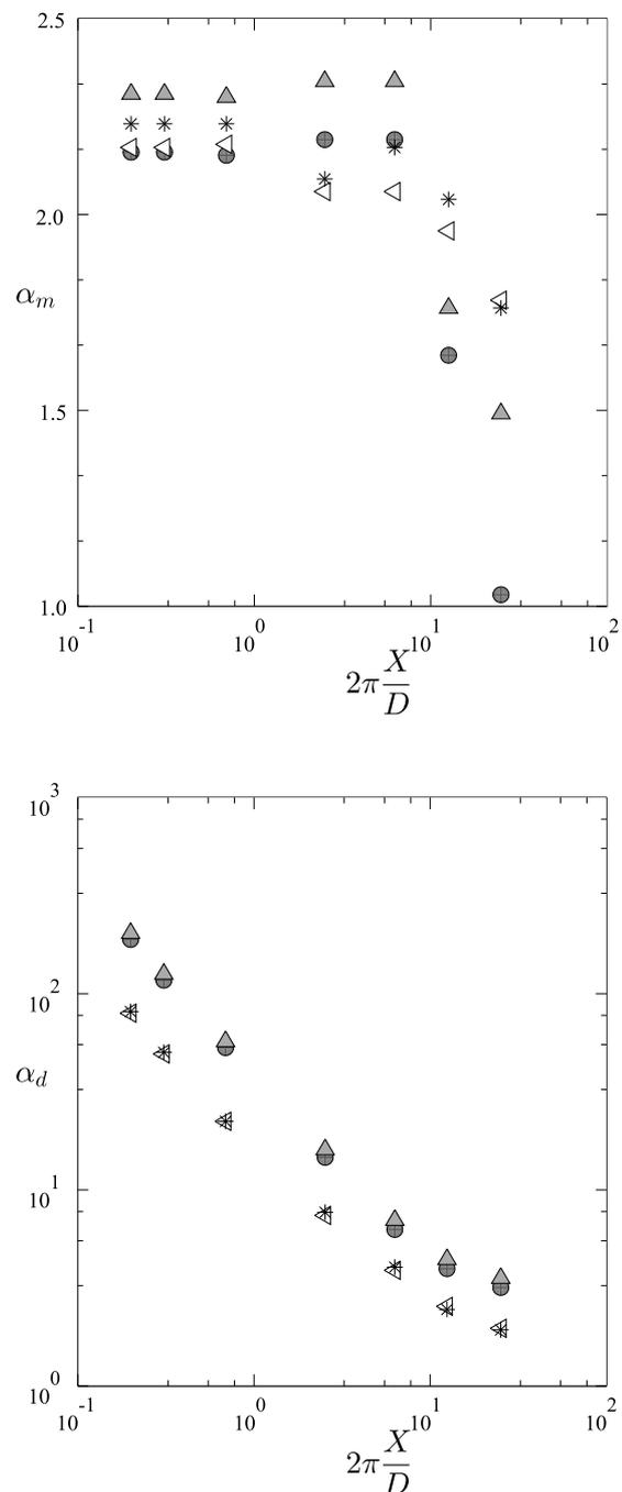
Fig. 8: mass and drag coefficients vs. Keulegan Carpenter number.  $\blacktriangle$ : center cylinder,  $\bullet$ : left central cylinder,  $\triangle$ : central upper cylinder,  $*$ : upper left cylinder
