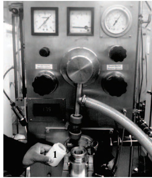
Fig. 3.10. Real representation of experimental setup for the injection of tracer. (Left) 1. Syringe and valve for tracer injection. 2. Inlet thermocouple. 3. SSHE 4. Outlet pipe of SSHE with valve. 5. Derivation pipe with valve (not shown in the picture). (Right) 1. Sampling cup
