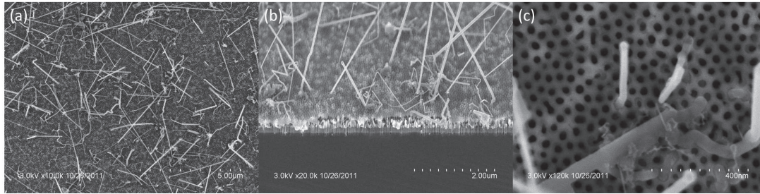
Figure 4.37: SEM pictures of the porous stack after a SiNW growth at 450°C for \text{SiH}_4:\text{H}_2 = 20:100 sccm.
