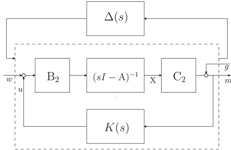
Figure 4.6: Closed-loop perturbed system. The closed-loop system composed by the plant and the compensator is enclosed in the dashed box. Noises  $w$  and  $g$  are the system inputs, while  $m$  is the measurement output. The perturbation  $\Delta(s)$  represents all possible disturbances to the closed-loop system.
