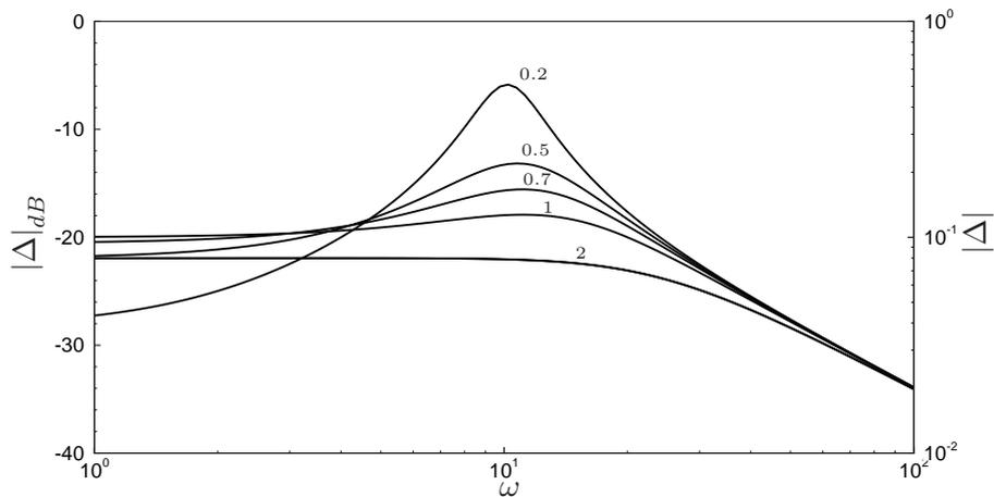
Figure 4.7: Amplitude of the perturbation  $\Delta$  expressed in  $dB$  on the left axis and non-dimensional on the right axis, for a given range of frequencies in  $rad/s$ . Every curve is obtained from Eq. (4.17), with a fixed value of  $\omega_\Delta = 10 rad/s$ . Values close to each curve indicate the damping ratio  $\zeta = -\sigma_\Delta/\omega_\Delta$ .
