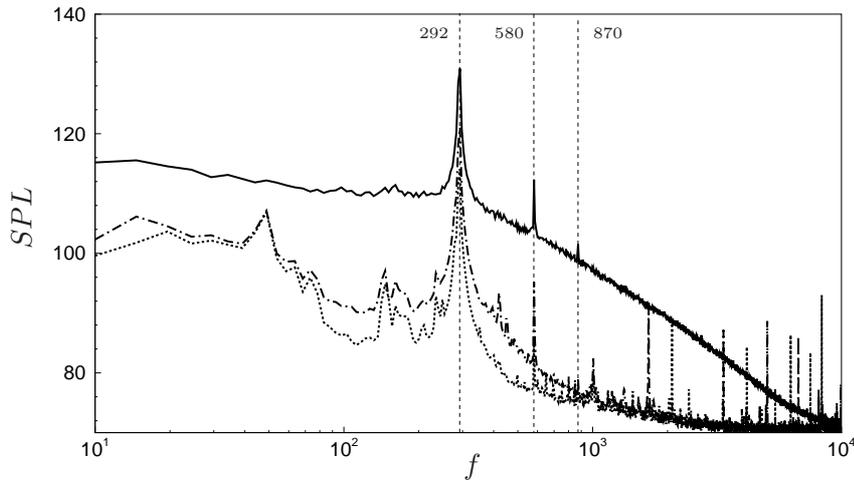
Figure 2.6: SPL, expressed in  $dB$ , of unsteady pressure measurements. Transducers are located on the upstream wall of the cavity (dashed line), on the downstream wall (solid line) and on the bottom (dashed-dotted line).
