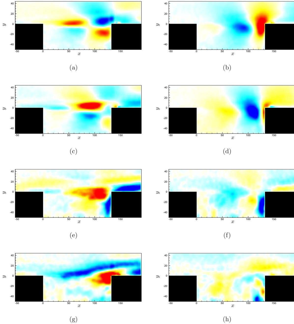
Figure 3.7: First 4 POD modes computed from 500 snapshots acquired at  $3 \text{ kHz}$  with a flow at  $34 \text{ m/s}$  and filtered with a Fourier filter above  $150 \text{ Hz}$ . (a)  $\Phi_1^u$ , (b)  $\Phi_1^v$ , (c)  $\Phi_2^u$ , (d)  $\Phi_2^v$ , (e)  $\Phi_4^u$ , (f)  $\Phi_4^v$ , (g)  $\Phi_5^u$ , (h)  $\Phi_5^v$ . Levels are from  $-0.035$  to  $0.035$ .
