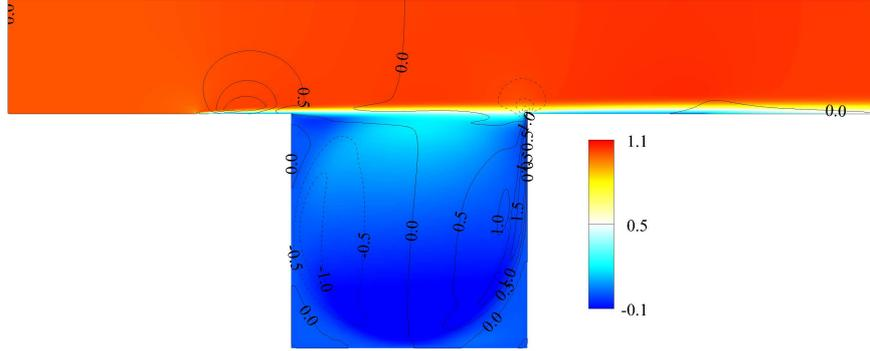
Figure 4.1: The contour plot corresponds to the streamwise component of the base flow,  $u_0$  obtained at  $Re = 7500$ , while the spatial profile of the control input  $u(t)$  is represented by the isolines.
