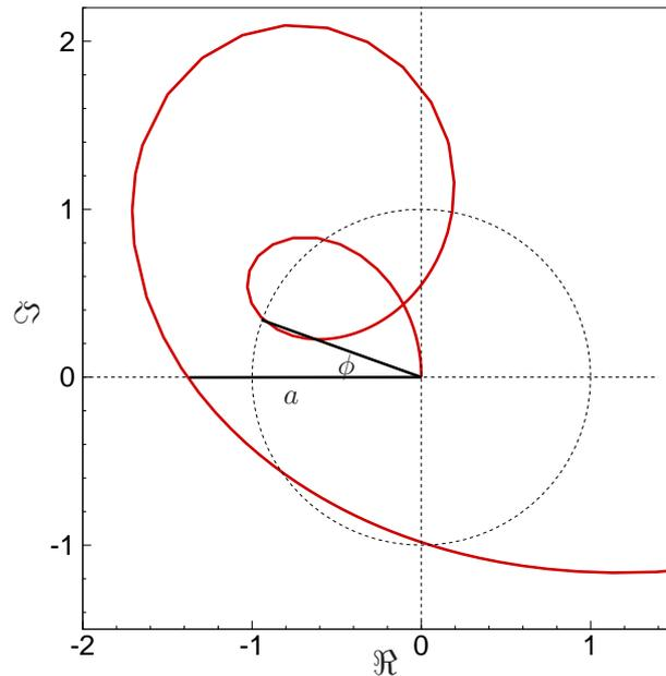
Figure 4.9: Graphical representation of the Nyquist criterion.
