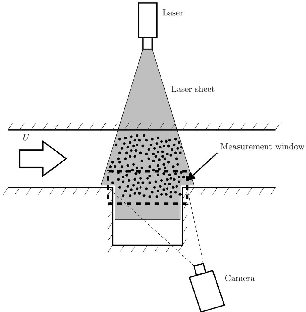
Figure 2.8: Scheme of a 2D-2C PIV acquisition for a cavity flow.
