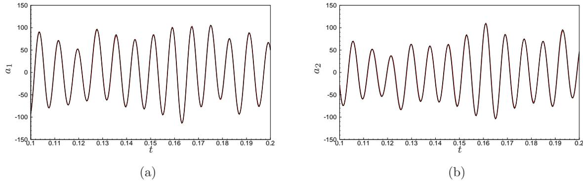
Figure 3.8: Comparison of the time projections corresponding to the first 2 POD modes computed from snapshots acquired at  $3kHz$  at a velocity of  $34\text{ m/s}$  and filtered with a Fourier filter above  $150\text{ Hz}$ . Red lines represent the filtered trajectories obtained from the original velocity fields; black lines represent trajectories from the filtered snapshots.
