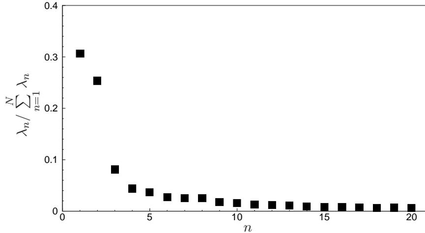
Figure 3.6: Contribution of the first 20 eigenvalues computed from the correlation term corresponding to a set of  $N_s = 500$  snapshot acquired at  $3 \text{ kHz}$  with a flow at  $34 \text{ m/s}$  and filtered with a Fourier filter above  $150 \text{ Hz}$ .
