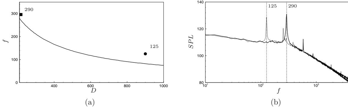
Figure 2.7: (a) East model for frequency (in  $Hz$ ) prediction as a function of the cavity depth,  $D$  (in  $mm$ ). The small square represents the characteristic frequency at the original depth, while the circle stands for the frequency obtained after cavity depth modification. (b) Comparison of SPL (in  $dB$ ) obtained from the same transducer measurement with the original cavity (solid line) and the modified one (dashed line).
