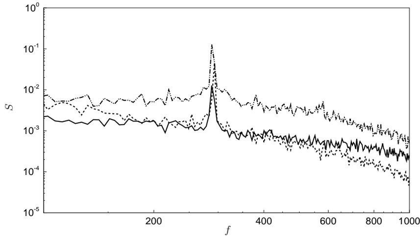
Figure 2.3: Spectra of measured signals (in  $V$ ) at three different locations in the cavity:  $x = 4mm, y = 0mm$  (solid line),  $x = 60.7mm, y = -25mm$  (dashed line) and  $x = 130mm, y = 0mm$  (dashed-dotted line).
