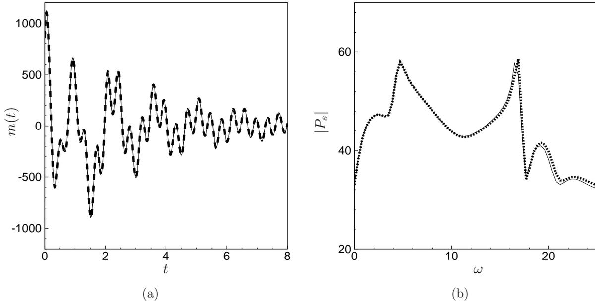
Figure 4.5: Impulse response of the stable system at Reynolds 5500. (a) Time behavior of the measurement  $m(t)$ . (b) Open-loop transfer function amplitude in  $dB$  over a range of frequencies expressed in  $rad/s$ . Thick dashed line corresponds to the DNS; thin solid line corresponds to the reduced model based on BPOD.
