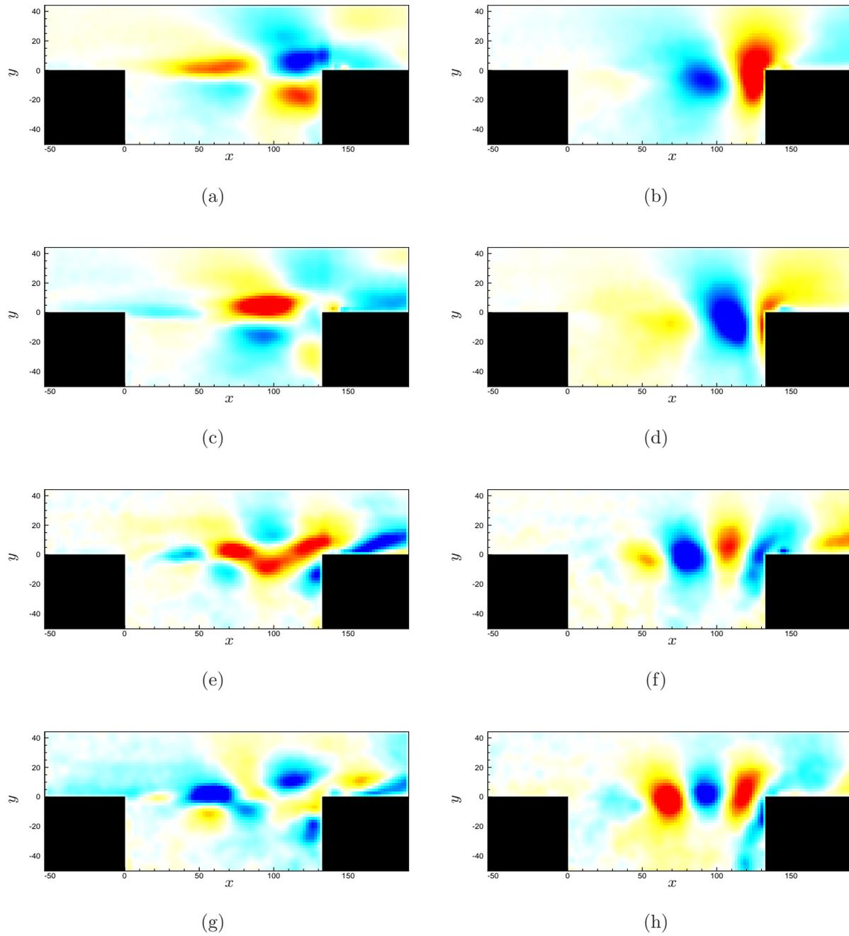
Figure 3.2: POD modes computed from 500 snapshots acquired at 3 kHz with a flow at 34 m/s. (a)  $\Phi_1^u$ , (b)  $\Phi_1^v$ , (c)  $\Phi_2^u$ , (d)  $\Phi_2^v$ , (e)  $\Phi_4^u$ , (f)  $\Phi_4^v$ , (g)  $\Phi_5^u$ , (h)  $\Phi_5^v$ . Levels are from -0.035 to 0.035.
