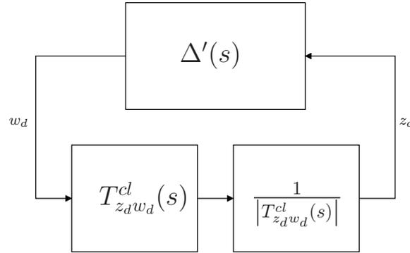
Figure 4.11: Normalized unstructured uncertainty block scheme.
