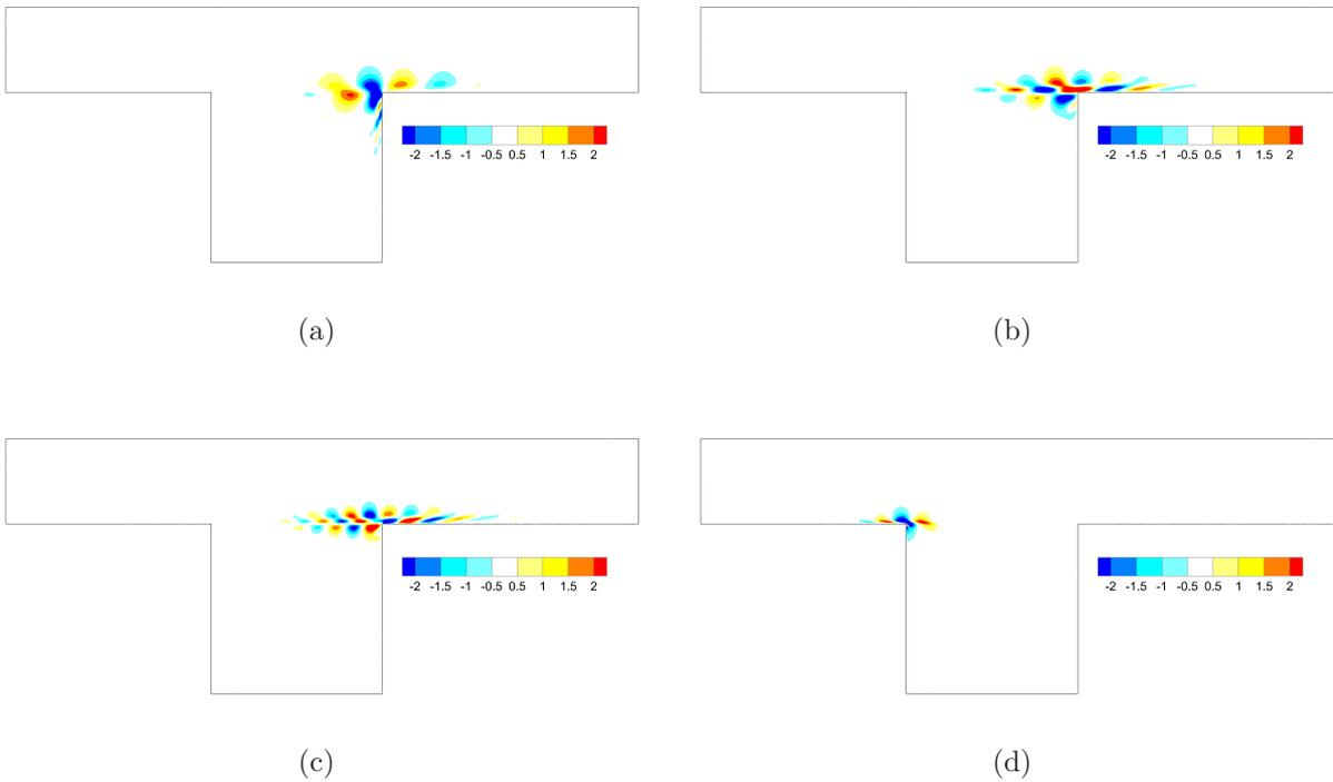
Figure 4.3: (a) cross-stream component of the direct global mode at  $\omega = 7.9$ ; (b) streamwise component of the direct global mode at  $\omega = 10.9$ ; (c) streamwise component of the direct global mode at  $\omega = 16.7$ ; (d) cross-stream component of the adjoint global mode at  $\omega = -13.8$ .
