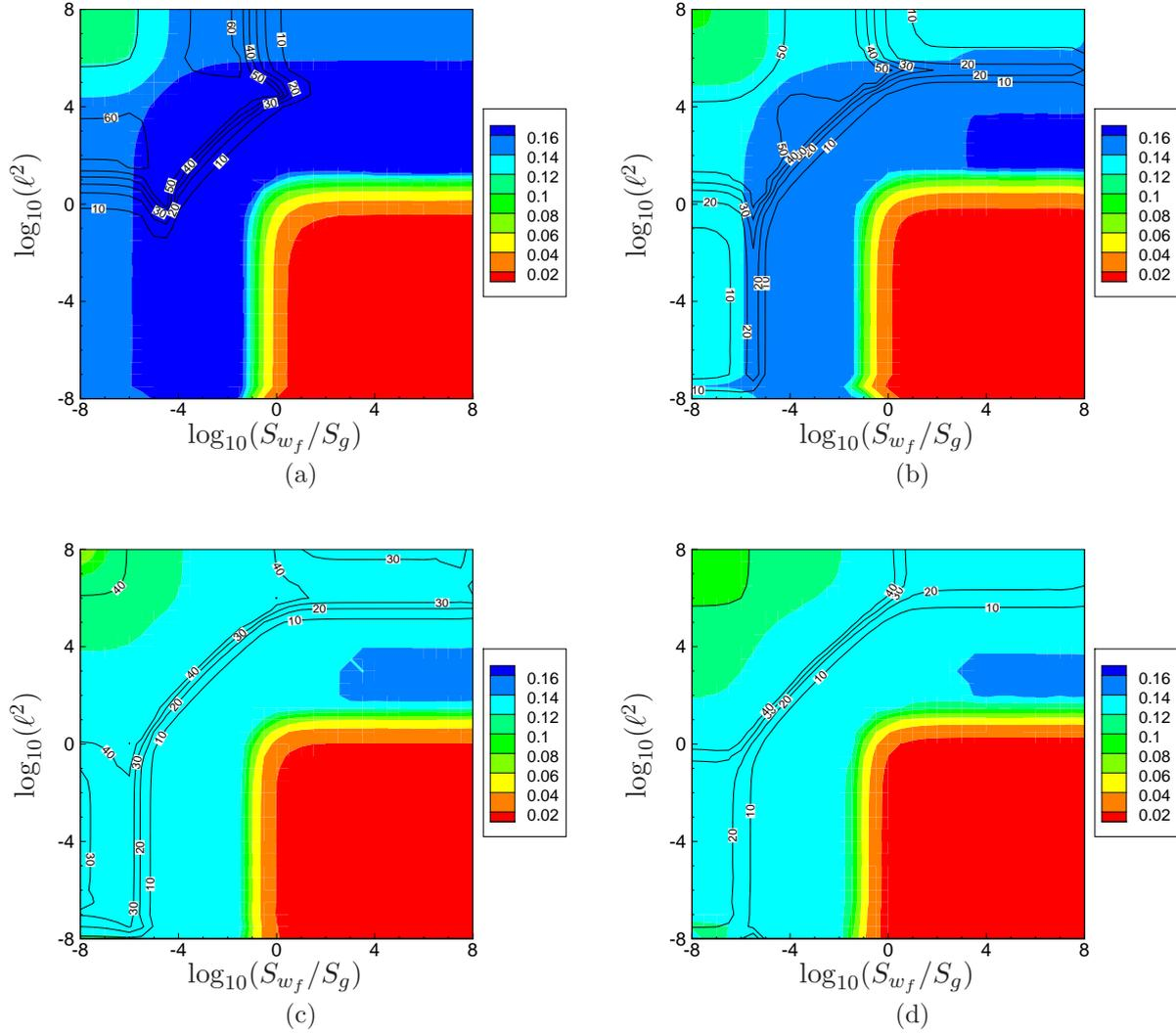
Figure 4.15: Parametric analysis over the four different Reynolds numbers. Contours correspond to the robustness parameter  $\rho_\infty^{im}$ . Iso-lines correspond to  $\rho_\infty^{io}$
