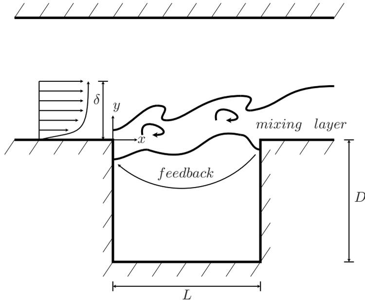
Figure 1.1: Schematic description of the cavity resonance.
