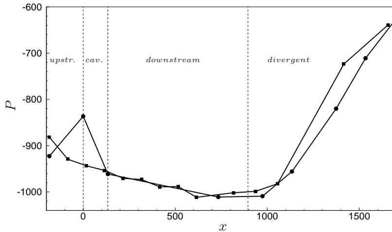
Figure 2.5: Steady pressure measurements along the model section. Pressure values are expressed in  $Pa$ , while the longitudinal direction is in  $mm$ . Top static probes are represented by squares, bottom probes by circles.
