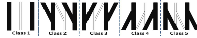
Fig. 11. Shape of 5 classes of turnout to classify in the bird's-eye view image.
