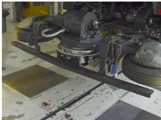
FIGURE 1.2 – La traverse chasse-corps du VAL.
