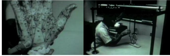
Figure 3. (a) Polygons drawn over a hand mock up for 3D registering of defining dots; (b) Digitalization of the hand with a 3D pointer which records all 3 coordinates.
