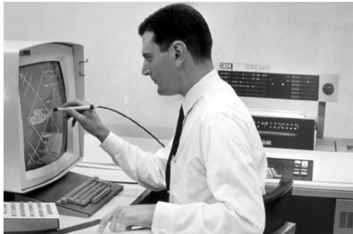
Figure 2. IBM 2250 Display connected to an IBM 1130 Computer
