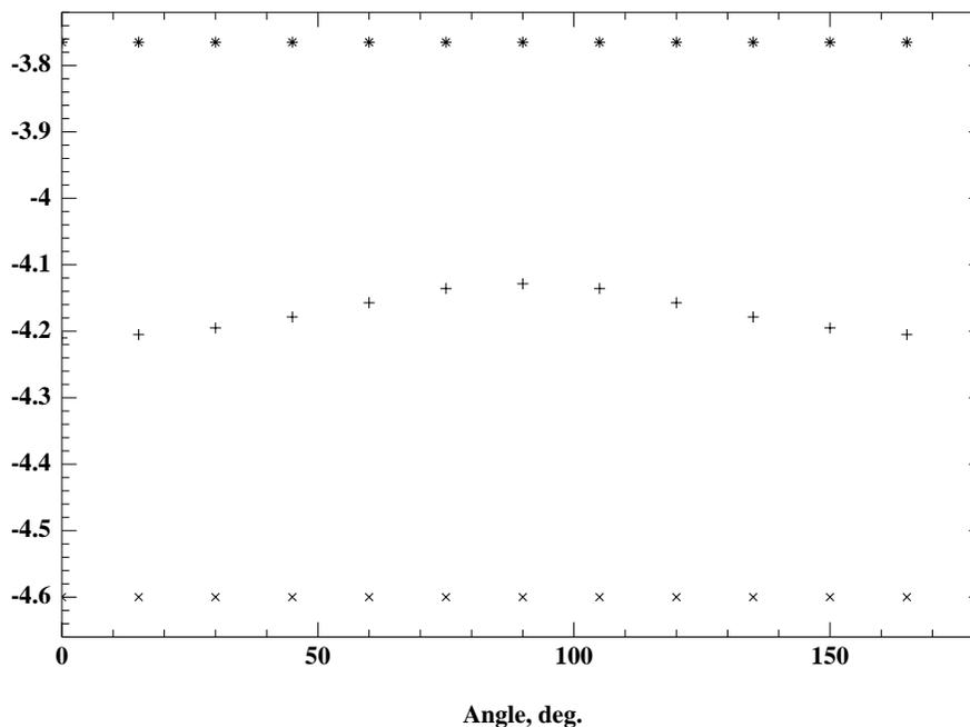
FIG. 2:  $\Delta G_{sol}$  values of HF in 7CB (+) and for two hypothetical isotropic solvents of permittivity equal to 5.54 (\*) and 17.1 (x) respectively, with respect to the angle between the bond axis and the  $z$  axis.
