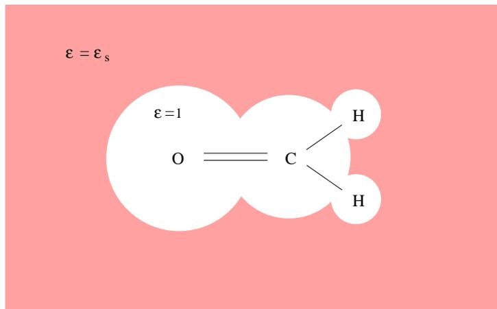
FIG. 1: Solvation Continuum Models: a representation of H<sub>2</sub>CO surrounded by a homogeneous dielectric modelling the solvent.
