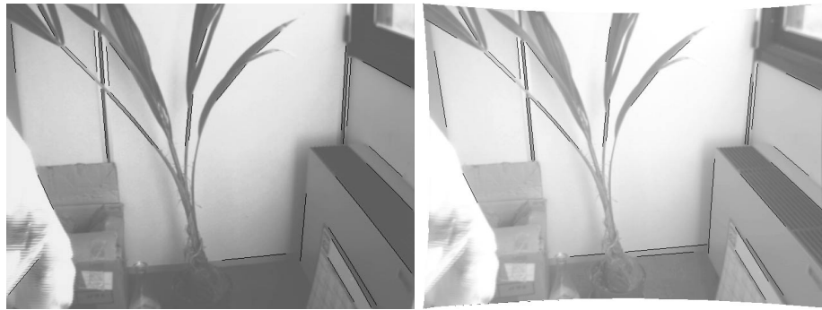
Figure A.2: A distorted image with the detected segments (left) and the same image at the end of the distortion calibration with segments extracted from undistorted edges (right): some outliers were removed and sometimes longer segments are detected.
