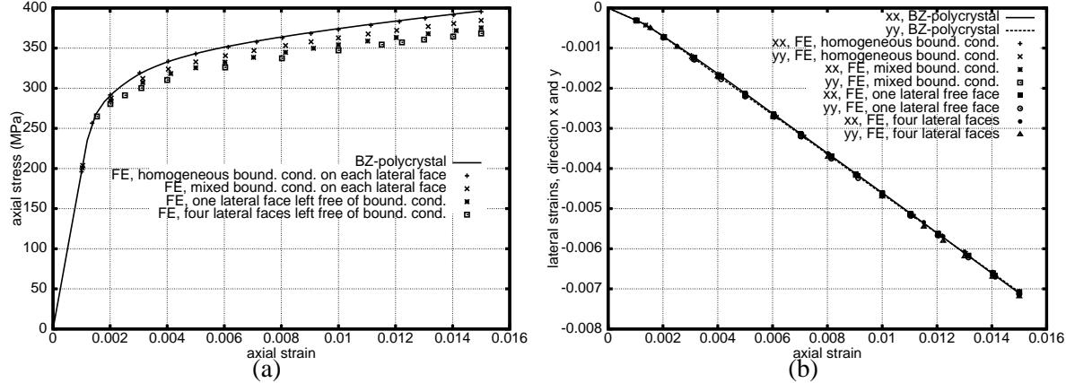
**Figure III.1** : Simulations of tensile tests to 1.5% axial strain, from BZ-homogenisation and F.E., with different loading conditions: (a) axial stress *vs* axial strain, (b) lateral strains *vs* axial strain
