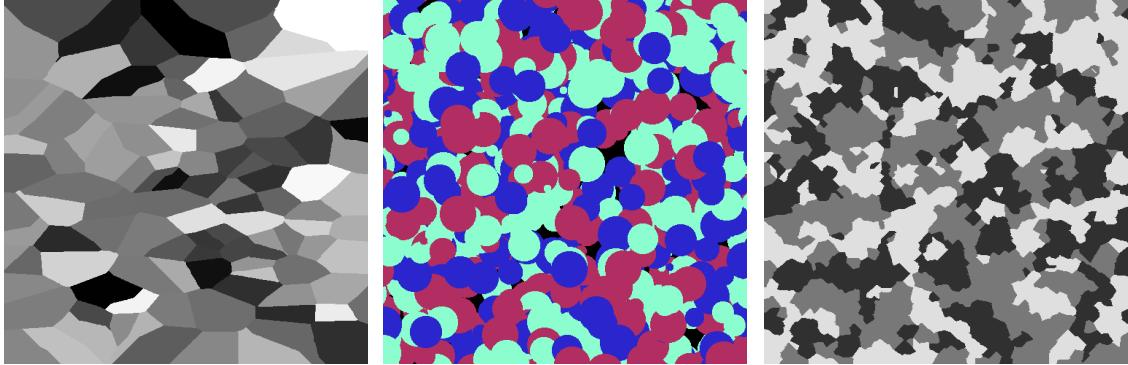
(a) Anisotropic grains obtained by deformation of the distance function.
