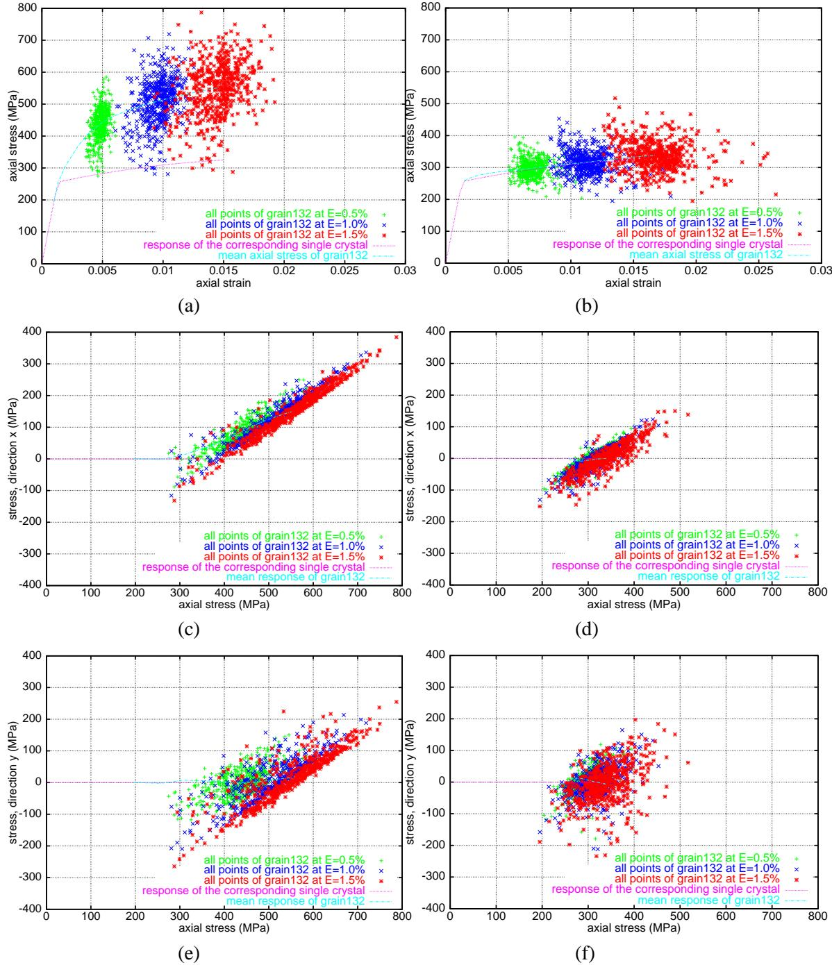
**Figure III.10 :** Intragranular heterogeneity and effect of the free surface: responses at three strains ( $E = 0.5\%, 1.0\%, 1.5\%$ ) of all the points within *grain132* (545 points); (a, b)  $\sigma_{zz}$  vs  $\epsilon_{zz}$ , (c, d)  $\sigma_{xx}$  vs  $\sigma_{zz}$ , (e, f)  $\sigma_{yy}$  vs  $\sigma_{zz}$ ; (left) case F.E. HSB, (right) case F.E. 4FF
