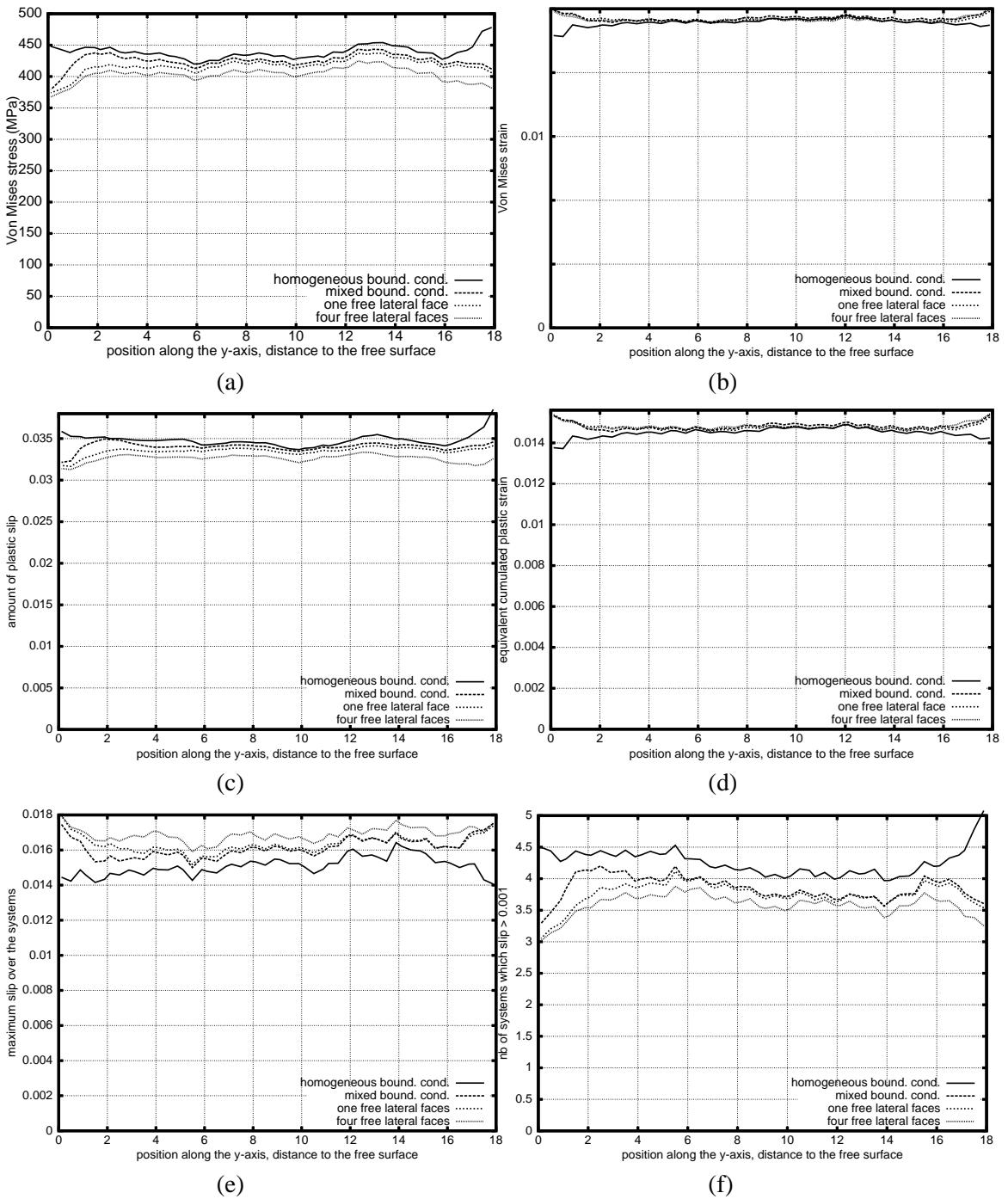
**Figure III.11 :** Variables averaged in planes parallel to a lateral face of the polycrystal in the four cases of load: (a) equivalent stress, (b) equivalent strain (c) amount of plastic slip, (d) equivalent cumulated plastic strain, (e) maximum plastic slip over the twelve systems, (f) number of slip systems whose plastic slip exceed 0.001
