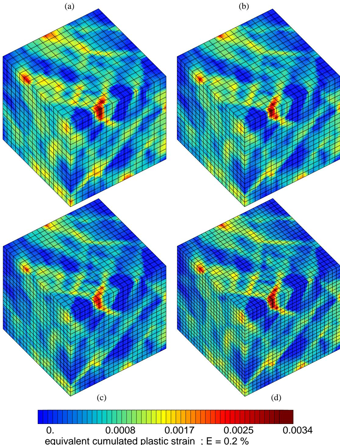
**Figure II.15** : Effect of the mesh size on the local behavior of the *m4-200-200* microstructure after 0.2% simple tension: (a)  $16^3$  quadratic elements, (b)  $18^3$  quadratic elements, (c)  $20^3$  quadratic elements, (d)  $24^3$  quadratic elements
