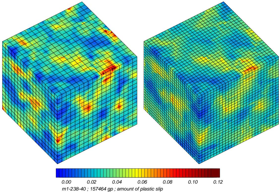
**Figure II.10 :** Effect of the interpolation mode on the local slip activity of the *m1-238-40* distribution subjected to isovolumic loading conditions: (left) 5832 quadratic elements, 157464 integration points, (right) 19683 linear elements, 157464 integration points
