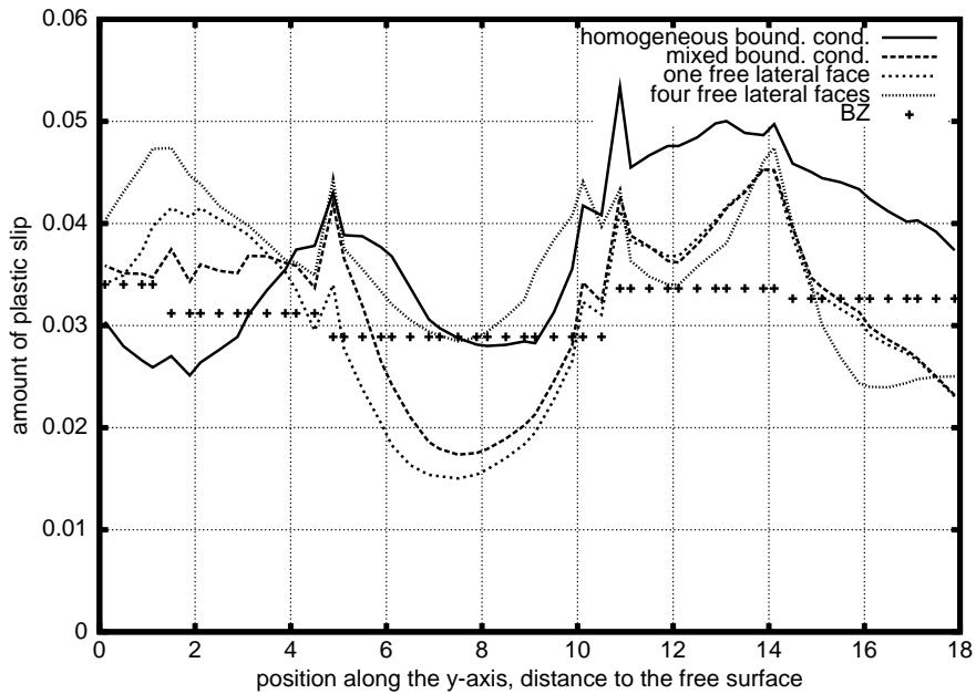
**Figure III.12 :** Evolution of the amount of plastic slip on a line perpendicular to the free surface of the polycrystal in the four cases of load; the line is located in the core and goes from side to side
