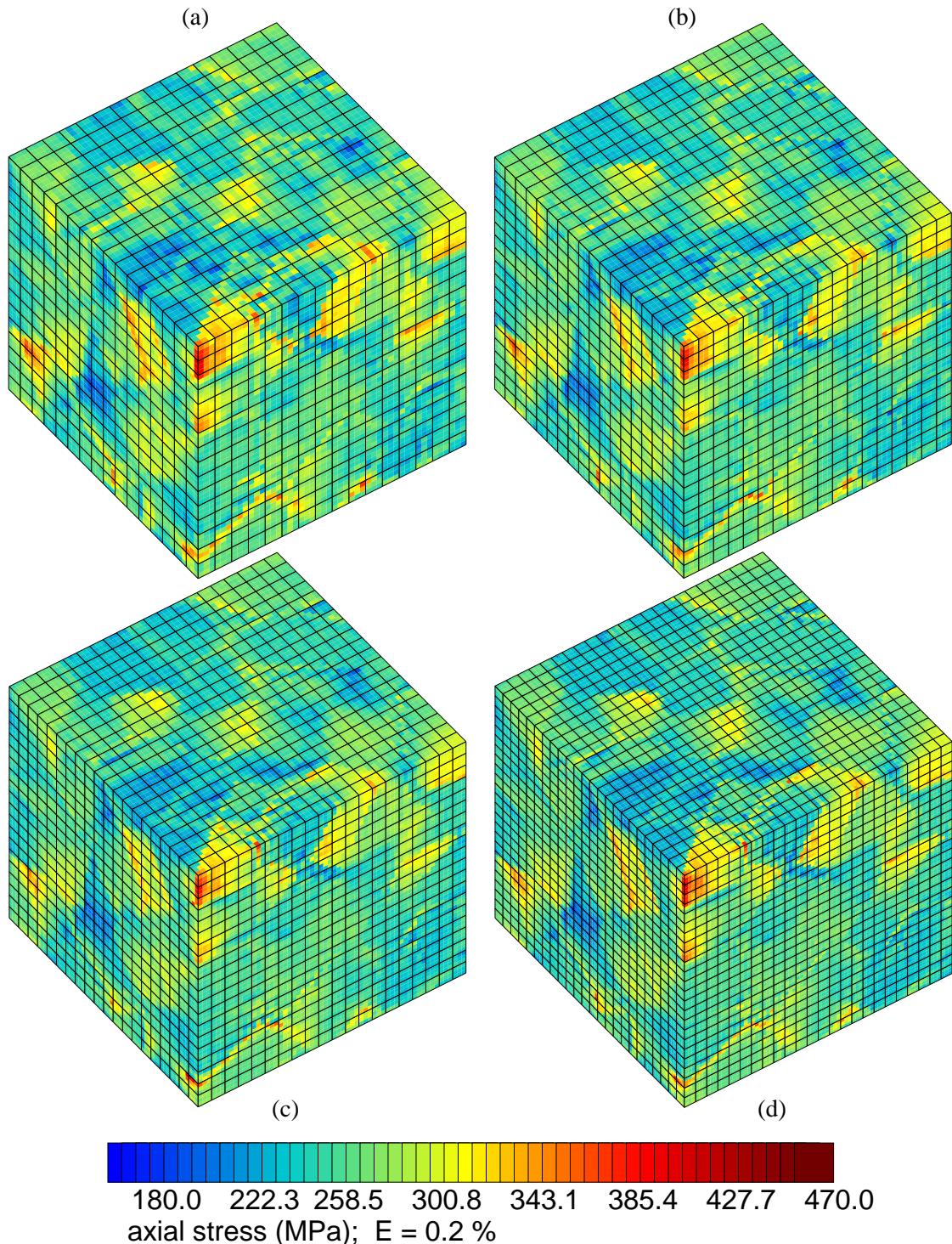
**Figure II.14 :** Effect of the mesh size on the local behavior of the *m4-200-200* microstructure after 0.2% simple tension: (a)  $16^3$  quadratic elements, (b)  $18^3$  quadratic elements, (c)  $20^3$  quadratic elements, (d)  $24^3$  quadratic elements
