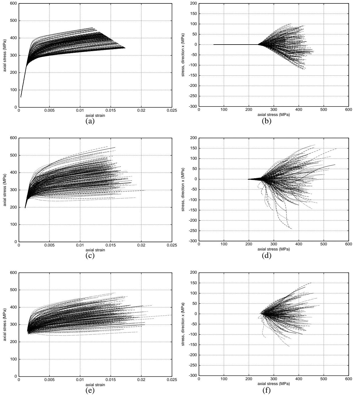
**Figure III.2 :** Illustration of inter- and intra-granular heterogeneity from the mean response of each of the 200 grains of the polycrystal: (a,b) BZ-homogenisation; (c,d) F.E. HSB; (e,f) F.E. 4FF; (left)  $\sigma_{zz}$  vs  $\varepsilon_{zz}$ , (right)  $\sigma_{xx}$  vs  $\sigma_{zz}$
