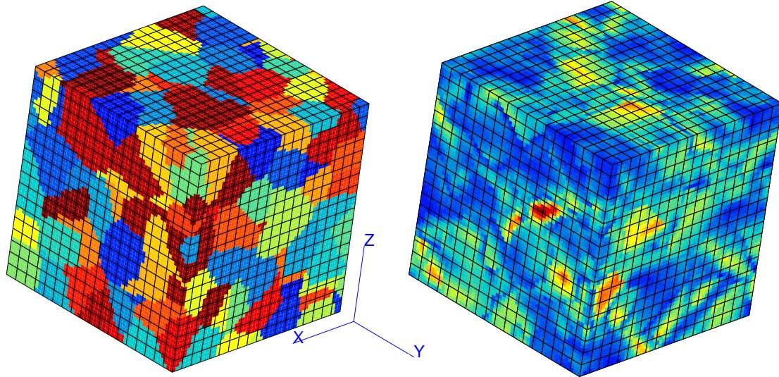
**Figure III.6 :** (left) Grain map, (right) contour of the norm of the lattice rotation vector at the onset of plastic deformation
