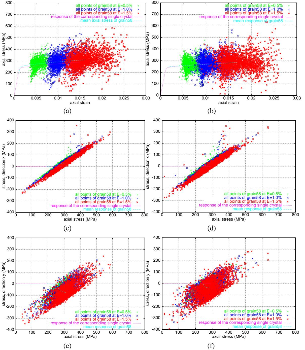
**Figure III.9 :** Intragranular heterogeneity and effect of the free surface: responses at three strains ( $E = 0.5\%, 1.0\%, 1.5\%$ ) of all the points within *grain58* (2265 points); (a, b)  $\sigma_{zz}$  vs  $\varepsilon_{zz}$ ; (c, d)  $\sigma_{xx}$  vs  $\sigma_{zz}$ ; (e, f)  $\sigma_{yy}$  vs  $\sigma_{zz}$ ; (left) case F.E. HSB, (right) case F.E. 4FF
