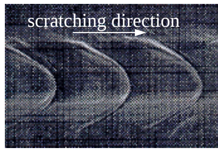
(b) Fissuration frontale. Crack initiation in front of the indenter (buckling).
