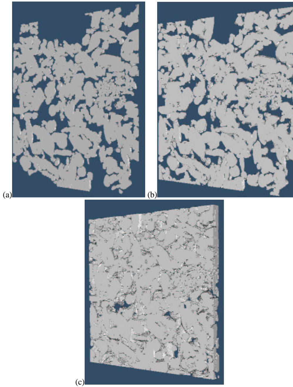
**Figure II.37** : Evolution of the percolating phase of the hard phase  $P_1$  for the sample  $SA_1$  in  $(OY)$  direction. (a) After  $3 \mu m$  ( $P_r = 0.90$ ), (b) after  $10 \mu m$  ( $P_r = 0.98$ ) and (c) the whole sample, after  $30 \mu m$  ( $P_r = 1$ ).
