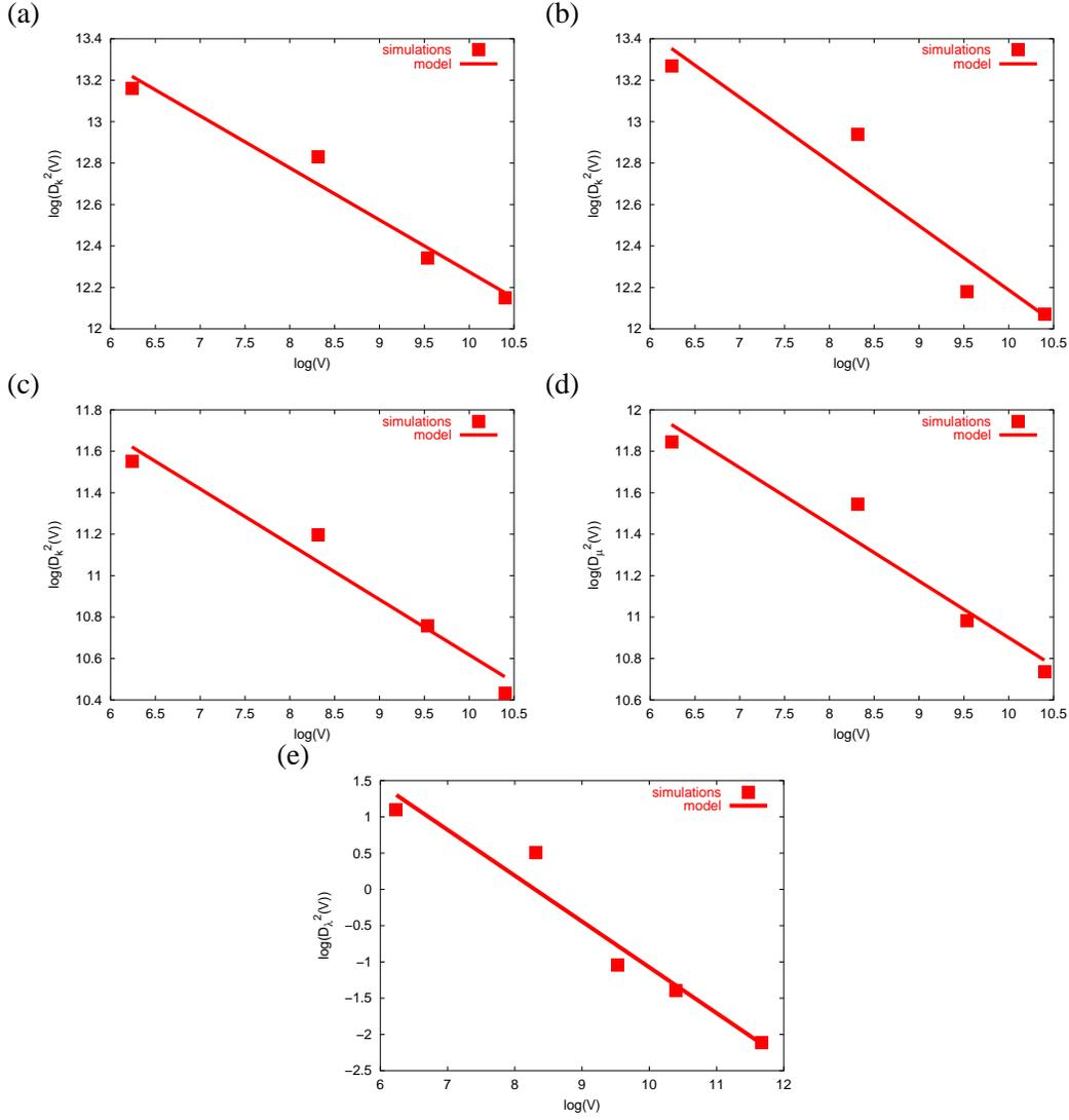
**Figure II.29** : Quality of the fit for the specimen  $SA_2$  in regular decomposition, (a)  $k$  for KUBC, (b)  $k$  for periodic, (c)  $\mu$  for KUBC, (d)  $\mu$  for periodic and (e)  $\lambda$  for periodic boundary conditions.
