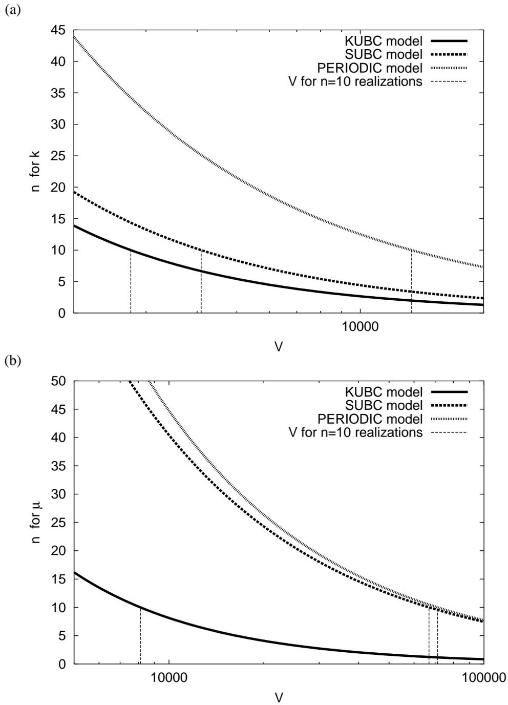
**Figure I.15** : Number of realizations as a function of the domain size for a given relative error  $\epsilon_{rela} = 1\%$  : (a) case of  $k^{app}$ , (b) case of  $\mu^{app}$ .
