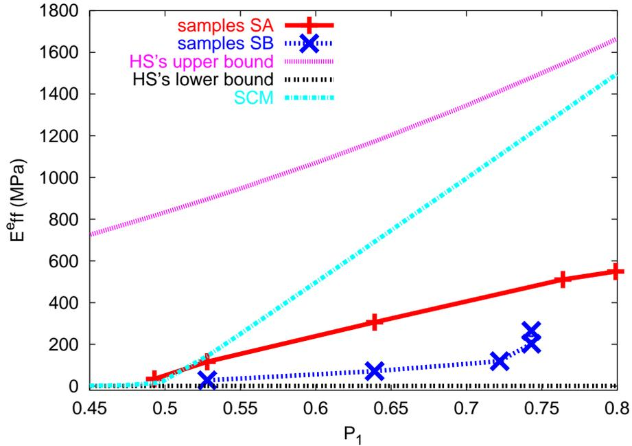
**Figure II.8** : Experimental results compared to Hashin-Shtrikman's bounds and self-consistent model (SCM) for Young's modulus. The bounds are very far apart and the self-consistent model gives the same result for different morphologies.
