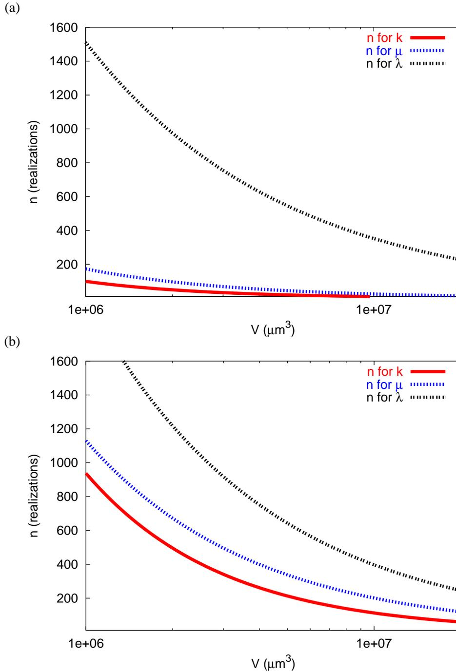
**Figure II.30** : Number of fields (for bulk modulus  $k$ , shear modulus  $\mu$  and thermal conductivity  $\lambda$ ) as a function of the domain size (for large domain size) for a given relative error  $\epsilon_{rela} = 1\%$  : (a) for the specimen  $SA_2$  and (b) for the specimen  $SB_1$ .
