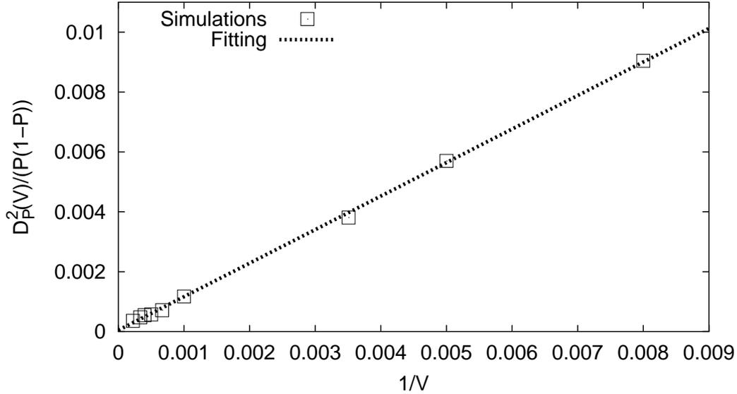
**Figure I.9** : Fitting of  $\frac{D_P^2(V)}{P(1-P)}$  as a function of the inverse of the volume of the field for volume fraction  $P = 70\%$ . The slope provides the value of the integral range  $A_3$  for the volume fraction.
