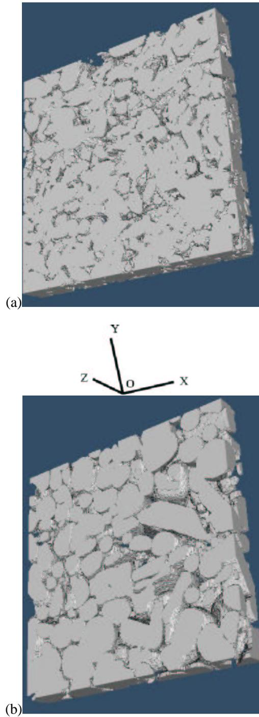
**Figure II.1** : Examples of studied microstructures obtained by confocal imaging in 3D, the size of the image is  $250 \times 250 \times 30 \mu m$ . The volume fraction of hard phase (in grey color) is about 70%. (a) Sample with additive SA and (b) sample without additive SB.
