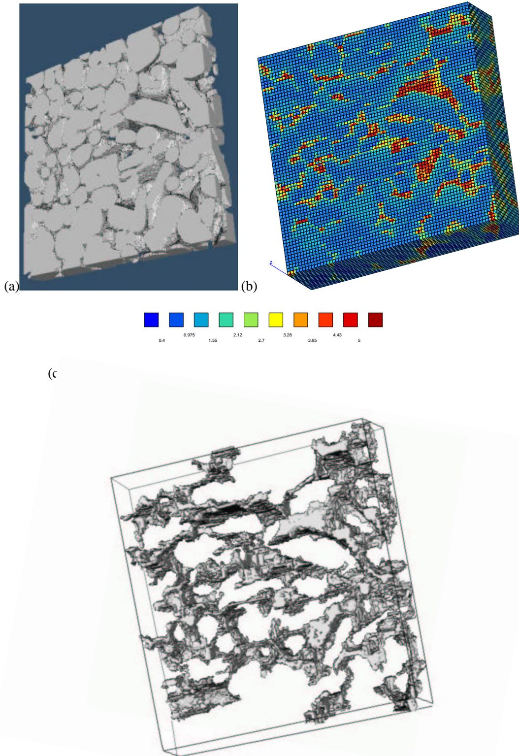
**Figure II.43** : Image of the percolated volume  $P_p$  for the variable  $\varepsilon_{eq}$  for the computation using the sample  $SB_1$ . The imposed strain tensor (loading) is  $E_{22} = 1$ . The percolation is given in the direction  $(OX)$ . (a) The whole sample, (b) map of  $\varepsilon_{eq}$  and (c) percolated volume for  $\varepsilon_{eq} = 0.5$  ( $P_r = 0.95$ ).
