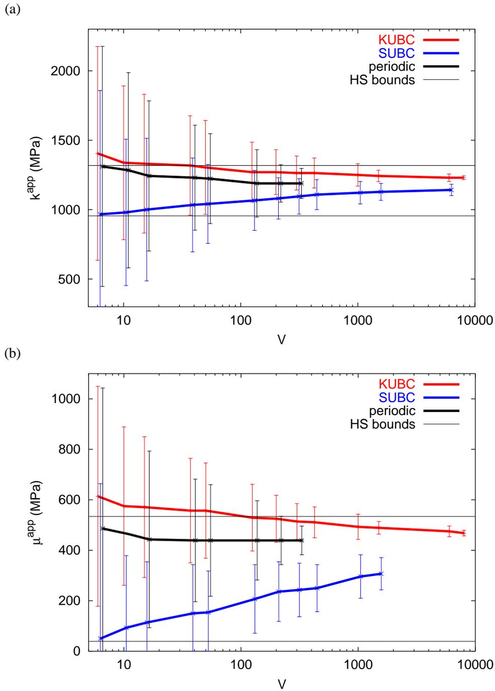
**Figure I.7** : Mean values and intervals of confidence on the mean value for the bulk modulus  $k^{app}$  (a) and (b) for the shear modulus  $\mu^{app}$ , as a function of domain size ( $P_1 = 70\%$ ). Three different types of boundary conditions are considered. For clarity, the errorbars are slightly shifted around each studied domain size.
