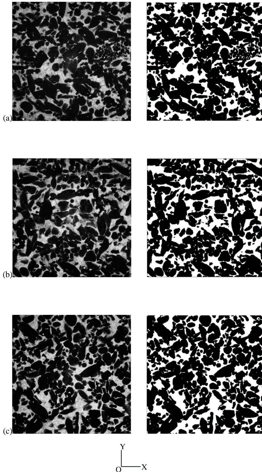
**Figure II.3 :** Specimens  $SA$ , confocal and thresholded images, (a)  $SA_1$ , (b)  $SA_2$ , (c)  $SA_3$ . The size of images is  $250 \times 250 \mu m$ . The hard phase is in dark color in confocal and thresholded images.
