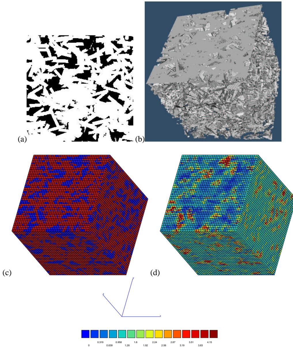
**Figure III.3** : Boolean model with 70% of plate hexagons ( $P70$ ). (a) The first section in plane  $XY$ , (b) the 3D image, (c) finite element mesh and (d) map of equivalent strain  $\epsilon_{eq}$  with loading  $E_{22} = 1$  under KUBC boundary conditions.
