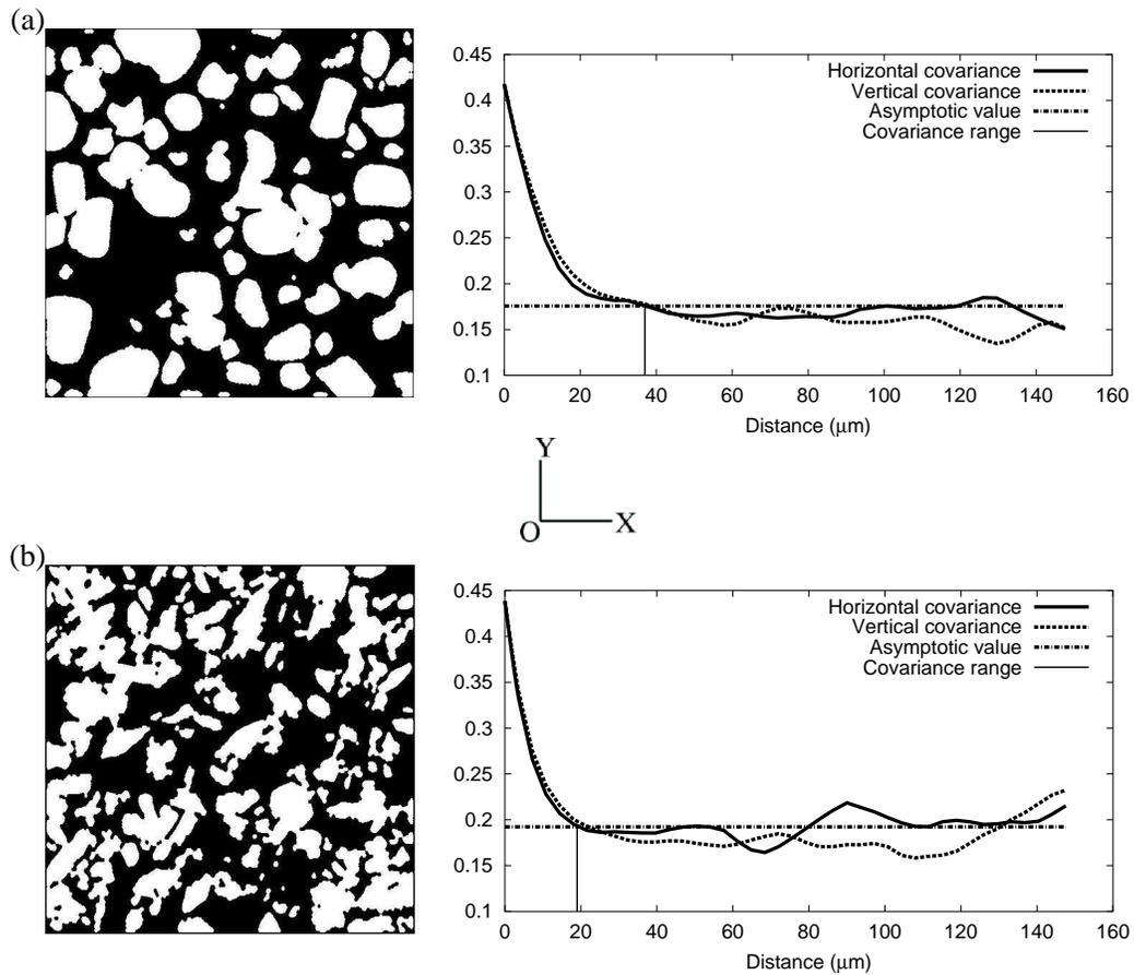
**Figure I.1** : Microstructures (with the same volume fraction and different morphologies) and their covariances in horizontal and vertical directions; the image size is  $150\mu m \times 150\mu m$ . The asymptotic value is equal to the square of the volume fraction (of the white phase); for the fine (a) and coarse (b) microstructures (material from food industry, (Colworth, 2000)).
