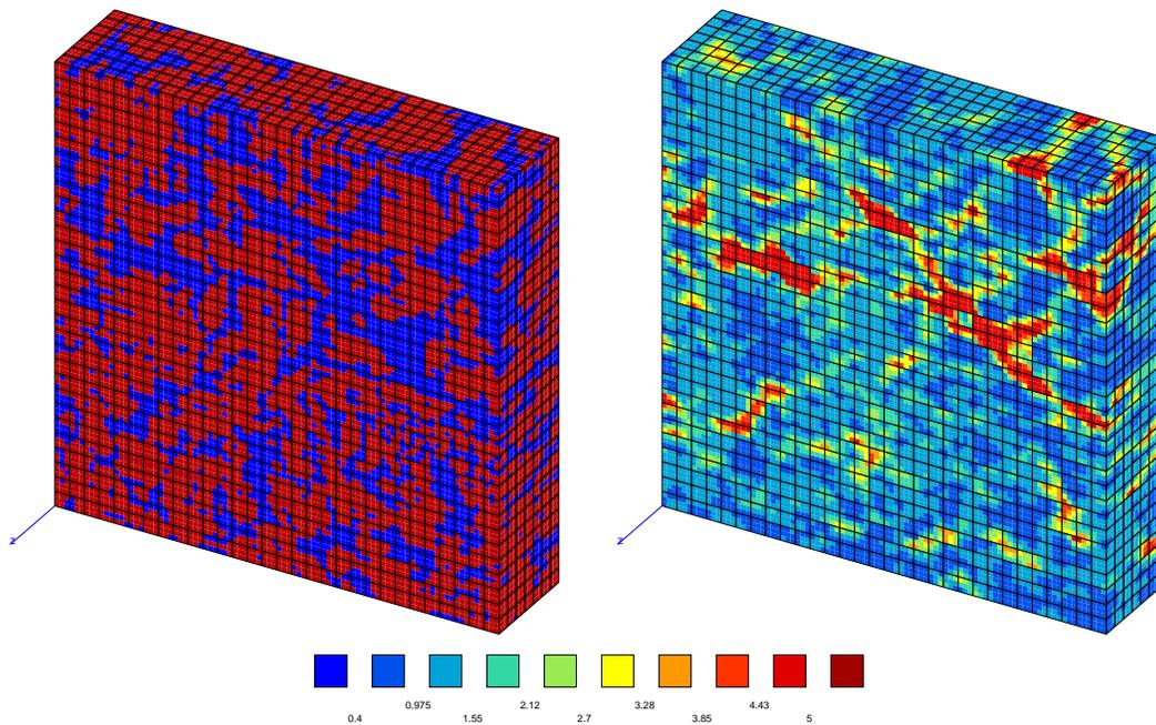
**Figure II.13** : Mesh and computation with 6300 elements (87885 d.o.f.), or  $298 \mu m^3$ /element and map of equivalent strain.
