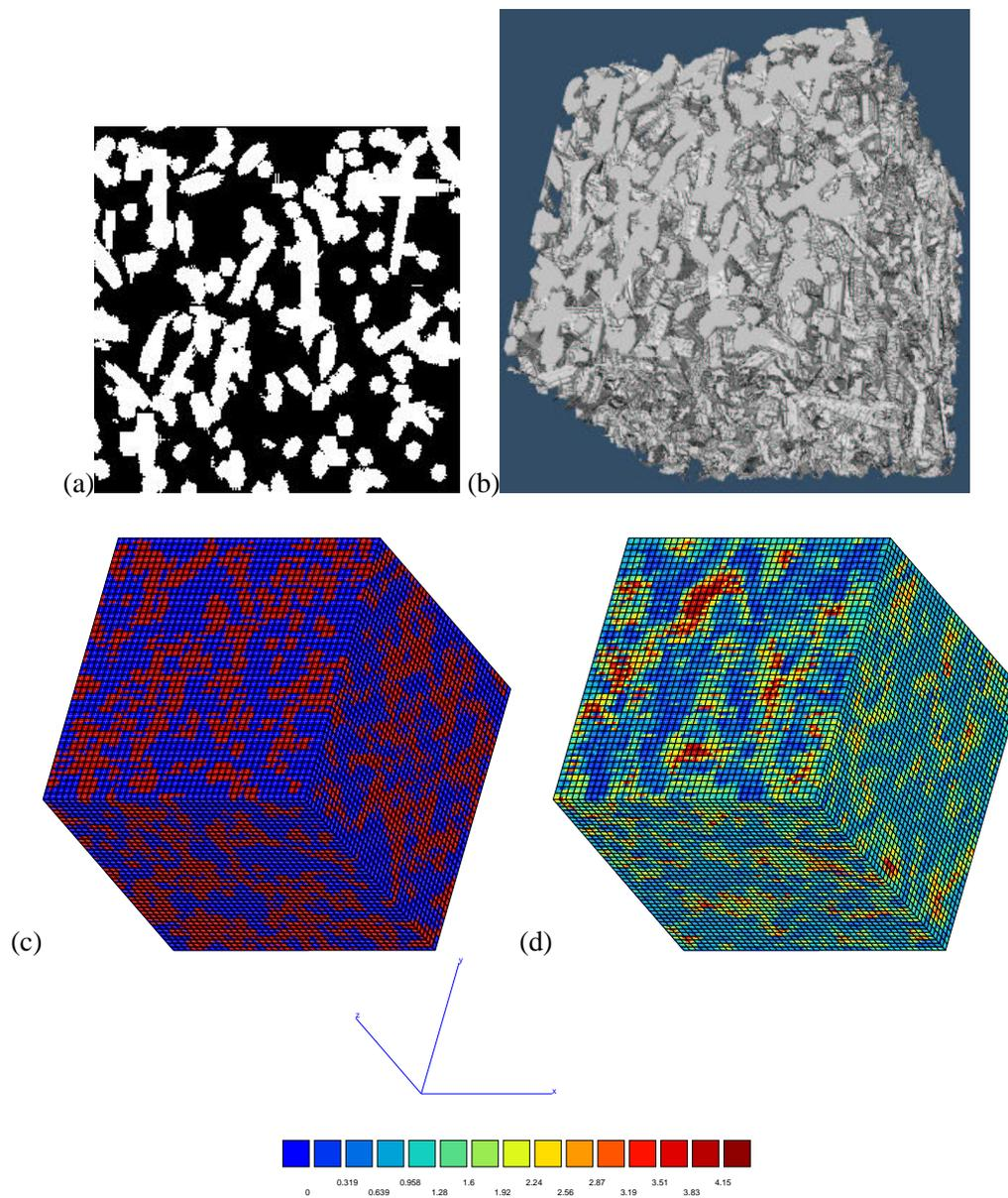
**Figure III.4** : Boolean model with 50% of rod hexagons ( $R50$ ). (a) The first section in plane  $XY$ , (b) the 3D image, (c) finite element mesh and (d) map of equivalent strain  $\varepsilon_{eq}$  with loading  $E_{22} = 1$  under KUBC boundary conditions.
