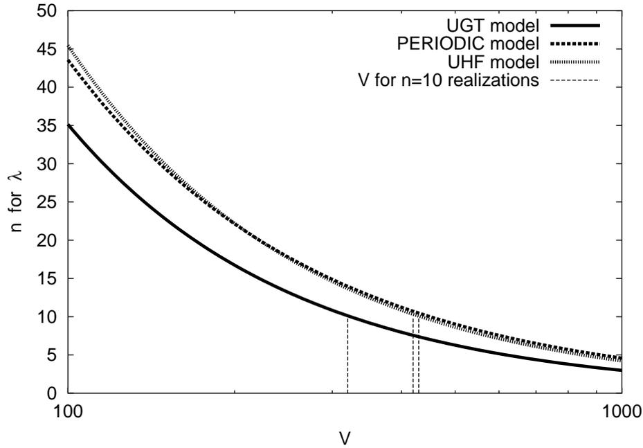
**Figure I.16** : Number of realizations as a function of the domain size, necessary to obtain an absolute precision  $\epsilon_{abs} = 0.05 W/mK$  on the mean value of apparent thermal conductivity  $P = 70\%$ .
