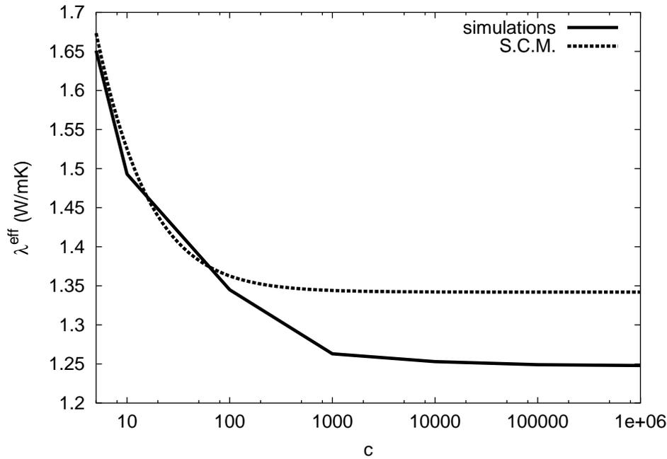
**Figure I.17** : Effective thermal conductivity of Voronoï mosaics as function of the contrast of properties  $c$  (the thermal conductivity  $\lambda_1 = 2.44 \text{ W/mK}$  is kept constant,  $P_1 = 70\%$ ) : comparison with the self-consistent estimate. The numerical estimation of the effective conductivity is obtained by finite element simulations with periodic boundary conditions on a volume  $V = 125$  and  $n = 1020$  realizations for each value of  $c$ . The mean value is plotted.
