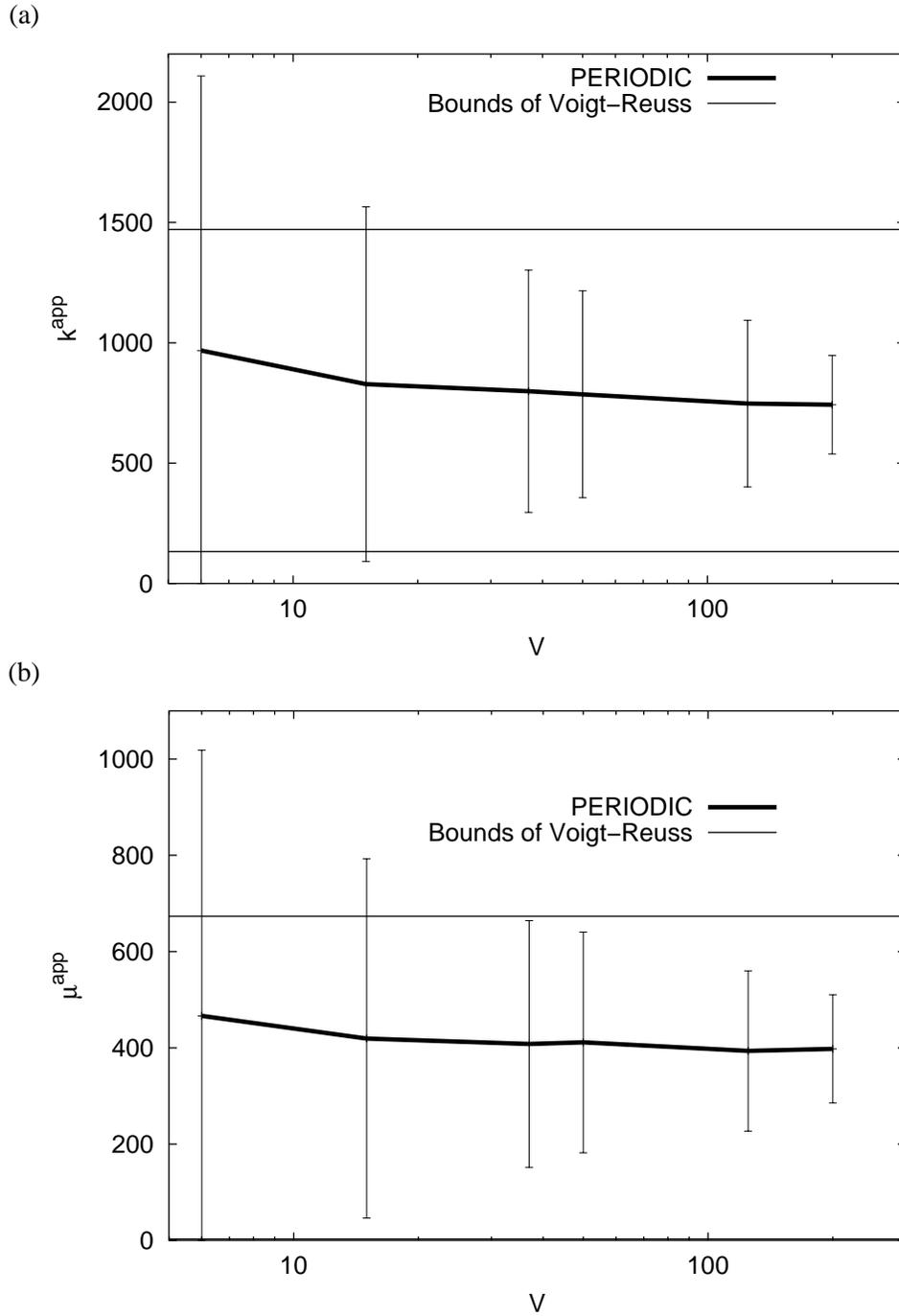
**Figure I.12** : Dispersion and mean value of the apparent elastic properties as a function of the domain size for periodic boundary conditions in the case ( $c = 1000$ ,  $P = 70\%$ ) : (a) evolution of  $k^{app}$  and (b) evolution of  $\mu^{app}$ .
