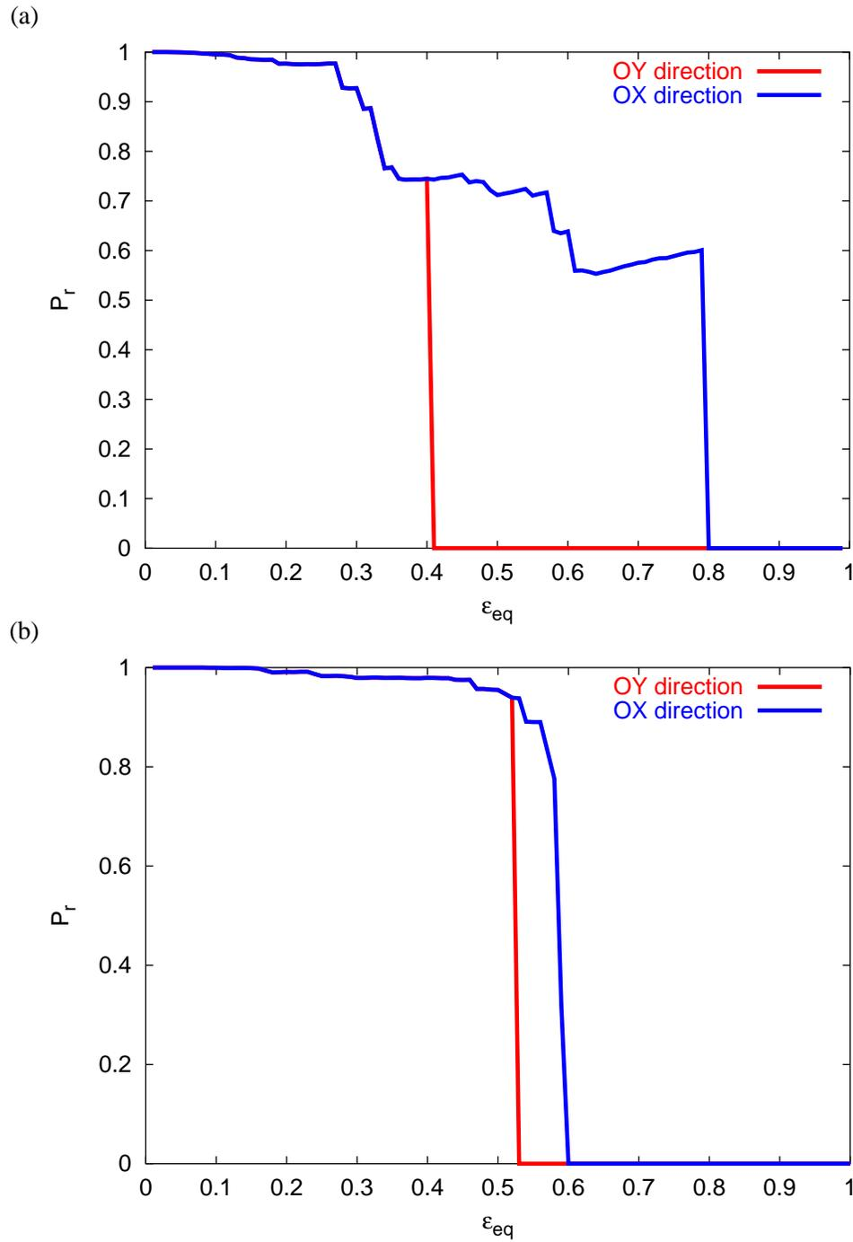
**Figure II.41** : Evolution of the strain field percolation ratio as a function of the equivalent strain threshold. (a) Example of computation of the sample  $SA_1$  with  $E_{22} = 1$  and (b) computation of the sample  $SB_1$  with  $E_{22} = 1$ .
