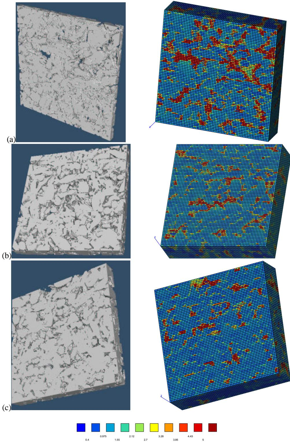
**Figure II.22** : Direct numerical simulation of samples with additive  $SA$ , example of computation with  $E_{22} = 1$ . in KUBC. The map of equivalent strain  $\varepsilon_{eq}$  is shown. The hard phase  $P_1$  is in grey color.
