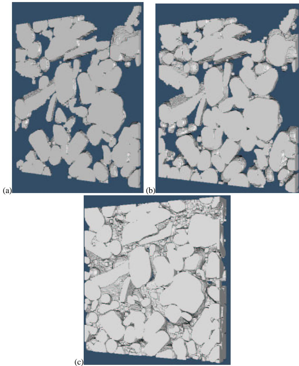
**Figure II.40** : Evolution of the percolating phase of the hard phase  $P_1$  for the sample  $SB_3$  in  $(OY)$  direction. (a) After  $6 \mu m$  ( $P_r = 0.89$ ), (b) after  $10 \mu m$  ( $P_r = 0.93$ ) and (c) the whole sample, after  $30 \mu m$  ( $P_r = 1$ ).
