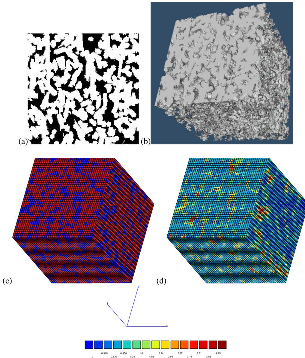
**Figure III.5** : Boolean model with 70% of rod hexagons ( $R70$ ). (a) The first section in plane  $XY$ , (b) the  $3D$  image, (c) finite element mesh and (d) map of equivalent strain  $\varepsilon_{eq}$  with loading  $E_{22} = 1$  under KUBC boundary conditions.
