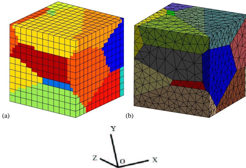
**Figure I.3** : Two meshes of the same microstructure (20 Voronoï cells) with approximately the same number of integration points (*i.p.*) and the same number of degrees of freedom (*d.o.f.*) : (a) multi-phase elements (13824 *i.p.* and 6591 *d.o.f.*), (b) free meshing (10326 *i.p.* and 6387 *d.o.f.*).
