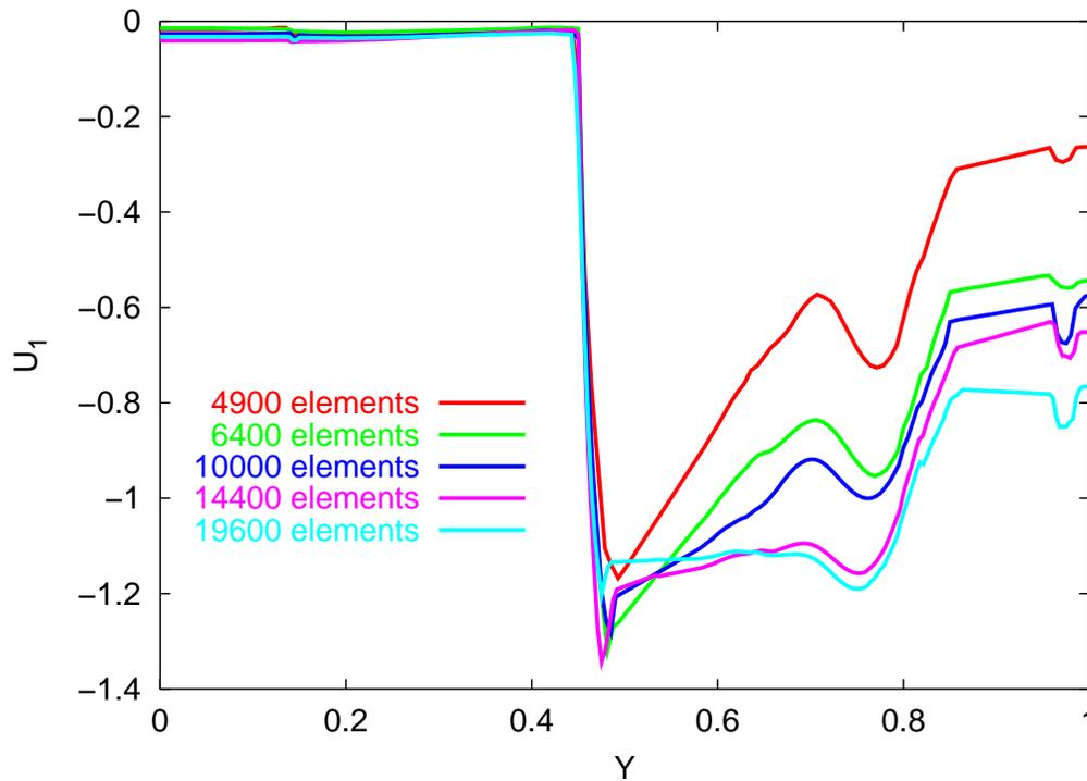
**Figure II.21** : Convergence of results in  $2D$ , displacement  $U_1$ .
