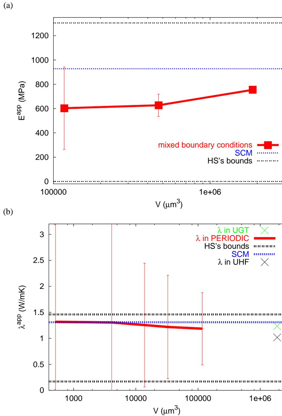
**Figure II.25** : Mean values and intervals of confidence on the mean value for Young's modulus  $E^{\text{app}}$  (a) and thermal conductivity (b) as a function of the domain size for the specimen  $SA_2$ .
