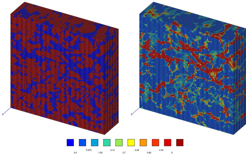
**Figure II.15** : Mesh and computation with 88200 elements (1126131 d.o.f.), or  $22 \mu\text{m}^3/\text{element}$  and map of equivalent strain.
