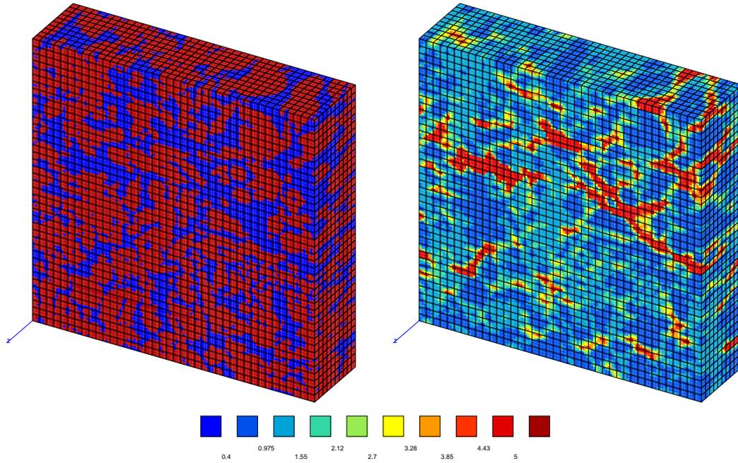
**Figure II.14** : Mesh and computation with 16000 elements (214143 d.o.f.), or  $117 \mu\text{m}^3/\text{element}$  and map of equivalent strain.
