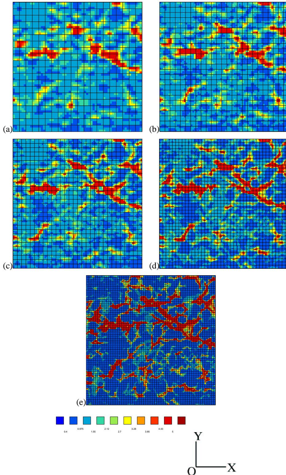
**Figure II.16** : Local convergence as a function of mesh density in 3D case : (a) 2000 elements, (b) 3750 elements, (c) 6300 elements, (d) 16000 elements and (e) 88200 elements. These maps are the first section of figures II.11 to II.15.
