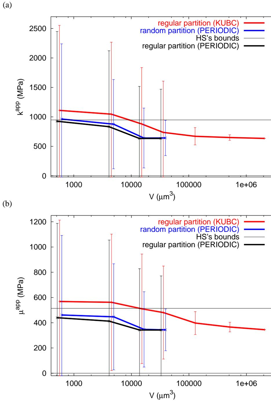
**Figure II.28** : Mean values and intervals of confidence on the mean value for the bulk modulus  $k^{app}$  (a) and (b) for the shear modulus  $\mu^{app}$  as a function of domain size for the specimen  $SA_2$ . The upper and lower bounds are (1430, 2.65 MPa) for  $k$  and (660, 0.05 MPa) for  $\mu$ .
