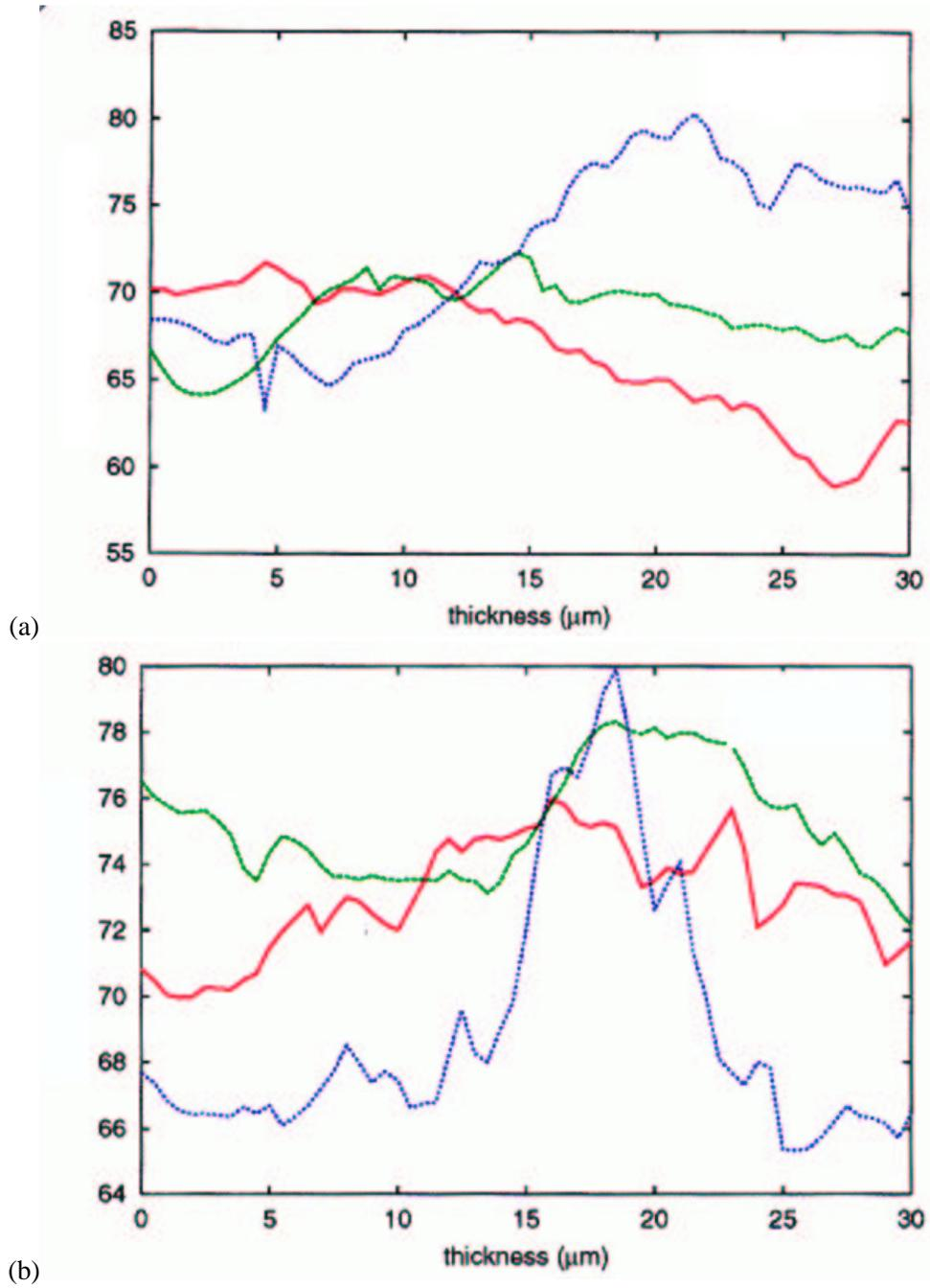
**Figure II.2** : Evolution of the area fraction of hard phase  $P_1$  (%) in thickness direction, (a) samples with additive  $SA$  and (b) samples without additive  $SB$ . An important variation is observed in samples with additive  $SA$ .
