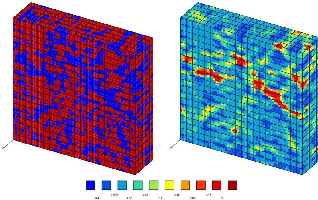
**Figure II.11** : Mesh and computation with 2000 elements (29673 d.o.f.), or  $938 \mu m^3/element$  and map of equivalent strain  $\varepsilon_{eq}$  for a mean prescribed strain  $E_{22} = 1$ .
