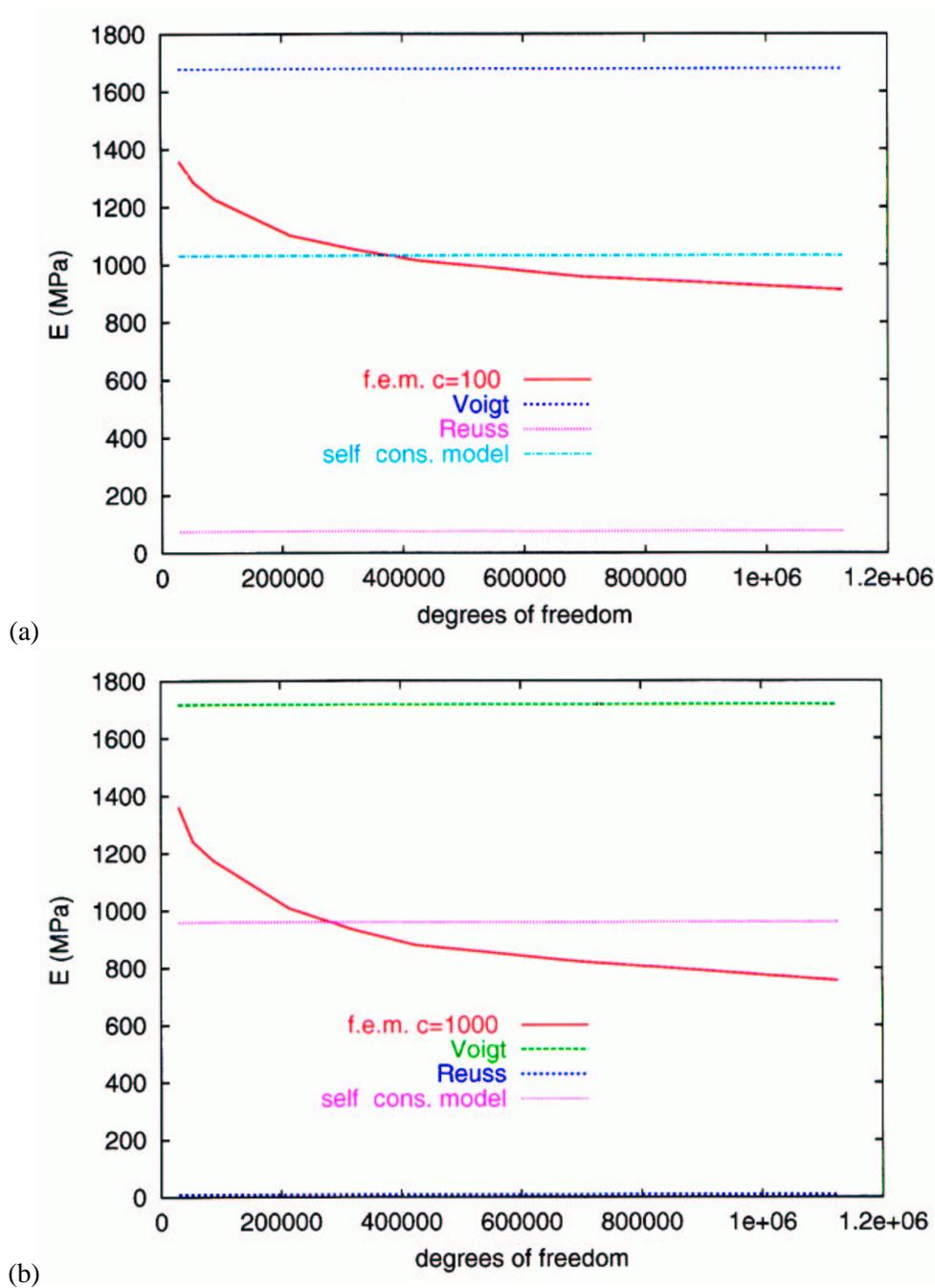
**Figure II.10** : Effect of the mesh density in finite element simulations (f.e.m.) on the global convergence of the apparent Young's modulus. The Hashin-Shtrikman's bounds are (1322, 140 MPa) for the specimen (a)  $SA_1$  and (1314, 16 MPa) for the specimen (b)  $SA_2$ .  $c = c_E$  represents the contrast in the Young's moduli of the phases.
