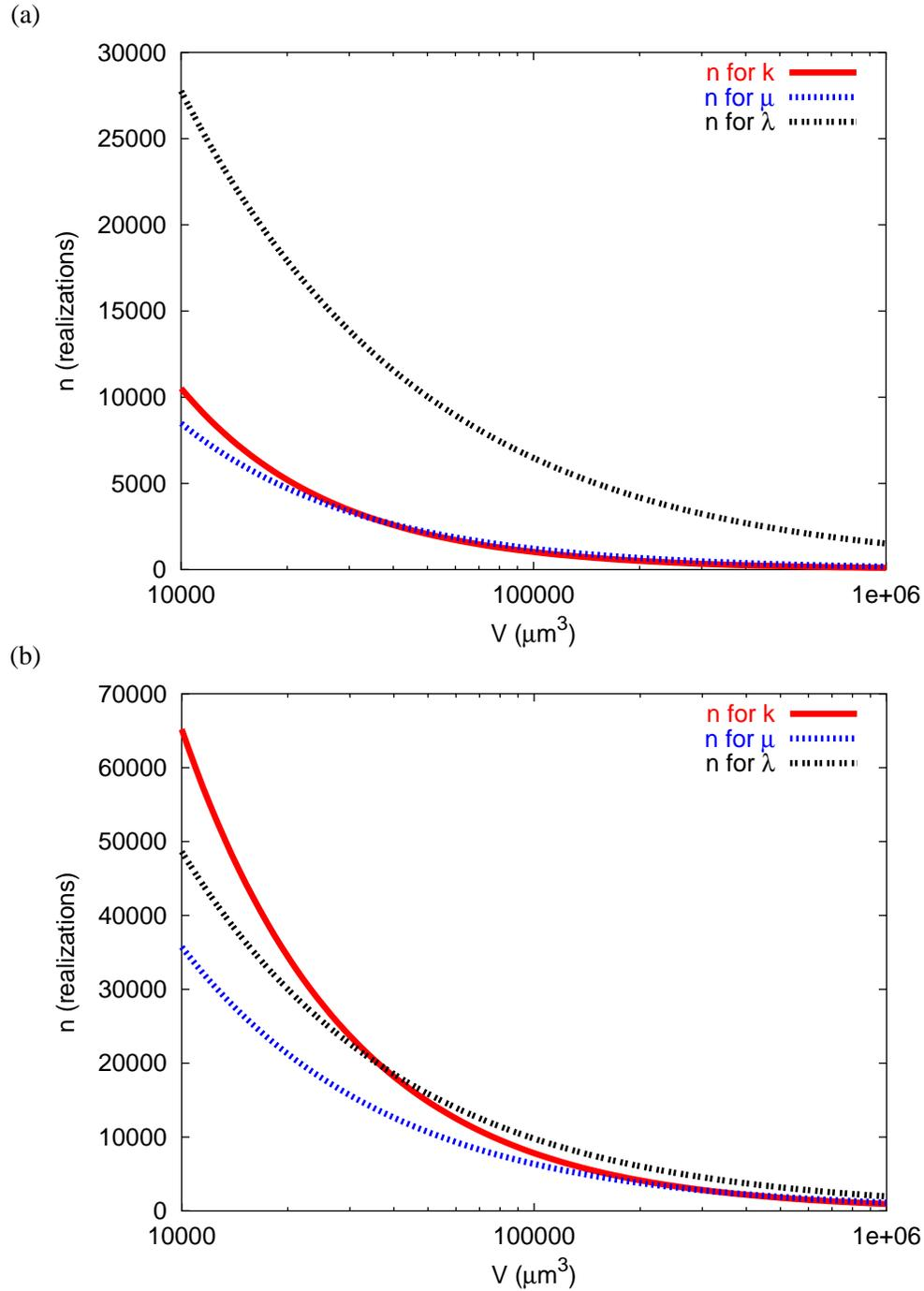
**Figure II.31** : Number of fields (for bulk modulus  $k$ , shear modulus  $\mu$  and thermal conductivity  $\lambda$ ) as a function of the domain size (for small domain size) for a given relative error  $\epsilon_{rela} = 1\%$  : (a) for the specimen  $SA_2$  and (b) for the specimen  $SB_1$ .
