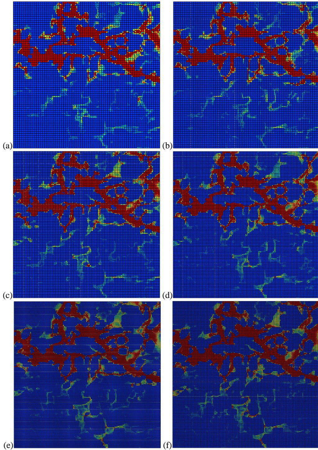
**Figure II.19** : Effect of mesh density in 2D. Maps of equivalent strain, (a) 4900 elements, (b) 6400 elements, (c) 8100 elements, (d) 10000 elements, (e) 14400 elements and (f) 16900 elements. The computations are performed with mixed boundary conditions.
