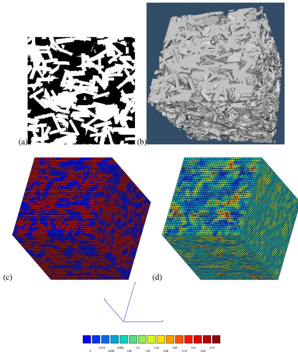
**Figure III.2** : Boolean model with 50% of plate hexagons ( $P50$ ). (a) The first section in plane  $XY$ , (b) the 3D image, (c) finite element mesh and (d) map of equivalent strain  $\varepsilon_{eq}$  with loading  $E_{22} = 1$  under KUBC boundary conditions.
