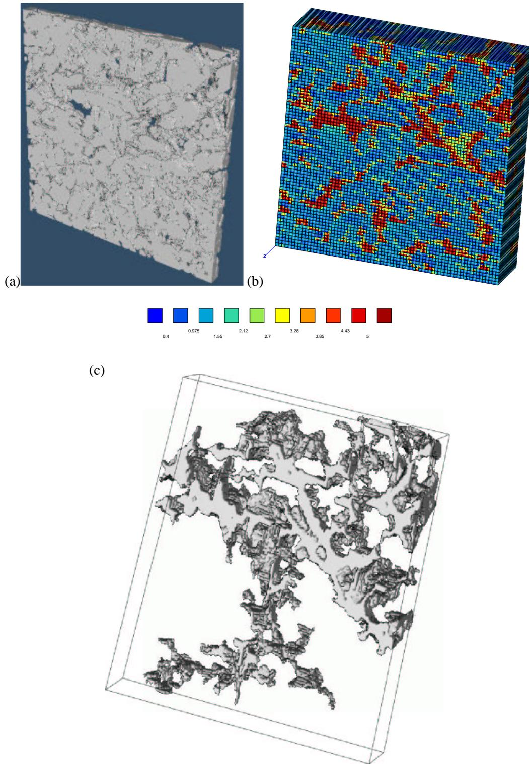
**Figure II.42** : Image of the percolated volume  $P_p$  for the variable  $\varepsilon_{eq}$  for the computation using the sample  $SA_1$ . The imposed strain tensor (loading) is  $E_{22} = 1$ . The percolation is given in the direction  $(OX)$ . (a) The whole sample, (b) map of  $\varepsilon_{eq}$  and (c) percolated volume for  $\varepsilon_{eq} = 0.4$  ( $P_r = 0.74$ ).
