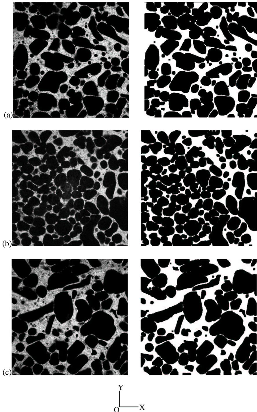
**Figure II.4 :** Specimens  $SB$ , confocal and thresholded images, (a)  $SB_1$ , (b)  $SB_2$ , (c)  $SB_3$ . The size of images is  $250 \times 250 \mu m$ . The hard phase is in dark color in confocal and thresholded images.
