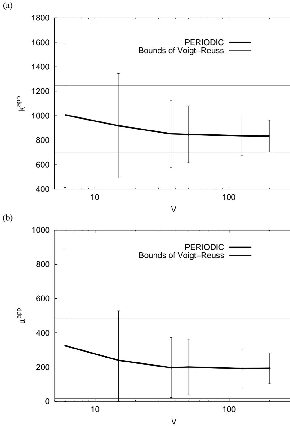
**Figure I.11** : Dispersion and mean value of the apparent elastic properties (given in  $MPa$ ) as a function of the domain size for periodic boundary conditions in the case of ( $c = 100$ ,  $P = 50\%$ ), (a) evolution of  $k$  and (b) evolution of  $\mu$ .
