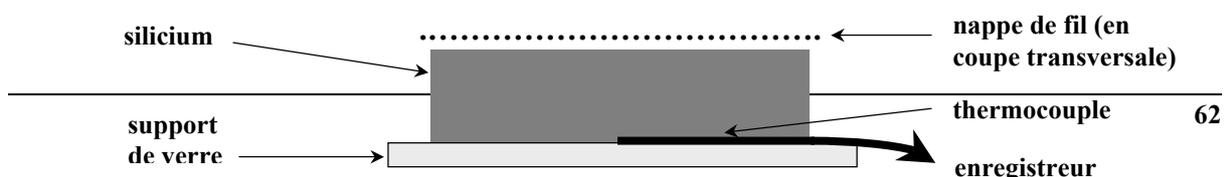
figure 2-25 : insertion du thermocouple
