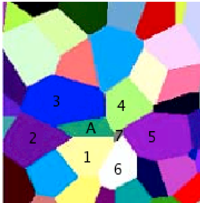
Fig. B.4 – Last step of the process detailed in figure B.3 : the new grain created is noted grain 7 and grains A, 2 and 3 has been convexed
