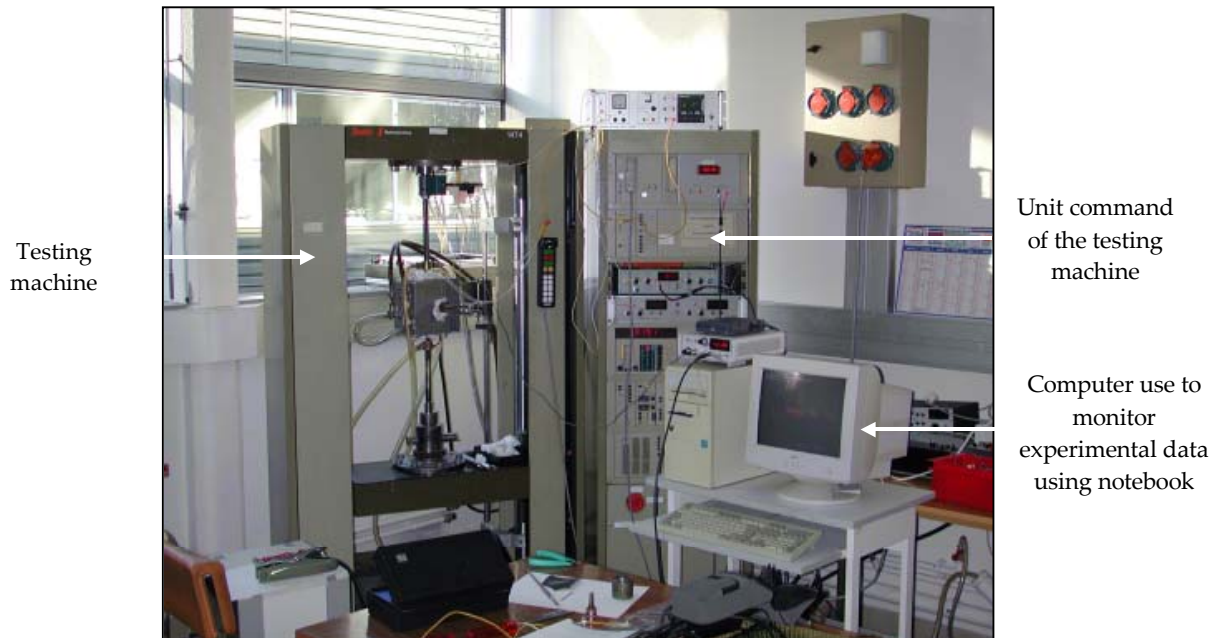
Figure B.D.1. General view of the Zwick testing machine used to perform tensile tests at high temperature
