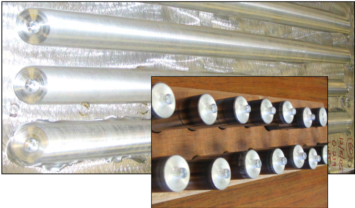
Figure 97: Photos of some experimental welding runs, and some tool utilized to study the pin length influence.
