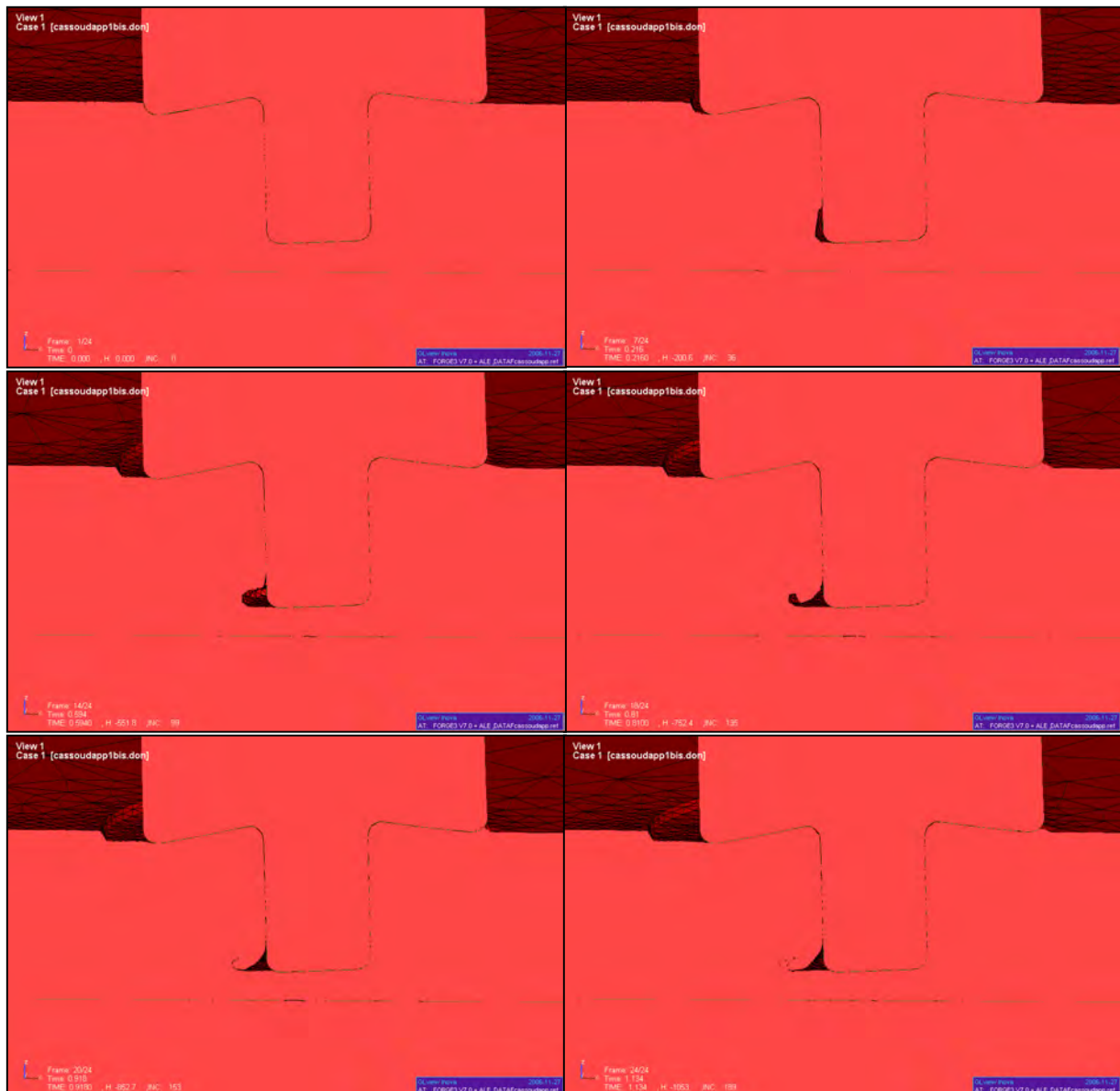
Figure 144: Initial void formation due to bad initial state (cross section view) The void tends to be field but leads to material interpenetration which is not handled by the code.
