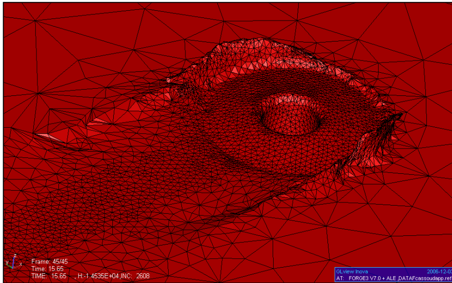
Figure 143: Example of flash occurring during an ALE simulation of transient welding phase.
