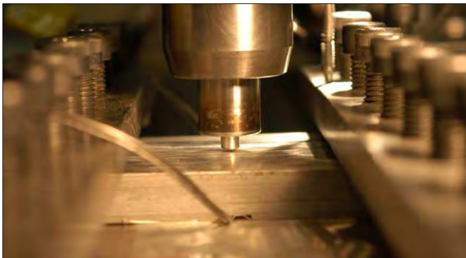
Figure 116: A view of the experimental plunge, just prior to the test. Notice the thermocouple wires extending out from the bottom of the block.
