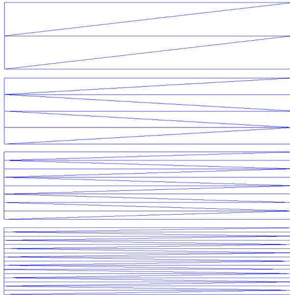
FIG. 2.17 – Maillages anisotropes (mesh anis1,...,mesh anis4).
