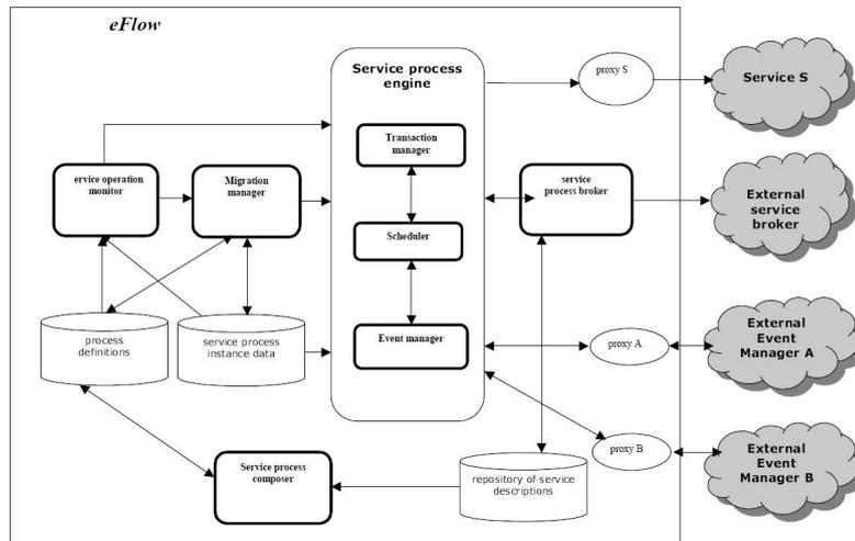
FIGURE 3.3: Plateforme eFlow
