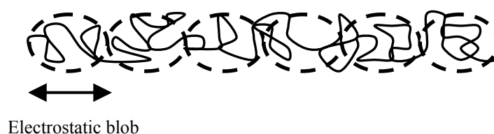
Figure 7: Polyelectrolyte chain in a dilute solution
