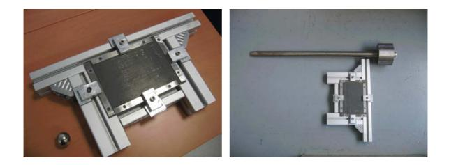
Figure 6.20: Support fixture and impactor.
