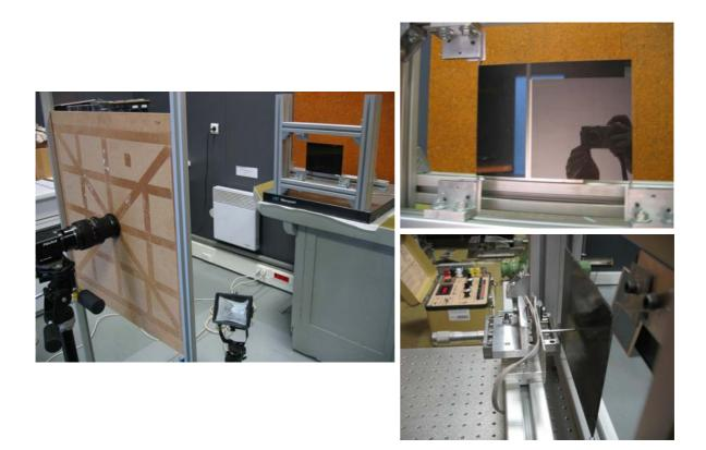
Figure 3.7: Deflectometry set-up.
