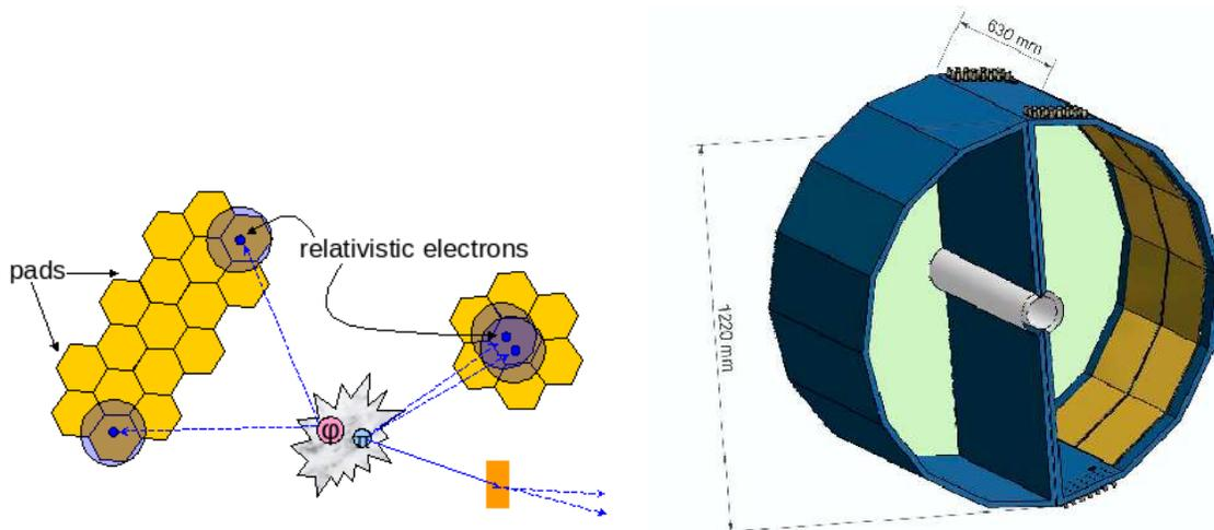
Figure II.17: Left: The hexagonally shaped pad read out. Small opening angle electrons make similar cluster to a single electron but the total photoelectron count is larger for two electrons. Right: The HBD support structure and  $\text{CF}_4$  containment vessel.
