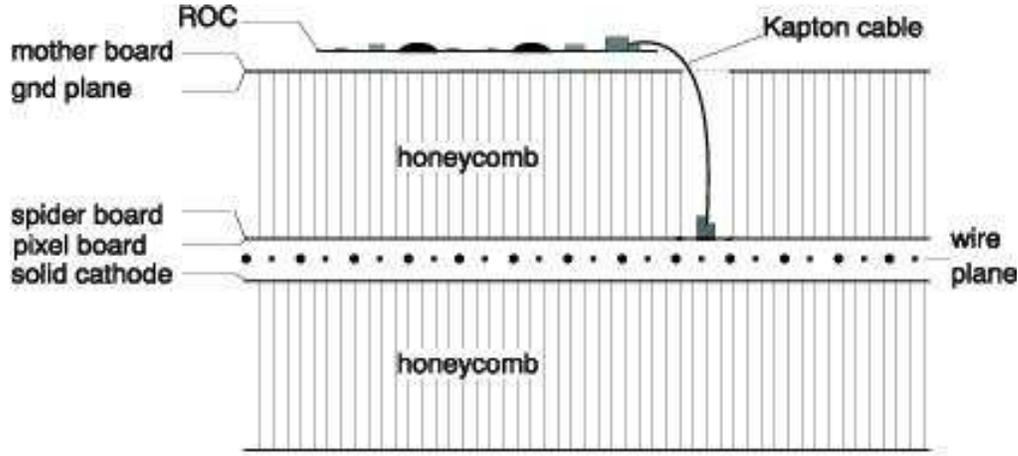
Figure II.11: Pad chamber wafer (not to scale).
