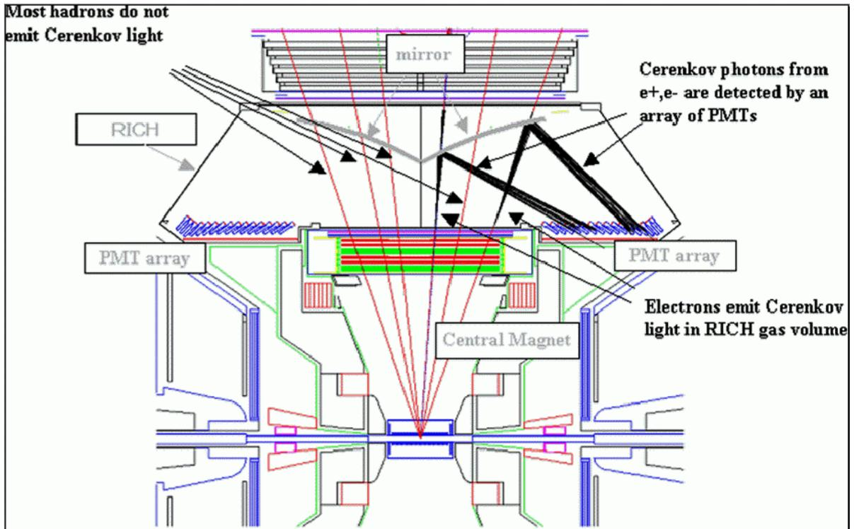
Figure II.13: Schematic cut-through view of the RICH detector.
