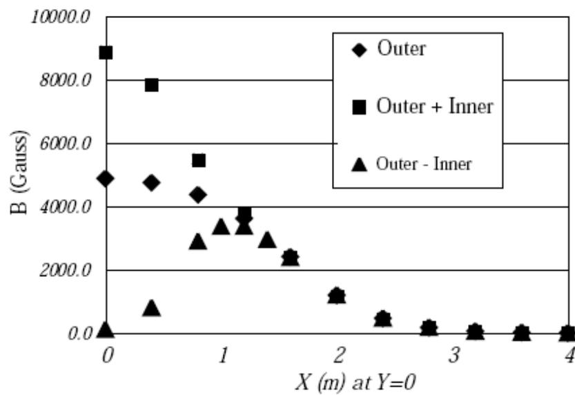
Figure II.8: The longitudinal component of the magnetic field as a function of radial distance for three configurations of the polarization in the inner and outer coils.
