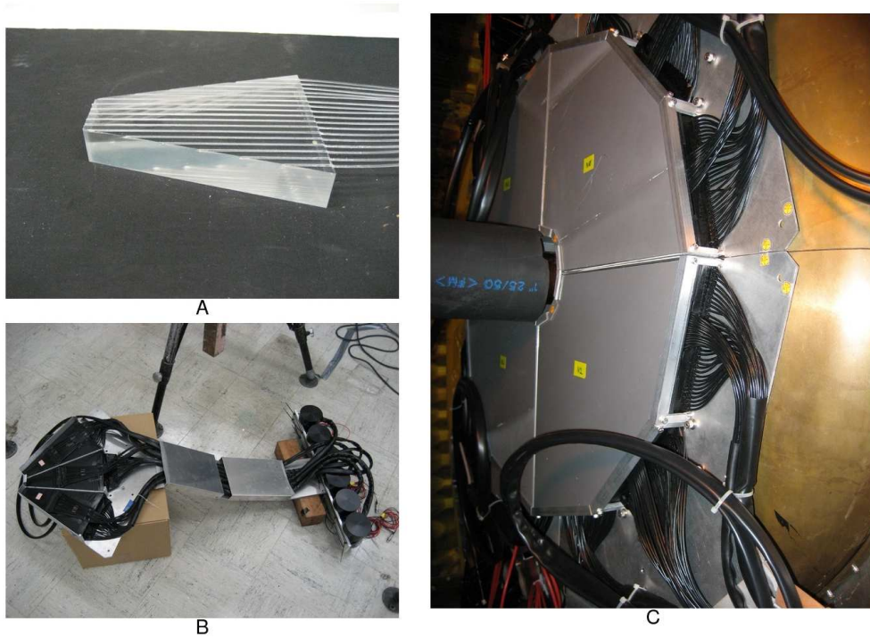
Figure II.5: RxNP detector (A) An uncovered scintillator slab - outer ring, with visible penetrating fibers (B) A fully assembled sector (three slabs) with photomultipliers (C) RxNP south fully mounted.
