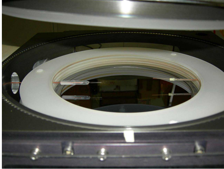
Figure 2.29: Two hairpin probes of different construction design inserted into the dual frequency plasma chamber.
