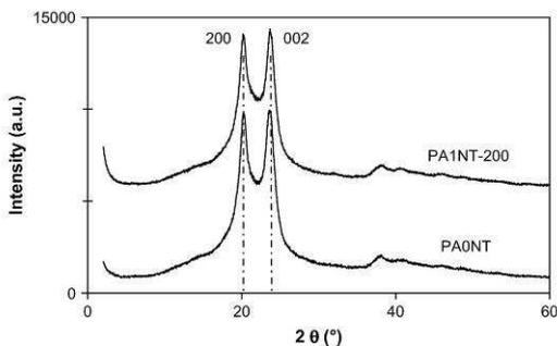
Fig. 4. WAXS patterns of neat PA-6 and PA-6/MWNT composites with 1 wt%.
