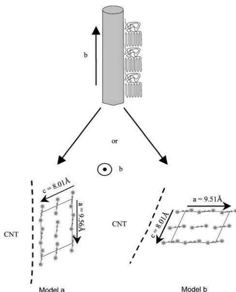
Fig. 8. Two orientations for the epitaxial growth of PA-6 lamellae with – Model a – the  $(\vec{a}, \vec{b})$  plane on the nanotube surface and – Model b – the  $(\vec{b}, \vec{c})$  plane on the nanotube surface.
