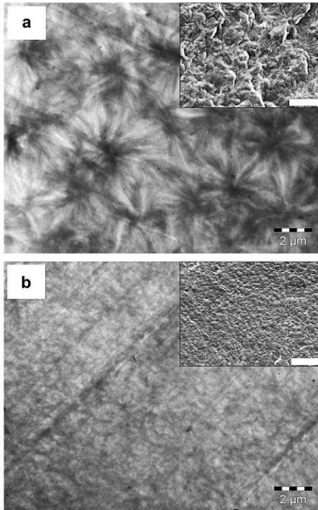
Fig. 6. TEM images of PA-6/MWNT composites with (a) 0 wt%, (b) 0.1 wt% and inset shows the SEM images of the same composites – scale bar 2 μm for TEM and 5 μm for SEM.
