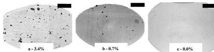
Fig. 1. Optical microscopy images of PA-6/MWNT composites with 1 wt% loading after melt mixing with the indication of the proportion of surface covered by dark spots – scale bar 400  $\mu$ m – (a) PA1NT-50, (b) PA1NT-100, (c) PA1NT-200.
