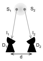
Figure 1.2: Scheme of the intensity interferometer. The light coming from a star is detected on two detectors separated by a distance d. The correlation between the detected intensities  $I_1$  and  $I_2$  is then measured.
