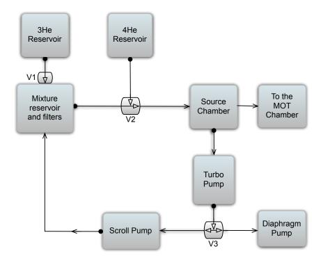
Figure 2.3: Sketch of the recycling system used in the Amsterdam setup when <sup>3</sup>He is injected in the apparatus (see text).
