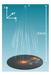
Figure 1.10: Sketch of the experimental setup used in the Amsterdam-Palaiseau experiment. A metastable helium cloud is released at the switch-off of the magnetic trap. The atoms fall under the effect of gravity on a 3D single atom detector situated 63 cm below the trap.
