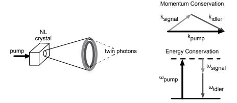
Figure 4.1: Illustration of the phase-matching conditions in parametric down-conversion processes. In case of type-I phase-matching the correlated photons are emitted on two concentric cones, as shown in the left side of the figure. On the right side of the figure energy and momentum conservation are illustrated.
