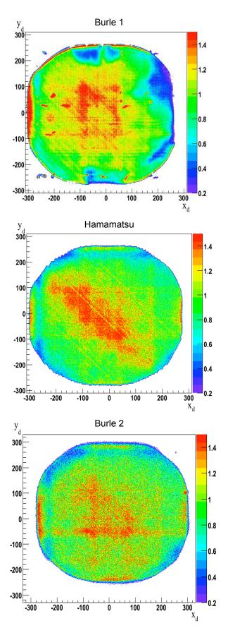
Figure A.10: Gain maps of the three MCPs used during this thesis. The number of atoms per pixel has been divided by the average number of counts per pixel in order to make a comparison among the three maps. The "Burle 1" gain map has been acquired in Amsterdam at 2350 V. The Hamamatsu gain map has been acquired at 2100 V and the "Burle 2" gain map has been acquired at 2350 V.
