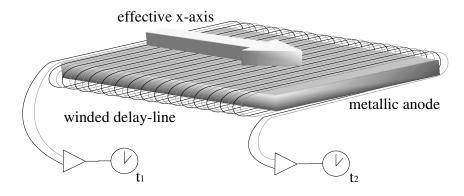
Figure A.4: In order to increase the number of pixels, the propagation speed of the electronic pulse on the delay-line is decreased by winding the line around a metallic plate. The measurement axis becomes the winding axis and the number of pixels along this axis is increased by the number of windings.
