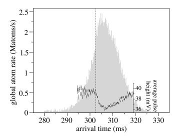
Figure A.9: Measurement of the saturation of the detector. This measurement has been performed on the detector referred as "Burle 1". We report the time-of-flight of a <sup>4</sup>He cloud at 1.6  $\mu$ K together with the variation of the averaged pulse height. We note a clear drop in the pulse height when the flux of detected atoms reaches 1.7  $\pm$  0.2 Matoms/s. This corresponds to a detected particle rate of  $82 \pm 10 \text{ katoms/cm}^2/\text{s}$ .
