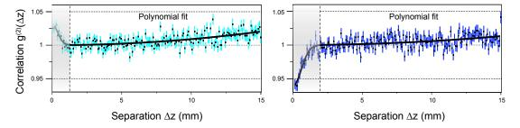
Figure 3.3: Normalised correlation function along the z axis for bosons (on the left) and fermions (on the right) at 0.5  $\mu$ K. In this figure the correlation function has been averaged over 10 couples  $(\Delta x, \Delta y)$  in order to increase the signal to noise ratio. The part of the graph in shadow is the bunching/antibunching and it is not fitted with the polynomial function. The error bars correspond to the square root of the number of entries in each bin.
