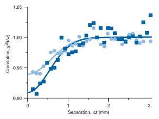
**Figure 3** | **Effect of demagnifying the source size.** We show normalized correlation functions along the z (vertical) axis for  ${}^{3}$ He\*, with (dark blue squares) and without (light blue circles) a diverging atomic lens in the x–y plane. The dip is deeper with the lens, because the increase of the correlation lengths in the x–y plane leads to less reduction of contrast when convolved with the resolution function in that plane.
