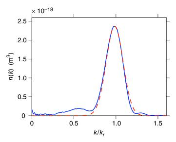
**Figure 4.** Angle averaged (radial) momentum distribution n(k) of the scattered atoms (solid line) and a simple Gaussian fit (dashed line) used to define the radial width  $\delta k = 0.10k_r$  of the halo around the peak momentum  $k_0 = 0.98k_r$  (see text).
