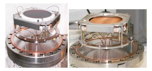
Figure A.5: On the left side: MCP detector with delay-line anode assembly. On the right side: the delay-lines are shown. The MCP has been removed from the mount.
