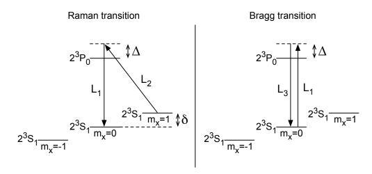
Figure 5.4: Level scheme for the transition used to drive Raman and Bragg transition.
