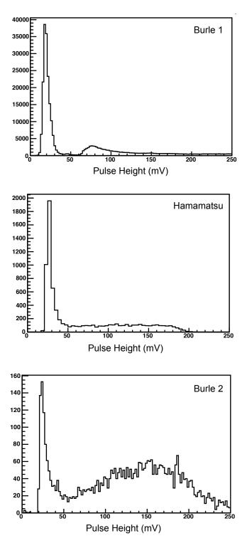
Figure A.8: Pulse height distribution for the three MCPs used during this thesis. The pulse height has been measured in the high gain region (at  $2350~\rm V$  for "Burle 1",  $2100~\rm V$  for "Hamamtsu",  $2400~\rm V$  for "Burle 2"). The two Burle MCPs clearly show a double structure, while this is less evident for the Hamamatsu. The vertical scale is not the same for the three graphs.
