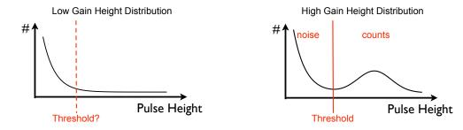
Figure A.7: Pulse height distribution for a chevron MCP working in the low gain region and in the high gain region. At low gain the amplitude distribution is exponential and cannot be distinguished from the background noise. When the gain saturates a double structure appears in the amplitude distribution and it is possible to discriminate between real counts and noise.
