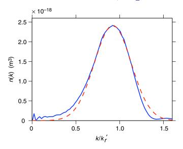
**Figure 9.** Same as in figure 4 except for  $\sqrt{2}$  times smaller collision velocity  $v_r'$  ( $k_r' = 4.1 \times 10^6 \,\mathrm{m}^{-1}$ ). The width and the peak of the fitted Gaussian are  $\delta k = 0.21 k_r' = 8.6 \times 10^5 \,\mathrm{m}^{-1}$  and  $k_0 = 0.92 k_r'$ .
