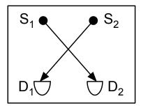
Figure 1.4: Two particles emitted by the two source points  $S_1$  and  $S_2$  are detected at  $D_1$  and  $D_2$ . The two particles can follow two paths that are sketched in this figure. The interference between the two paths leads to the Hanbury Brown Twiss effect.
