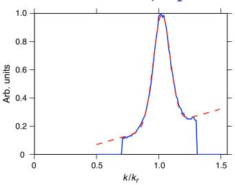
**Figure 2.** Cross-section of the scattering halo. A sloped background is present due to thermal atoms in the trap. This background has been fitted to a straight line and subtracted in order to estimate the rms width,  $\delta k \simeq 0.067 k_r$ .
