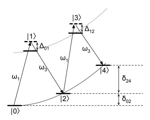
Figure 5.7: Energy diagram of the states that can be excited in a two-photon and a four-photon Bragg process.
