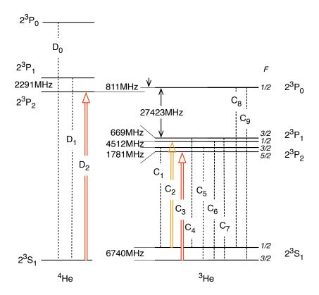
Figure 2.4: On the left, scheme of the optical transitions used to laser cool  ${}^{4}\text{He}$ . On the right, scheme of the optical transition used to cool  ${}^{3}\text{He}$ . Since the isotopic shift is about 30 GHz, a double laser system is needed. The transitions  $C_{3}$  and  $D_{2}$  are used to cool  ${}^{3}\text{He}$  and  ${}^{4}\text{He}$  respectively. An additional laser resonant with the transition  $C_{2}$  of the  ${}^{3}\text{He}$  is needed as a repumper.
