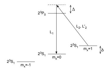
Figure 4.7: Scheme of the Raman transition used to create the two colliding condensates. Since the final state of the Raman transition is insensitive to the magnetic field, the atoms that undergo the Raman transition fall on the micro-channel plate under the effect of gravity and are detected without the need of switching off the magnetic trap.
