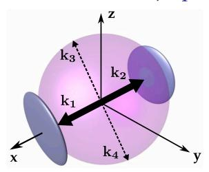
**Figure 1.** Schematic momentum space diagram of the atomic four-wave mixing interaction. Optical Raman pulses generate untrapped condensates with momenta  $\mathbf{k}_1$  and  $\mathbf{k}_2 = -\mathbf{k}_1$  parallel to the *x*-axis (dark disks). These undergo a four-wave mixing interaction to produce correlated atomic pairs on a spherical shell of radius  $k_1$ .
