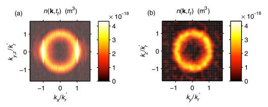
**Figure 8.** Same as in figure 3, except for  $\sqrt{2}$  times smaller collision velocity,  $v_r' =$  $6.46 \,\mathrm{cm}\,\mathrm{s}^{-1}$   $(k_r' = 4.09 \times 10^6\,\mathrm{m}^{-1})$ . The axes for the momentum components  $k_i$ (i = x, y and z) are in units of smaller recoil momentum than in figure 3, and therefore the absolute radius of the s-wave scattering sphere is smaller in the present example.
