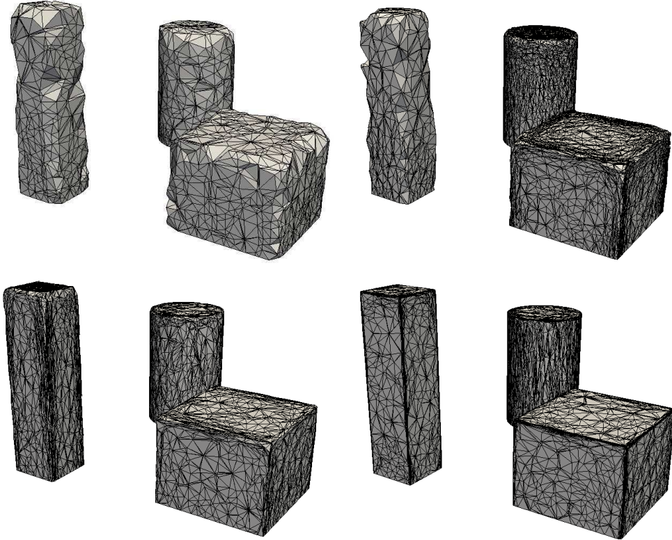
Figure 1. Mesh adaptation in the vicinity of the interface: from the initial mesh to the final mesh.
