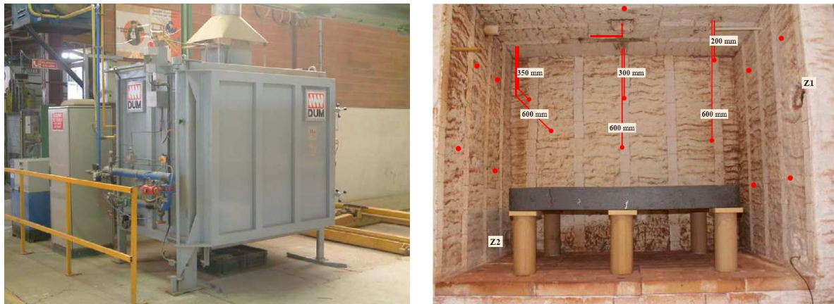
Figure 1. 1 \text{ m}^3 furnace (left) and the support grid (right)
