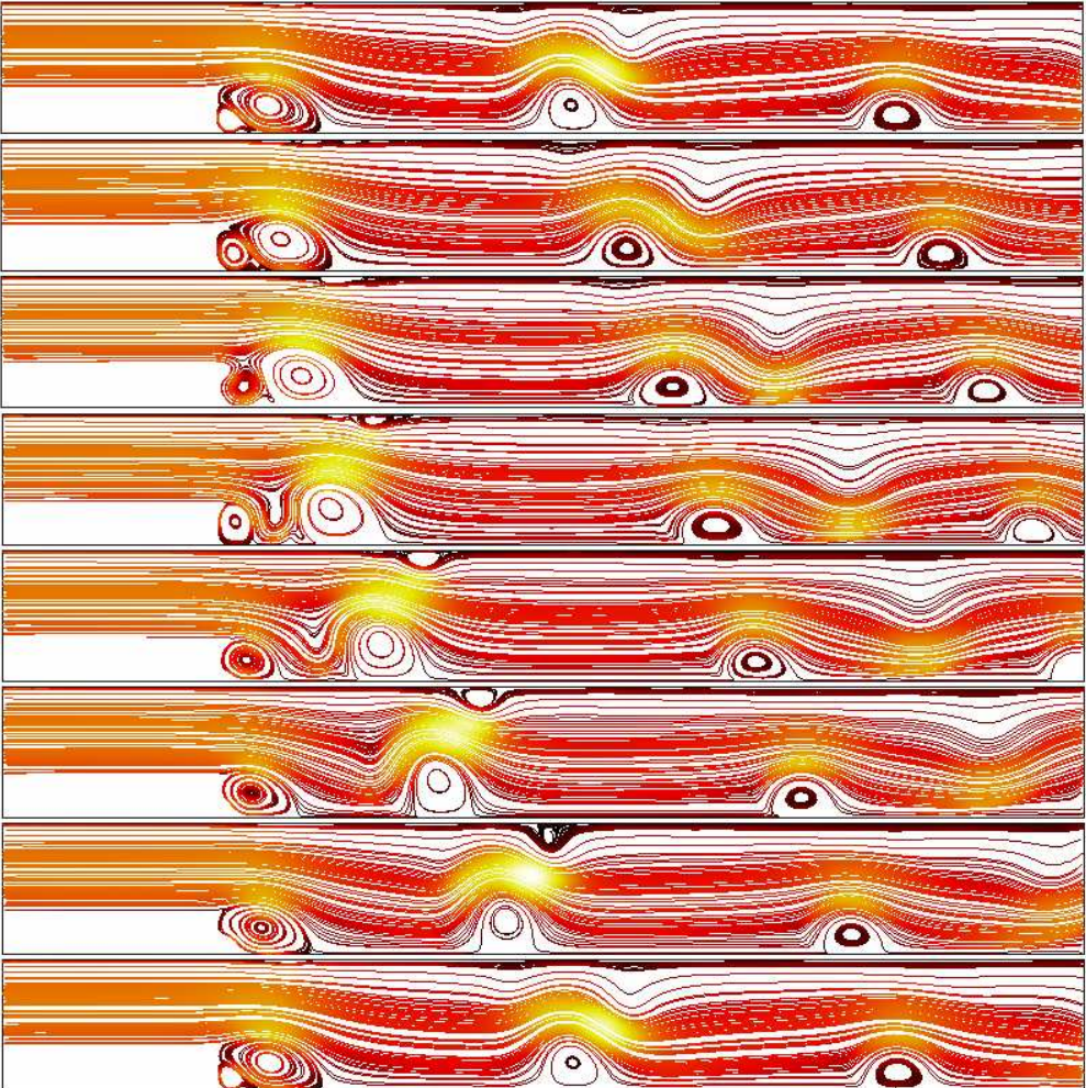
Figure 29. Periodic evolution of streamlines from t=3.04s to t=3.11s
