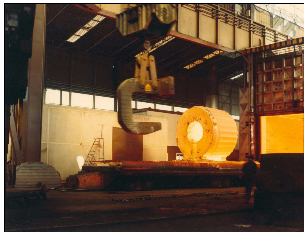
Large hollow metal ingot outside the furnace
