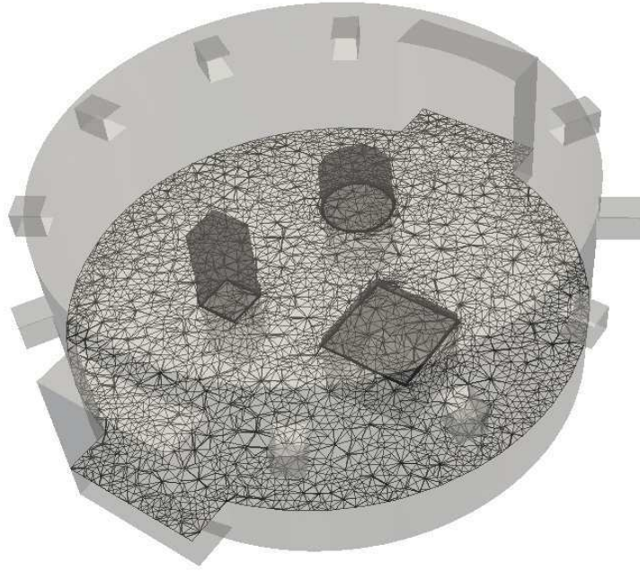
Figure 2. Computational domain after anisotropic adaptation
