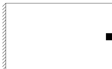
FIG. 3.2 – Boundary conditions for a 2-d cantilever (the black zone is heavier and not subject to optimization).
