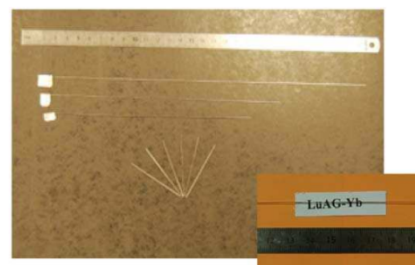
Fig. 5. Undoped and Yb-doped LuAG fibers grown under stationary state.
