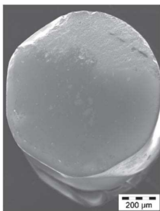
Fig. 7. Fiber cross-section showing the LuAG facets.
