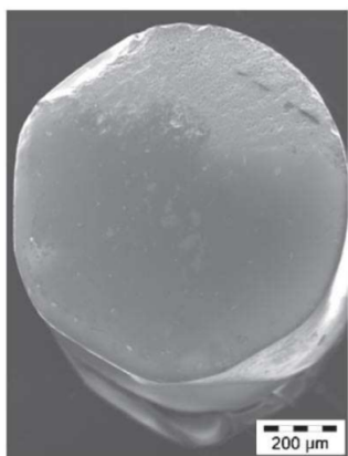
Fig. 7. Fiber cross-section showing the LuAG facets.
