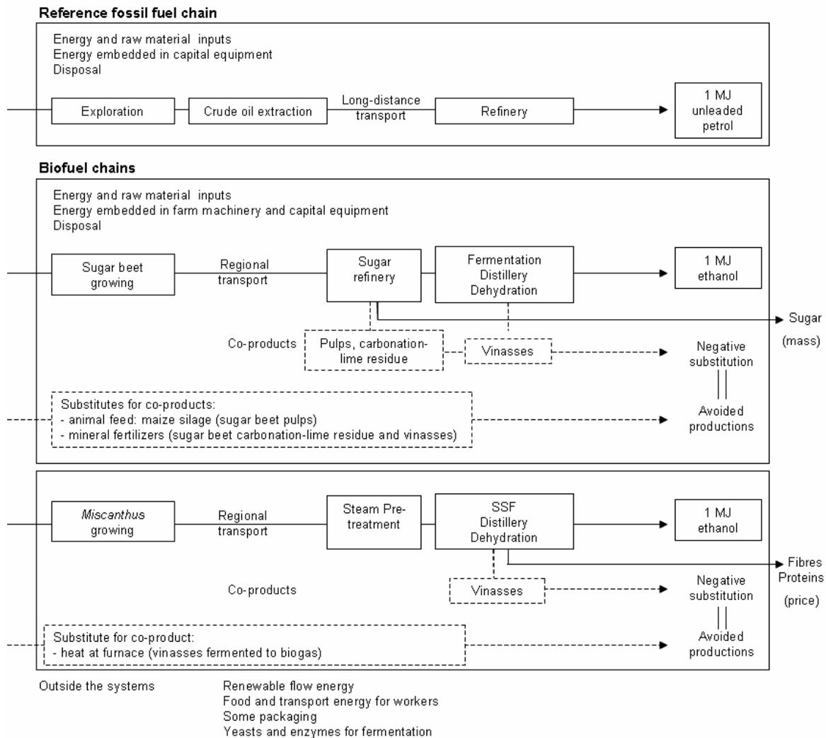
Figure 1: Well-to-Tank system boundaries of studied fuel chains.
