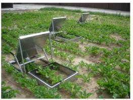
Measurement of N<sub>2</sub>O and CO<sub>2</sub> fluxes with automatic chambers in a sugar beet plot, Estrées-Mons, June 2008 bessou©INRA
