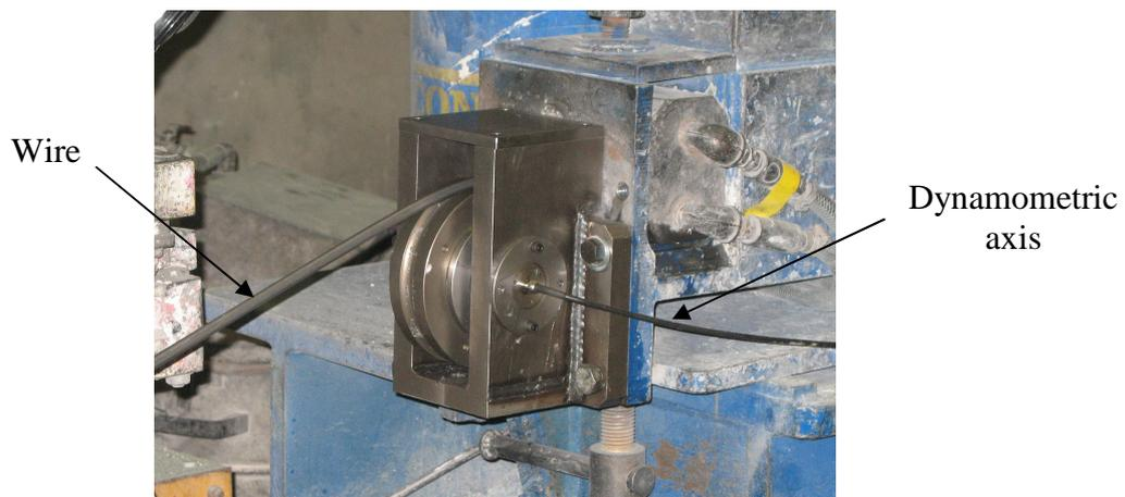
**Figure 47: Experimental device for the drawing force measurement [4]**
