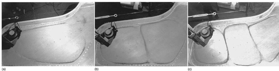
FIG. 1.8 – Chladni patterns of the three lowest modes of the soundboard of a concert grand installed in its wooden rim, without bridges, string frame and strings, after Conklin [35]. (a) (1,1)-mode, f \approx 49 Hz. (b) (2,1)-mode, f \approx 66.7 Hz. (c) (3,1)-mode, f \approx 89.4 Hz.
