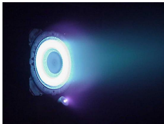
Figure 1: Photo of the PPS®1350-G thruster in operation
