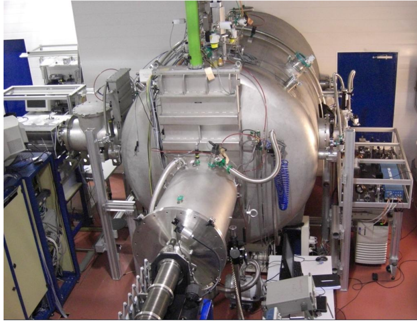
Figure 2.5: Vacuum vessel at PIVOINE ground test facility with optical bench PRAXIS-I
