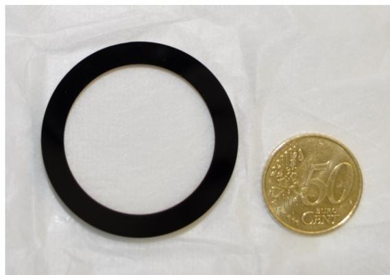
**Figure 5.14.:** 2 at.% doped  $\text{Yb}^{3+}$ :YAG (35 mm diameter, transparent) ceramic with 5 mm thick  $\text{Cr}^{4+}$ :YAG periphery (black). The thickness is 7 mm. A 50 Euro-Cent coin is given for size comparison.
