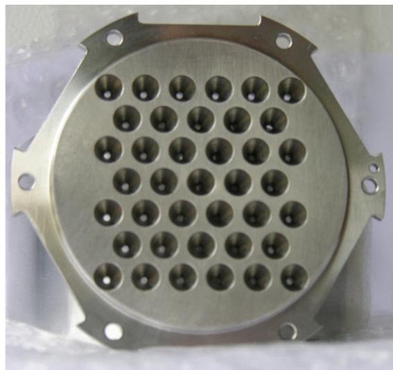
Figure 2.31.: Manufactured jet-plate with 39 holes, shown from the water inlet side.
