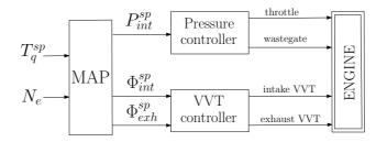
Figure 1.8: Classic control strategy to manage the cylinder filling.  $T_q^{sp}$  and  $N_e$  refer to the driver torque demand and the engine speed, respectively. Look-up tables determine set points for the intake manifold pressure and VVT actuator positions,  $P_{int}^{sp}$ ,  $\Phi_{int}^{sp}$ , and  $\Phi_{exh}^{sp}$ .
