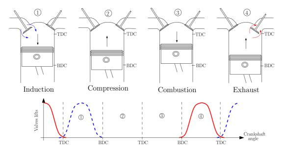
Figure 1.1: Four-stroke cycle of internal combustion engines. Four successive phases (induction, compression, combustion, exhaust) take place. They are separated by TDC and BDC.
