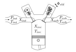
Figure 4.2: CI engine in-cylinder variables as a function of cylinder bounding conditions.
