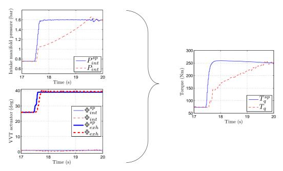
Figure 1.9: Experimental results obtained on vehicle during a large torque tip-in. Classical controller do not exploit the VVT actuators at their best. These are fed with static set points values. The obtained torque response is relatively slow, and can be improved.
