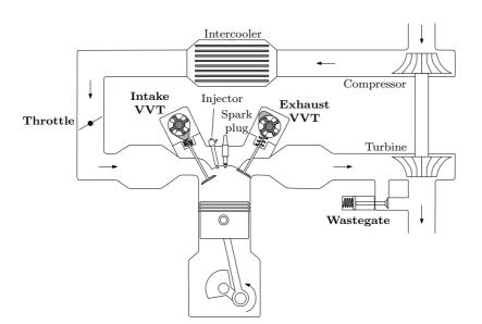
Figure 1.4: Schematic illustration of a turbocharged, VVT-equipped SI engine.
