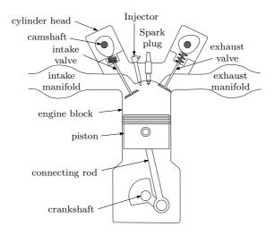
Figure 1.2: Engine components about the combustion chamber.
