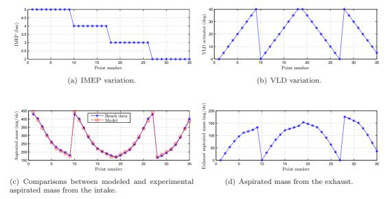
Figure 2.14: Comparisons between modeled and experimental aspirated mass at constant engine speed (1500 rpm).
