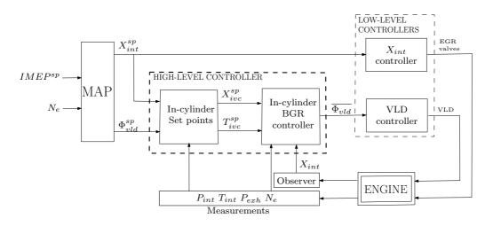
Figure 4.9: Control scheme. The in-cylinder set points  $X_{ivc}^{sp}$  and  $T_{ivc}^{sp}$  are given in Section 4.2.1. The high-level controller coordinates the low-level controllers using the control law presented in Section 4.2.2 to determine VLD actuator trajectory  $\overline{\Phi_{vld}}$ .
