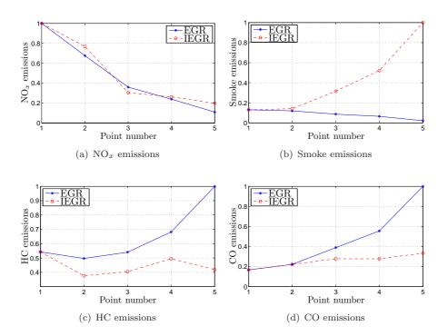
Figure 1.11: Engine emissions for increasing external or internal EGR at constant IMEP (2 bar), constant engine speed (2000 rpm) and constant intake manifold pressure (1 bar). IEGR allows a reduction of the HC-CO emissions to the detriment of the smoke emissions. Experimental data obtained at test bench on a 4-cylinder CI engine equipped with VLD actuator and LP EGR capability.
