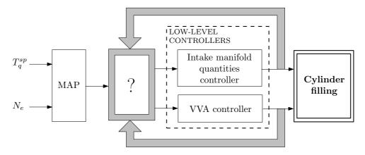
Figure 1.14: Sketch of the coordination-based control strategy.  $T_q^{sp}$  and  $N_e$  refer to the driver torque demand and the engine speed, respectively. A high-level controller block takes place upstream the low-level controllers.
