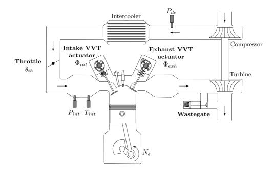
Figure 3.1: Schematic illustration of a turbocharged, VVT-equipped SI engine. The intake manifold pressure and temperature  $P_{int}$  and  $T_{int}$  and the downstream compressor pressure  $P_{dc}$  are measured by sensors.  $\theta_{th}$  is the angular position of the throttle,  $\Phi_{int}$  and  $\Phi_{exh}$  are the positions of the VVT actuators.
