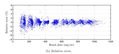
Figure 2.9: Comparisons between modeled and experimental aspirated air mass over more than 3000 points ( $P_{int}$  from 0.3 to 2 bar,  $N_e$  from 750 to 3000 rpm and all intake and exhaust VVT actuators positions).
