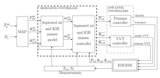
Figure 3.5: Control scheme. The high-level controller coordinates the low-level controllers using control laws (3.12) and (3.16).
