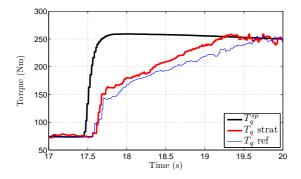
Figure 3.13: On-board experimental results from a vehicle equipped with a four-cylinder turbocharged VVT SI engine. Large torque tip-in. Comparison between proposed strategy ("strat") and classical strategy ("ref") on the torque production.
