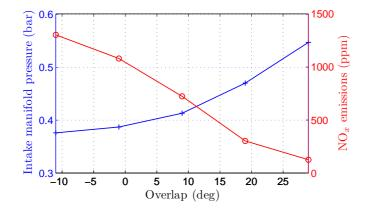
Figure 1.6: Beneficial effects of valve overlap variations on the intake manifold pressure and the  $NO_x$  emissions at constant engine speed (1500 rpm) and constant torque (30 Nm). Experimental data obtained on a 4-cylinder SI engine test bench equipped with VVT actuators.
