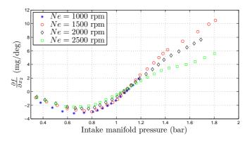
Figure 3.9: Sensitivity of aspirated air mass with respect to the VVT actuator.
