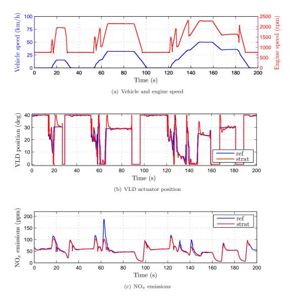
Figure 4.16: Test-bench results for a four-cylinder CI engine for an ECE driving cycle with and without the proposed control strategy.  $NO_x$  emissions are reduced during transients.
