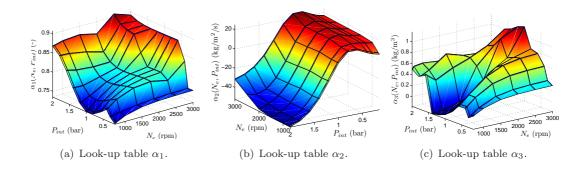
Figure 2.7: Look-up tables for the cylinder filling model parameters.
