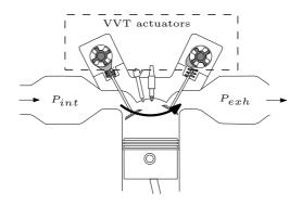
Figure 1.7: Under turbocharging conditions, a part of the fresh air can be *scavenged* towards the exhaust pipe.
