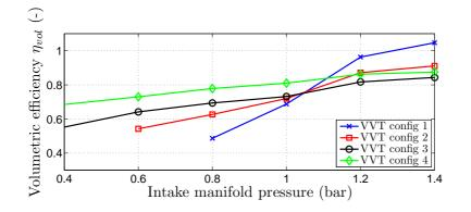
Figure 2.1: Volumetric efficiency function of the intake manifold pressure, at constant engine speed (1500 rpm), and different positions of the VVT actuators.
