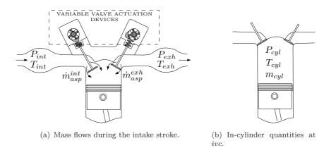
Figure 2.2: Notation used in the cylinder filling model. In this section, all the intake and exhaust manifolds thermodynamics quantities for the general model design are used. It will be seen later that some exhaust quantities are in fact not measured in the application.
