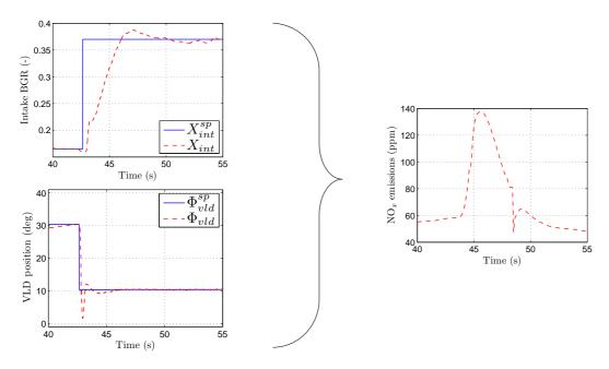
Figure 1.13: Experimental IMEP transient (3-5 bar) at test bench on a 4-cylinder CI engine equipped with VLD actuator and LP EGR capability. The difference in response times between the intake manifold BGR and the VLD actuator leads to  $NO_x$  emission peak during transient.
