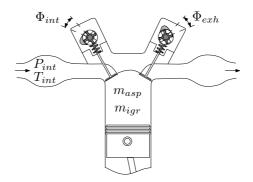
Figure 3.2: SI engine control variables as a function of cylinder bounding conditions.  $m_{asp}$  and  $m_{igr}$  are the control targets.  $P_{int}$ ,  $\Phi_{int}$  and  $\Phi_{exh}$  are the "actuators".
