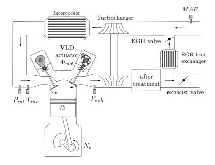
Figure 4.1: Schematic illustration of a turbocharged VLD-equipped engine. The intake manifold pressure and temperature  $P_{int}$  and  $T_{int}$ , the exhaust manifold pressure  $P_{exh}$  and the mass air flow at the intake MAF are measured by sensors.  $\Phi_{vld}$  is the position of the VLD actuator.
