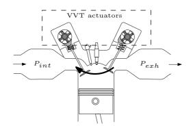
Figure 1.5: Under atmospheric conditions, *back-flow* of exhaust burned gases may occur during the intake stroke.
