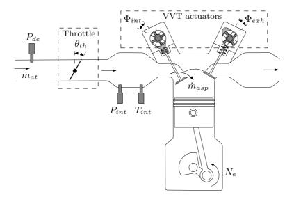
Figure A.1:  $\dot{m}_{at}$  and  $\dot{m}_{asp}$  are the non-measured inlet and aspirated air mass flows respectively. Downstream compressor pressure,  $P_{dc}$ , intake manifold pressure and temperature,  $P_{int}$  and  $T_{int}$ , and engine speed,  $N_e$ , are measured by sensors.  $\theta_{th}$ ,  $\Phi_{int}$  and  $\Phi_{exh}$  are the actuators angle positions.
