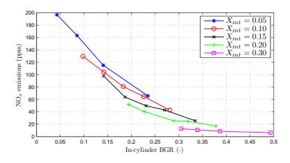
Figure 2.16: NO<sub>x</sub> emissions function of the in-cylinder BGR, for different intake manifold BGR levels,  $X_{int}$ , at constant engine speed (2000 rpm).
