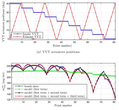
(b) In-cylinder aspirated mass from intake.
