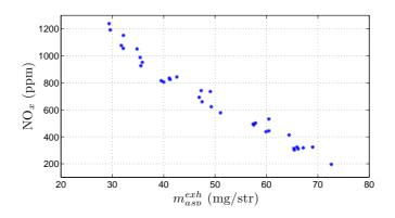
Figure 2.10: Experimental  $NO_x$  emissions function of estimated aspirated mass from the exhaust at constant torque. Emissions decrease with the increase of the in-cylinder burned gas fraction [24].
