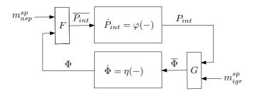
Figure 3.6: The control strategy implies an interconnection of the intake manifold pressure and the VVT subsystems. The mappings F and G are given by the model inversions (3.8) and (3.9)–(3.10).
