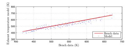
Figure 4.6: Comparisons between modeled and experimental exhaust temperature over the whole engine operating range. Experimental data obtained at test bench on a 4-cylinder CI engine equipped with VLD actuator and LP EGR capability.
