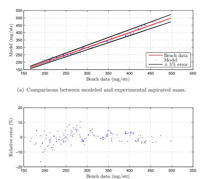
Figure 2.15: Comparisons between modeled and experimental aspirated mass over about 150 points (IMEP from 2 to 6 bar,  $N_e$  from 800 to 2500 rpm and all VLD actuator positions).
