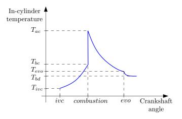
Figure 4.5: Detail of the exhaust temperature model.
