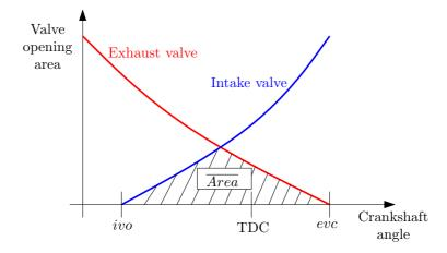
Figure 2.3: Intake and exhaust valves opening areas as a function of the crankshaft angle.  $\overline{Area}$  is defined as the average opening area under both valves during the valve overlap.
