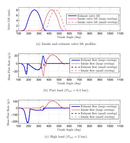
Figure 2.4: Amesim<sup>TM</sup> simulator results. Instantaneous flows through intake and exhaust valves for two different valve overlap at part and high load.
