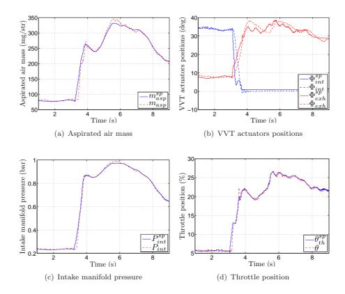
Figure A.6: Experimental results for a four-cylinder SI engine on vehicle during take off.
