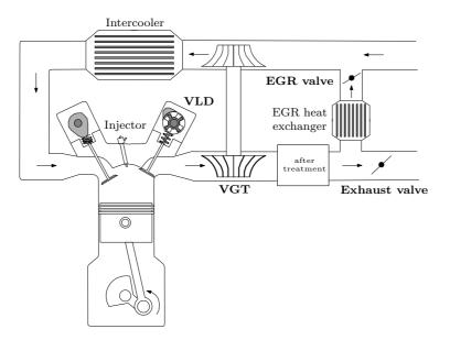
Figure 1.10: Schematic illustration of turbocharged, VLD-equipped CI engine.
