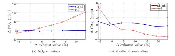
Figure 4.12: Variation of  $NO_x$  emissions and middle of combustion (CA<sub>50</sub>) relative to an exhaust valve position variation. Point (0,0) refers to the reference engine operating point.
