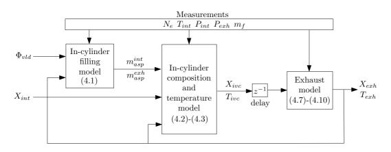
Figure 4.7: Schematic view of the in-cylinder BGR and temperature model.
