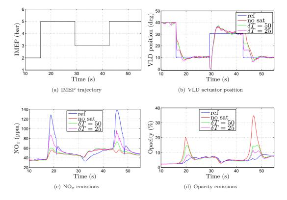
Figure 4.15: Test-bench results for a four-cylinder CI engine for step torque demand at constant speed of 1000 rpm with and without the proposed control strategy. Taking into account an in-cylinder temperature limitation in the control strategy permits to decrease the losses in smoke emissions while keeping the gains in  $NO_x$  emissions.
