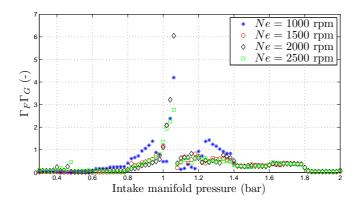
Figure 3.8: Conditions for small-gain theorem.
