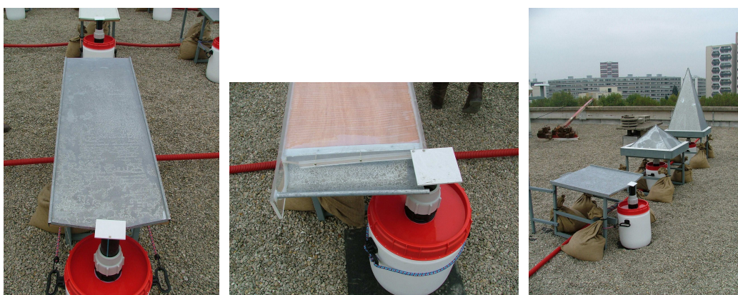
Figure 1: pictures of our experimental test bed (left to right: natural zinc panel, gutter, and pyramids)
