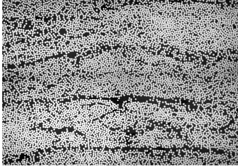
Figure 3.1: Two-dimensional cut of a composite material used in the aeronautics industry, extracted from [83] and reproduced with permission of the author. It is clear that this material is not periodic, yet there is some kind of an underlying periodic arrangement of the fibers.
