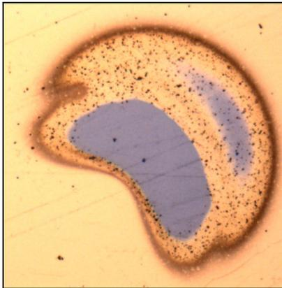
Figure 6: optical image of the degraded gold substrate.
