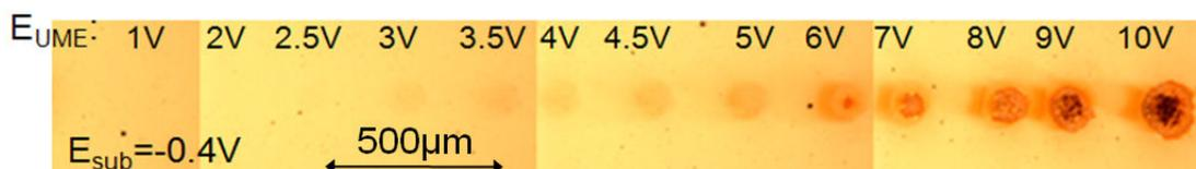
Figure 8: Localization of the grafting from the diazonium salt alone. Optical image of grafted dots for different potentials imposed to UME;  $E_{sub} = -0.4V$ /Ag wire,  $DNB: 2 \cdot 10^{-3} \text{ mol.dm}^{-3}$ ,  $H_2SO_4: 0.25 \text{ mol.dm}^{-3}$ ,  $100 \mu\text{m-Pt}$ ,  $d = 20 \mu\text{m}$ ,  $t = 5\text{s}$ .
