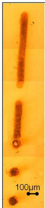
Figure 32: Optical microscopy image of the localized electrografted PNP initiated by the electroreduction of NBD ( $2 \cdot 10^{-3} \text{ mol.dm}^{-3}$ ),  $\text{H}_2\text{SO}_4$   $0.25 \text{ mol.dm}^{-3}$ ;  $50\mu\text{m-Pt UME}$ ,  $d = 20 \mu\text{m}$ ,  $I = -2\text{mA}$ , lines obtained at a scan rate of  $50 \mu\text{m s}^{-1}$ , dots:  $t = 5 \text{ s}$ .
