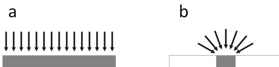
Scheme 1: Schematic representation of planar (a) and hemispherical (b) diffusion.
