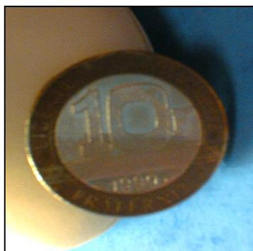
*Figure 1: Electrografted film of polymethacrylonitrile on half part of a French coin.*
