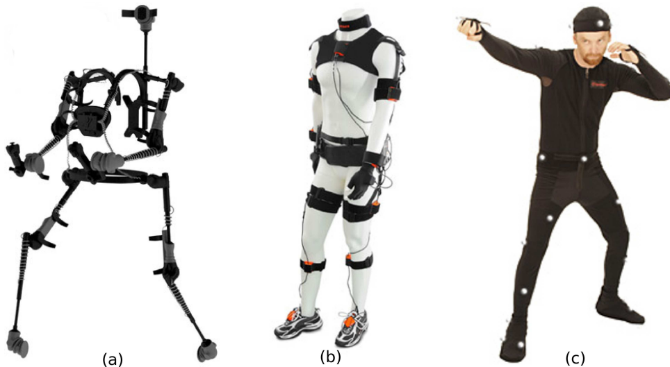
FIGURE 2.1: Examples of systems using markers. (a) exoskeleton of Gypsy TM mechanical system. (b) markers of Xsens TM inertial system. (c) markers of OptiTrack TM passive optical system.
