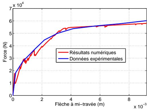
FIG. 4.40 – Courbe force/déplacement  $T_c = 1,25\%$ .
