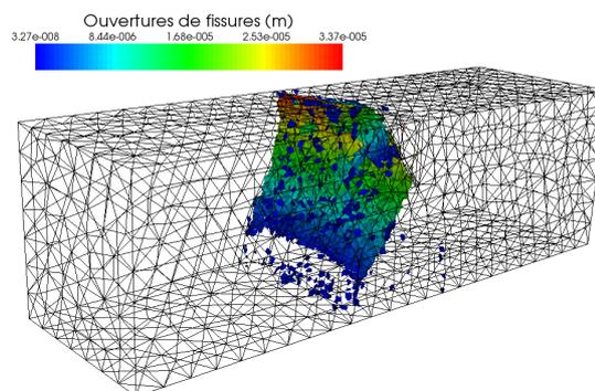
FIG. 6.2 – Surface de fissuration.
