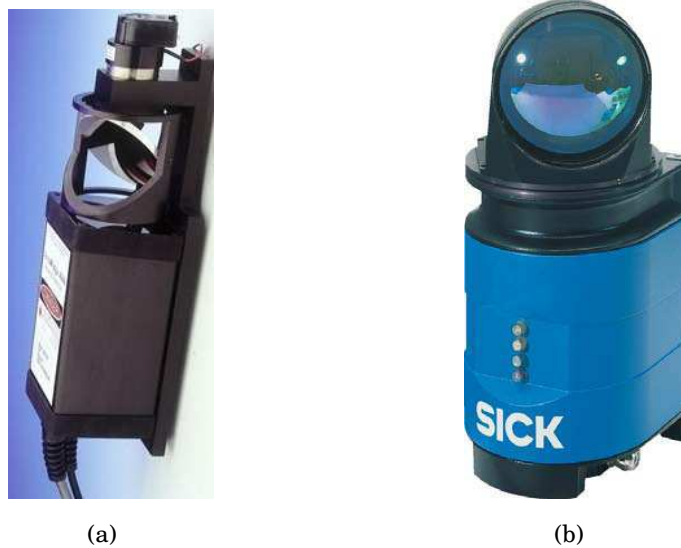
Figure 2.13: Laser range finders mounted on Anis and Hannibal respectively. 2.13(a) AccuRange 4000. 2.13(b) Sick LD-LRS1000.
