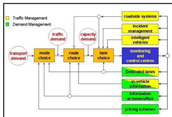
Figure 1: The ITS control Scheme
