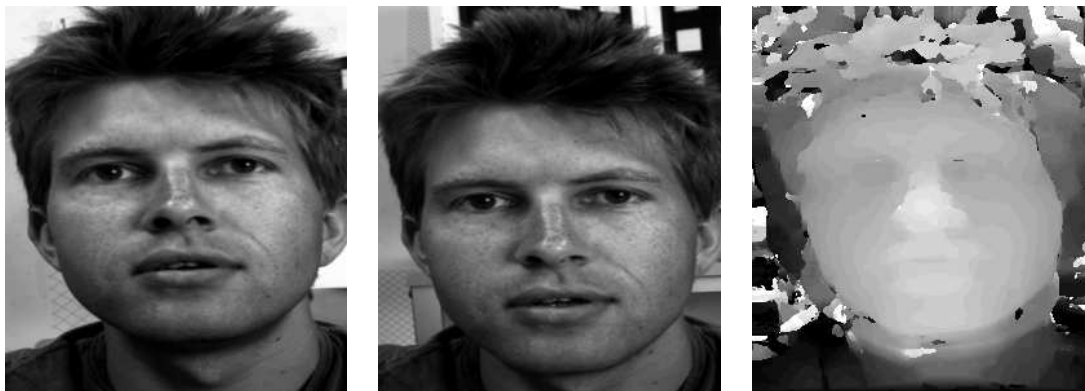
Figure 5.8: Two images and the stereo reconstruction using a maximum spanning forest algorithm. This preliminary result is obtained using a different graph than the one described in Fig. 5.7, and is composed of different levels, each level corresponding to a different disparity.
