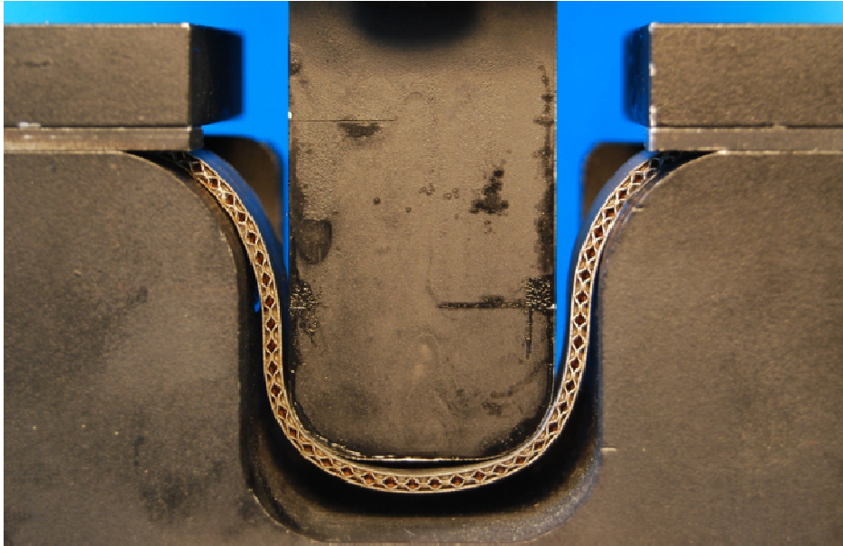
Fig. 3 : Experiment of bi-directional draw bending of a sandwich prototype.
