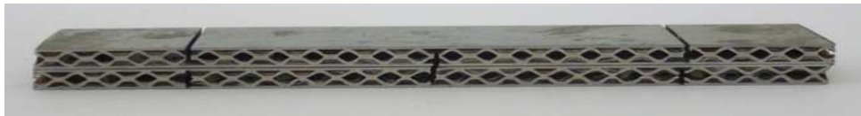
Fig. 2.6 : Shear-lap test experiment specimen.
